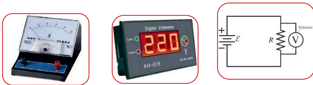
Figure 6.29: Voltage measuring devices
