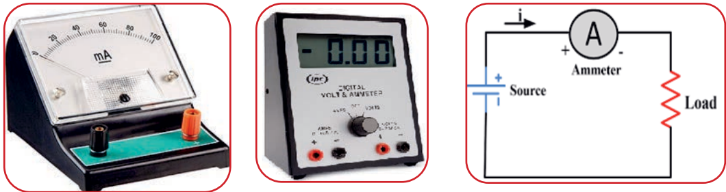
Figure 6.27: Ammeters and How to connect them.
