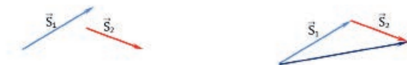
Figure 2.6 Triangle law of addition of vectors: \vec{s}_1 and \vec{s}_2 are placed head to tail.
