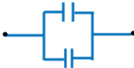
Figure 6.56: The equivalent capacitance of the network in Figure 6.55
