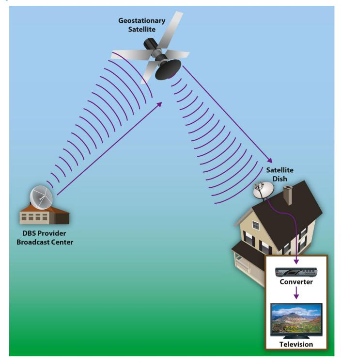
Figure 9.17 Subscribers of DBS receive signals from geostationary satellites that are broadcast in digital format at microwave frequency and intercepted by a satellite dish. A converter next to the television produces output that can be viewed on the television receiver.
