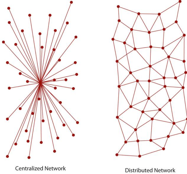
Figure 11.2 Centralized versus distributed communication networks
