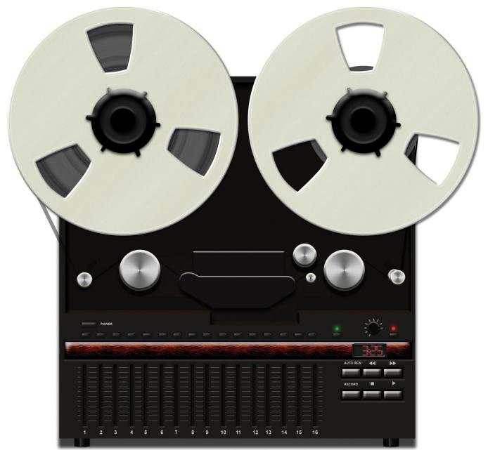
Figure 6.5 Reel-to-reel tape recorders and magnetic tape not only helped artists experiment with overdubbing, but they also were a compact method for reproducing and preserving audio.
