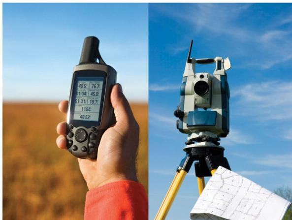
In the case of GPS, handheld units access positional data from satellites and log the information for subsequent retrieval. A network of twenty-four navigation satellites is situated around the globe and
