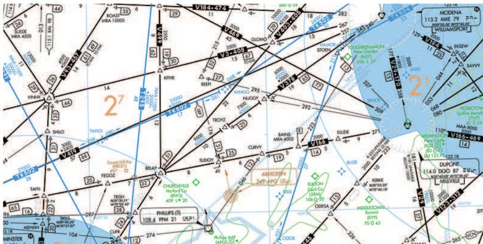
Figure 10.8: Air navigation chart: VOR stations as black hexagons (PPM, DQO, MXE), NDB station as brown spot (APG), VORNAV intersection fixes as black triangles (FEGOZ, BELAY, SAVVY), RNAV fixes as blue stars (SISSI, BUZIE, WINGO), VORNAV airways in black (V166, V499), RNAV airways in blue (TK502, T295), and other data. Author: User:Orion 8 / [Wikimedia Commons](#) / Public Domain.
