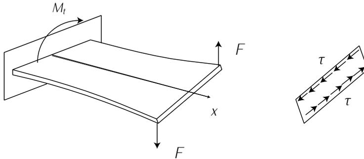
Figure 4.5: Shear stress due to torsion. Adapted from FRANCHINI *et al.* [2].
