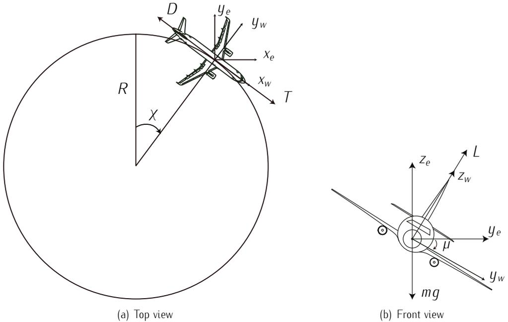
Figure 7.3: Aircraft forces in a horizontal loop.
