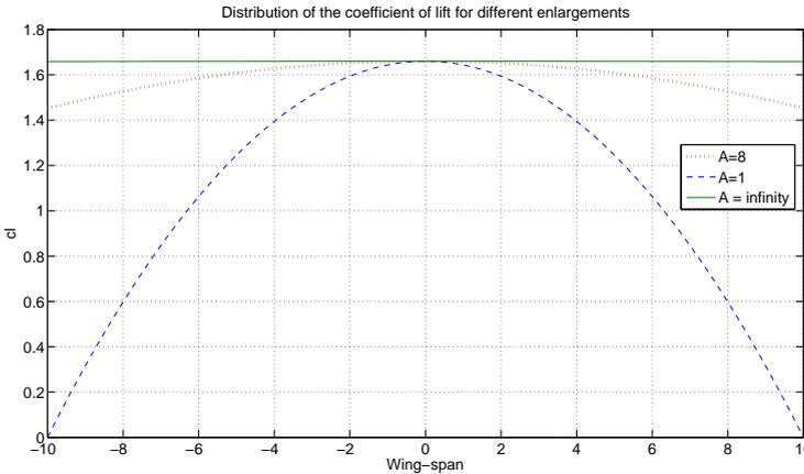
Figure 3.33: Coefficient of lift along the wingspan (Problem 3.4).
