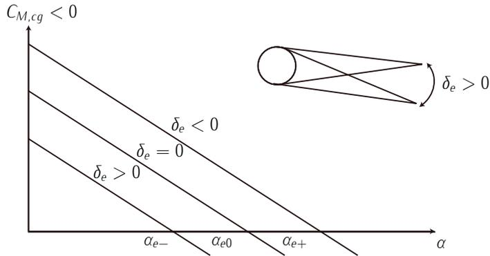
Figure 7.15: Effects of elevator on moments coefficient. Adapted from FRANCHINI and GARCÍA [3].
