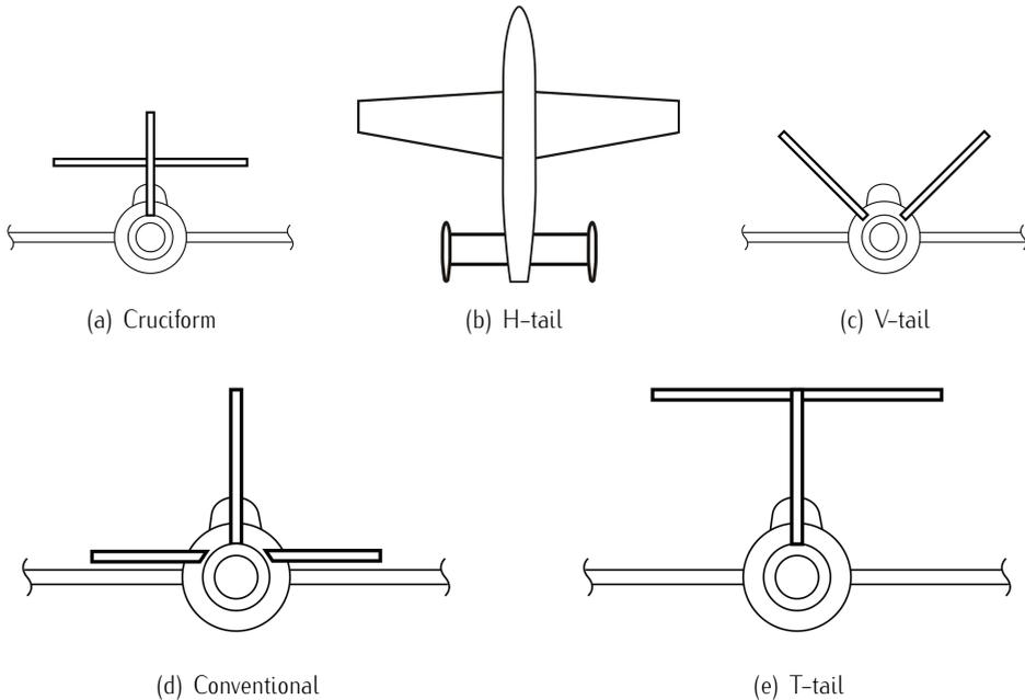
Figure 2.13: Aircraft's empennage types. © Guy Inchbald / [Wikimedia Commons](https://commons.wikimedia.org/wiki/File:Empennage_types.png) / CC-BY-SA-3.0.
