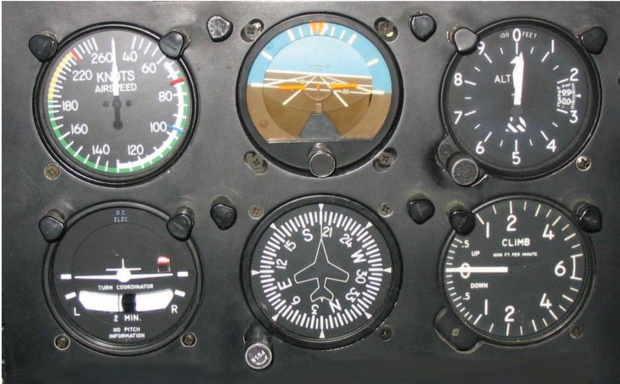
Figure 5.9: Six basic instruments in a light twin-engine airplane arranged in a *basic-T*. From top left: airspeed indicator, attitude indicator, altimeter, turn coordinator, heading indicator, and vertical speed indicator. © User:Meggarr / [Wikimedia Commons](#) / [CC-BY-SA-3.0](#).
