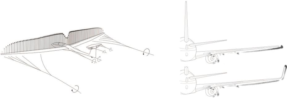
(a) A realistic lift distribution over the wing of an aircraft. The continuously changing lift distribution causes the shedding of a vortex sheet whose strength varies span-wise.. © Olivier Cleynen / [Wikimedia Commons](#) / [CC-BY-SA-3.0](#).
