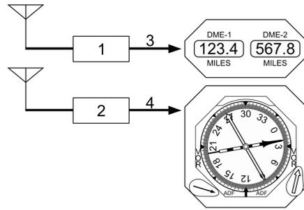
(b) DME on-board receiver, together with ADF unit (reading the VOR information). © User:Tosaka / [Wikimedia Commons](#) / [CC-BY-SA-3.0](#).
