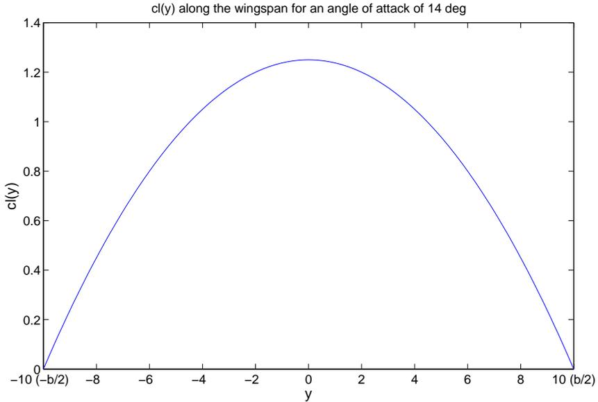
Figure 3.29: Coefficient of lift along the wingspan (Problem 3.1).
