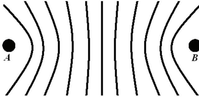
(a) LORAN diagram: the difference between the time of reception of synchronized signals from radio stations A and B is constant along each hyperbolic curve. Author: User: Massimiliano Lincetto / [Wikimedia Commons](#) / Public Domain.
