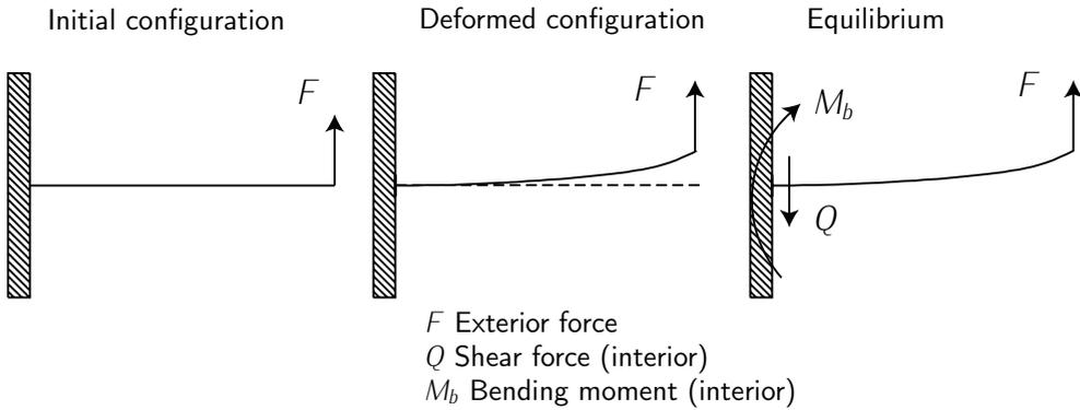
Figure 4.2: Bending. Adapted from FRANCHINI *et al.* [2].
