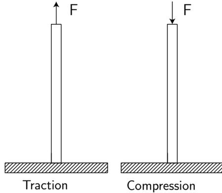
Figure 4.1: Normal stress. Adapted from FRANCHINI *et al.* [2].
