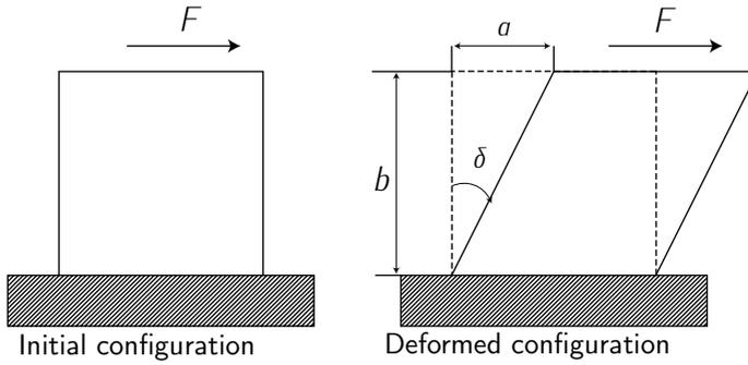
Figure 4.8: Tangential deformation. Adapted from FRANCHINI *et al.* [2].
