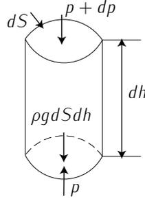
Figure 2.16: Differential cylinder of air. Adapted from FRANCHINI *et al.* [3].
