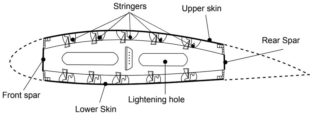
Figure 4.14: Structural wing torsion box. Adapted from © User Kadellar / [Wikimedia Commons](https://commons.wikimedia.org/wiki/File:Wing_torsion_box.png) // [CC-BY-SA-3.0](https://creativecommons.org/licenses/by-sa/3.0/).
