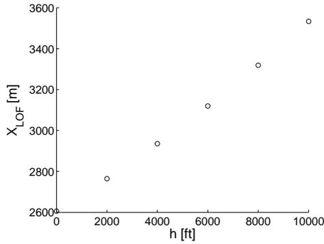
Figure 9.24:  $X_{LOF}$  for different altitudes at calm conditions.
