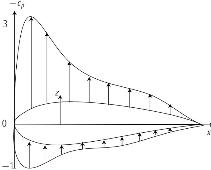
Figure 3.16: Distribution of Coefficient of Pressures. Adapted from FRANCHINI *et al.* [4].
