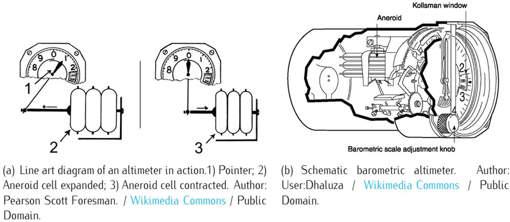
Figure 5.1: Barometric altimeter.
