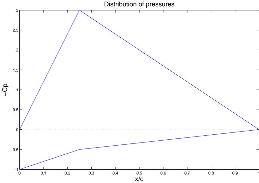
Figure 3.28: Distribution of the coefficient of pressures (Problem 3.1).
