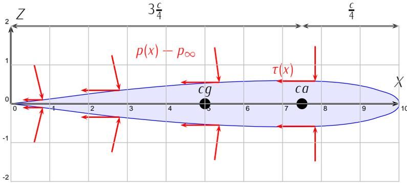
Figure 3.12: Pressure and friction stress over an airfoil.
