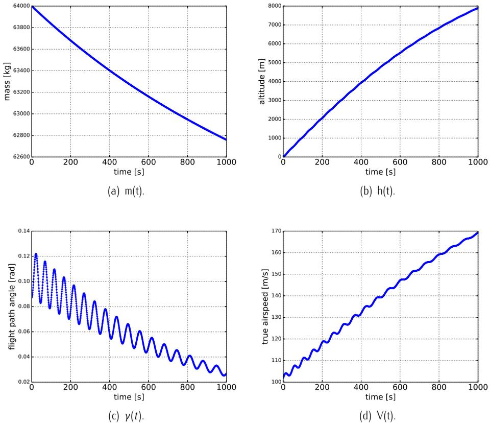
Figure B.4: Aircraft climb motion solution.
