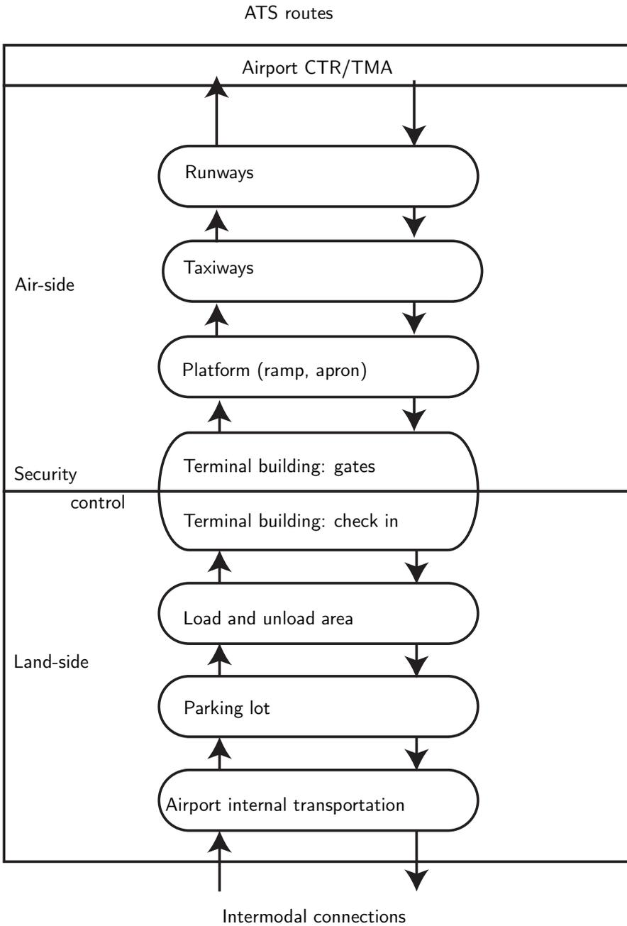
Figure 9.2: Schematic configuration of an airport. Adapted from FRANCHINI *et al.* [2].
