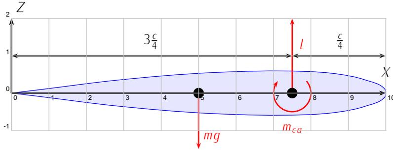
Figure 3.13: Aerodynamic forces and torques over an airfoil.
