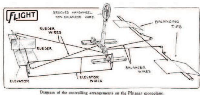
(a) Diagram showing the linkage between the control column and wheel and the various control surfaces of the Pfliizer Flyer (conventional control system). © User:Flight Magazine. / [Wikimedia Commons](#) / CC 0 1.0.
