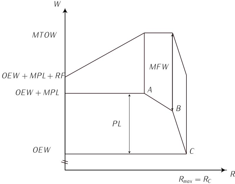
Figure 7.9: Payload-range diagram.
