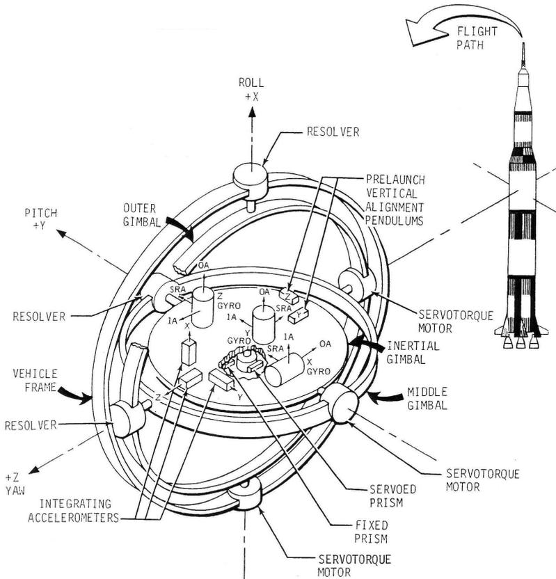
Figure 5.5: Diagram of ST-124 gimbals with accelerometers and gyroscopes (conforming the basic elements of a Inertial Measurement Unit). Author NASA/MSFC / Wikimedia Commons / Public Domain.
