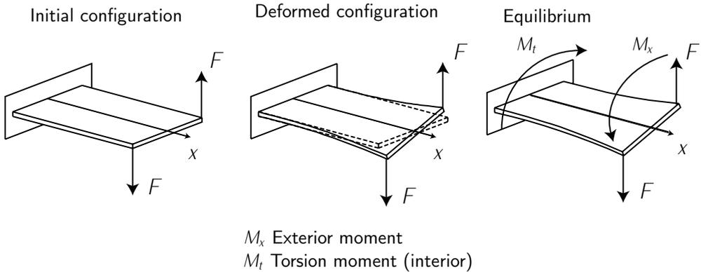
Figure 4.3: Torsion. Adapted from FRANCHINI *et al.* [2].
