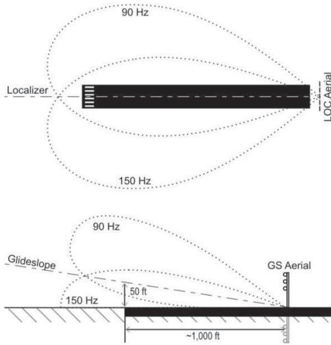
Figure 9.15: ILS: The emission patterns of the localizer and glide slope signals. Note that the glide slope beams are partly formed by the reflection of the glide slope aerial in the ground plane. © User:treemill / [Wikimedia Commons](#) / [CC-BY-SA-3.0](#).
