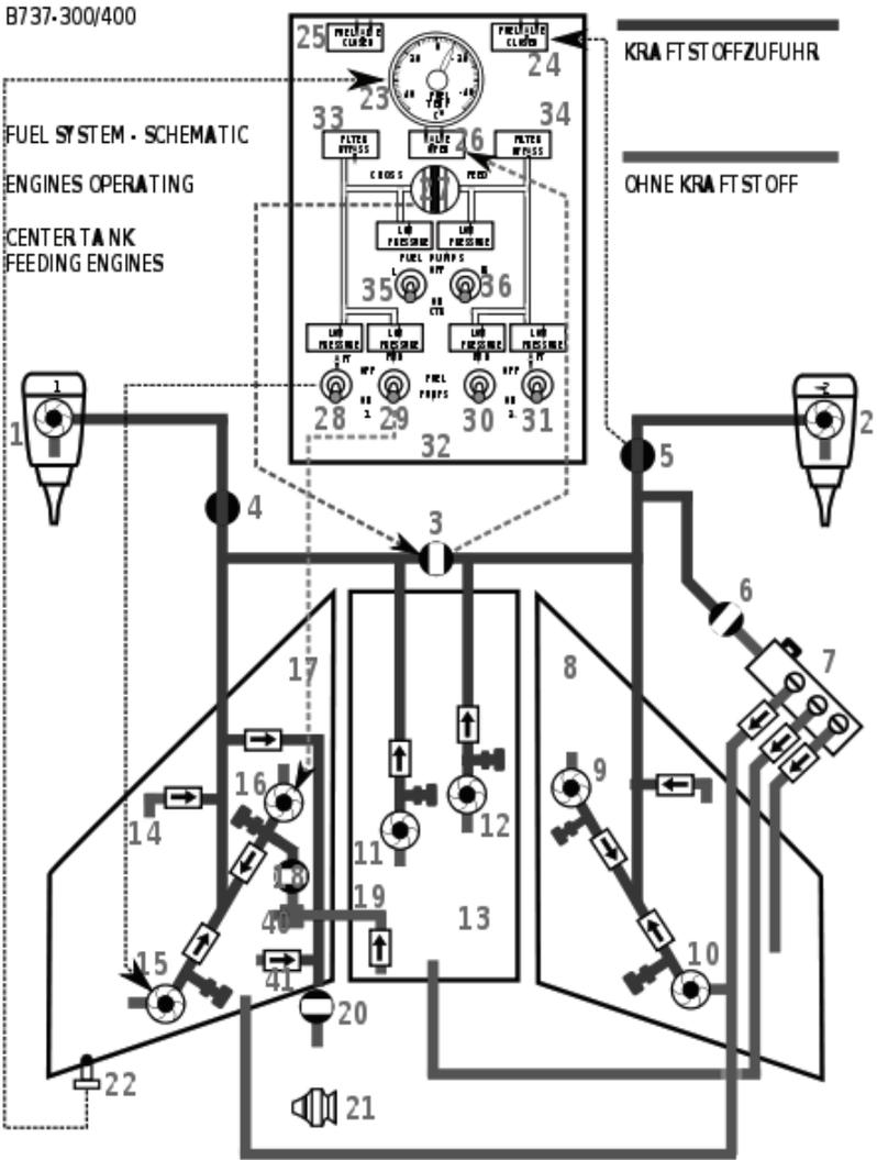
Figure 5.16: Diagrammatic representation of the Boeing 737-300 fuel system. © User:RosarioVanTulpe / Wikimedia Commons / Public Domain.
