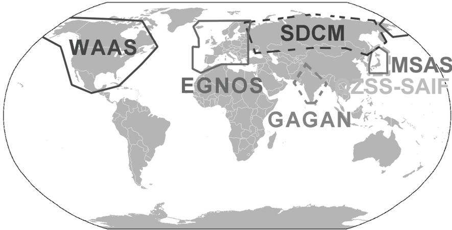
Figure 11.9: Service Areas of Satellite Based Augmentation Systems (SBAS). © User:Persimlex / [Wikimedia Commons](#) / [CC-BY-SA-3.0](#).
