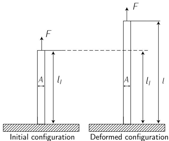
Figure 4.7: Normal deformation. Adapted from FRANCHINI *et al.* [2].
