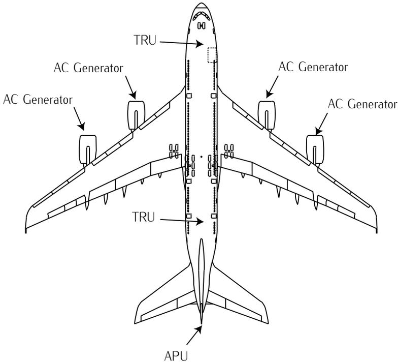
Figure 5.15: A380 power system components.
