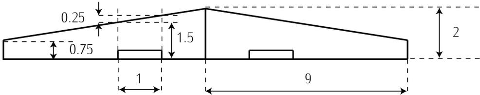
Figure 3.34: Plant-form of the wing (dimensions in meters).
