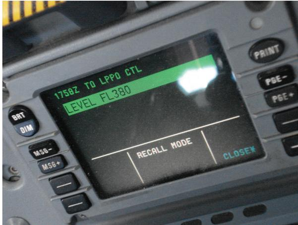
Figure 11.2: Datalink control and display unit (DCDU) on an Airbus A330. © User:SempreVolando / [Wikimedia Commons](#) / [CC-BY-3.0](#).
