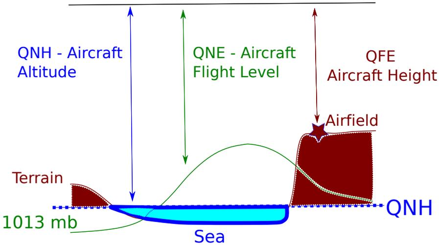
Figure 5.2: Diagram of barometric settings.
