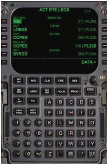
(a) FMS Control Display Unit of a B-737-300. © User:PresLoiLoi / Wikimedia Commons / CC-BY-SA-3.0.
