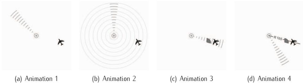
Figure 11.13: Spatial modulation in VORs. A radio beam sweeps (30 times per sec.). When the beam is at the local magnetic north, the station transmits a second, omni-directional signal. The time between the omni-directional signal and instant in which the aircraft receives the directional beam gives the angle from the VOR station (105 deg in this case).
