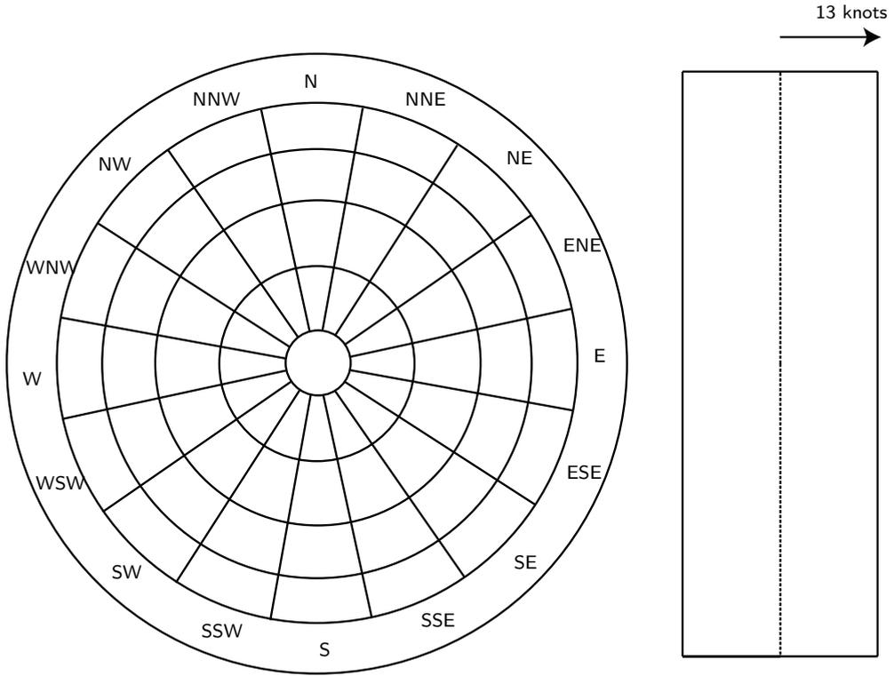
Figure 9.19: Wind Rose coordinate system and template with cross wind component limits of 13 knots.
