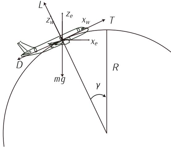
Figure 7.4: Aircraft forces in a vertical loop.
