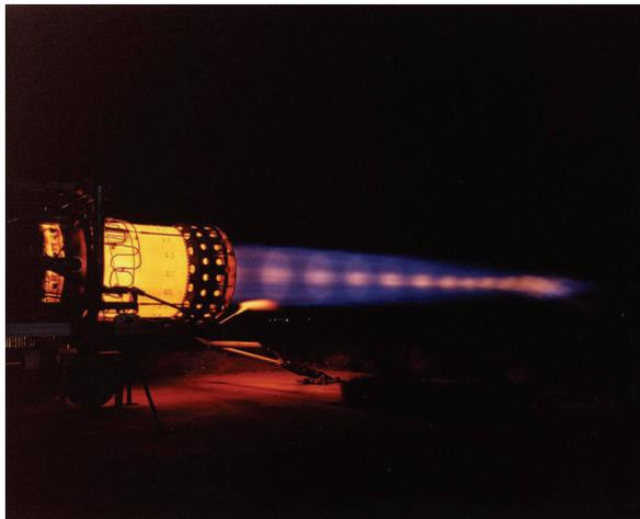
Figure 6.16: A statically mounted Pratt & Whitney J58 engine with full after-burner.
