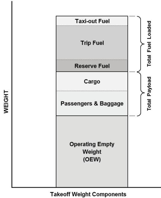
Figure 7.8: Take-off weight components. © Mohsen Alshayef / [Wikimedia Commons](https://commons.wikimedia.org/wiki/File:Takeoff_weight_components.png) / CC-BY-SA-3.0.
