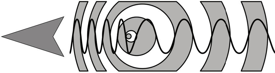
Figure 11.3: Doppler effect: change of wavelength caused by motion of the source. © User:Tkarcher / [Wikimedia Commons](#) / CC-BY-SA-3.0.
