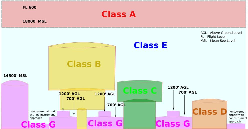
Figure 10.11: Classes of Airspace in the USA (altitudes AGL in feet).
