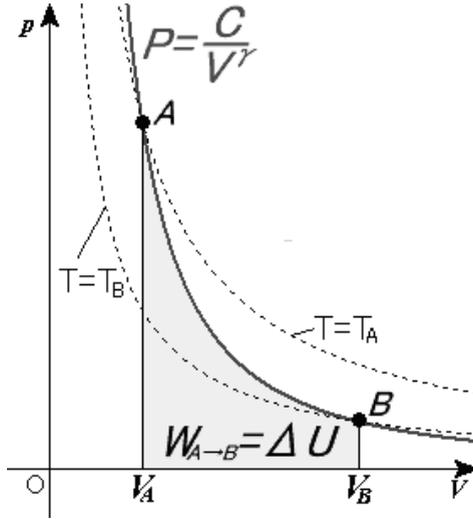
Figure 6.3: Sketch of an adiabatic process. © Yuta Aoki / [Wikimedia Commons](https://commons.wikimedia.org/wiki/File:Adiabatic_process.png) / CC-BY-SA-3.0.
