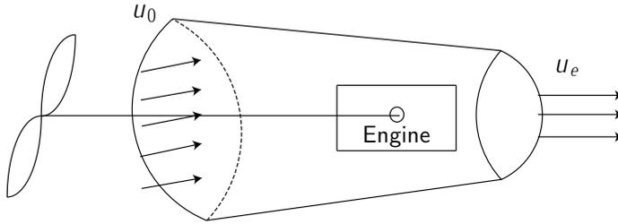
Figure 6.1: Propeller schematic.
