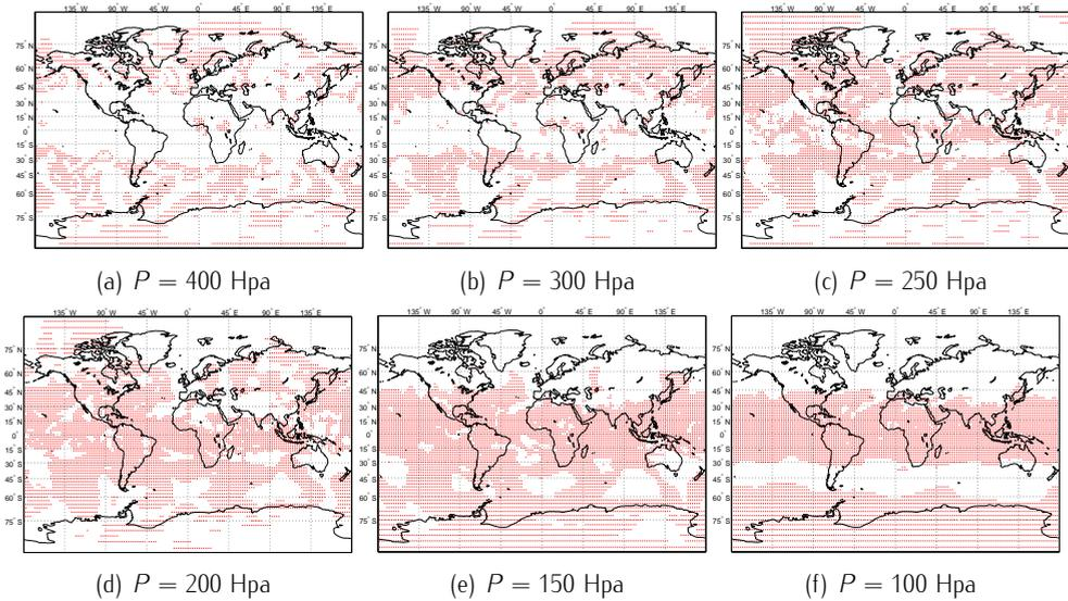
Figure 8.12: Longitude–latitude grid points that present favorable conditions for persistent contrail formation for different barometric altitudes.
