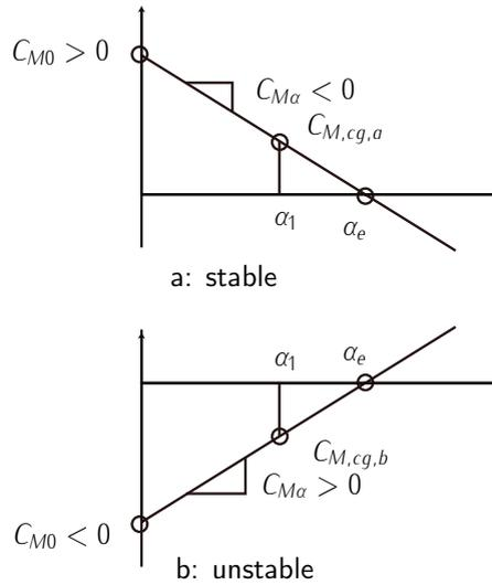
Figure 7.14: Longitudinal stability. Adapted from FRANCHINI and GARCÍA [3].
