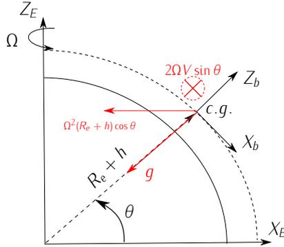
Figure 11.20: Inertial Navigation System, including gravitational acceleration, Coriolis acceleration ( $2\Omega V$ ), and centrifugal acceleration ( $\Omega^2(R_e + h)\cos(\theta)$ ).
