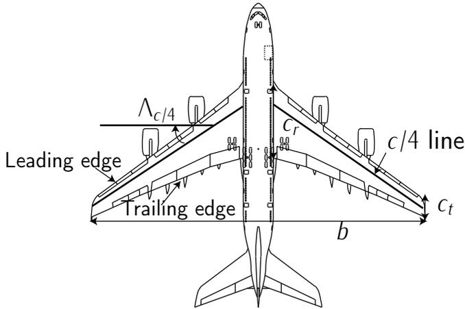
Figure 3.20: Wing geometry
