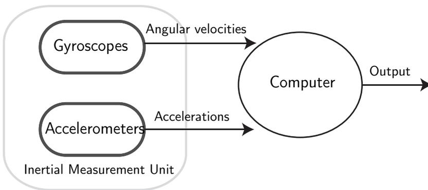
Figure 11.4: Scheme of an Inertial Navigation System (INS). The output refers to position, attitude, and velocity.
