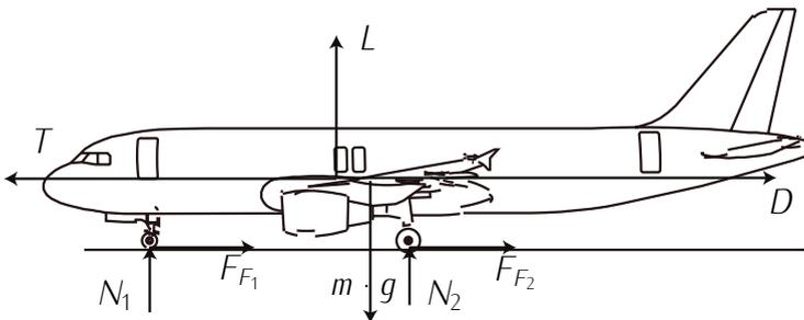
Figure 9.23: Forces during taking off run.
