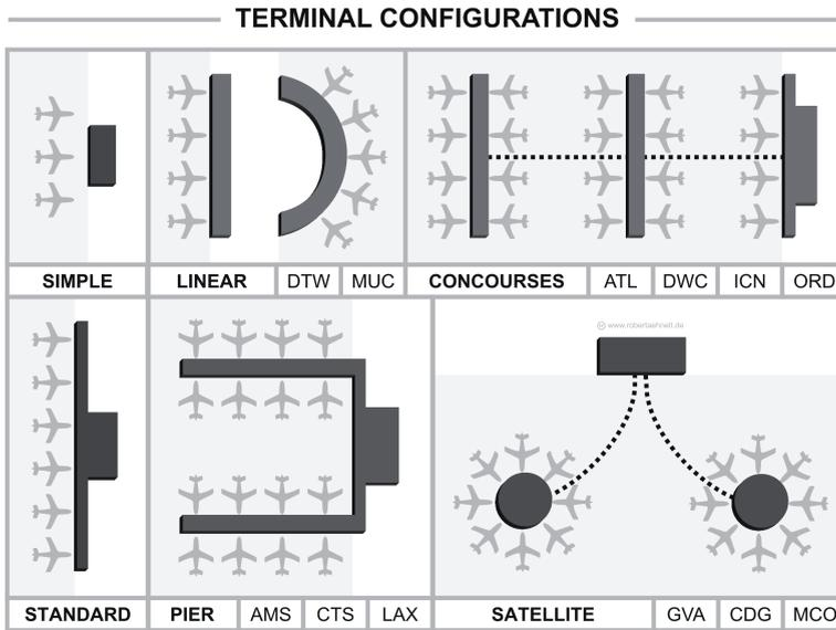
Figure 9.10: Typical terminal configurations. © Robert Aehnelt. / [Wikimedia Commons](https://commons.wikimedia.org/wiki/File:Terminal_configuration.png) / CC-BY-SA-3.0.
