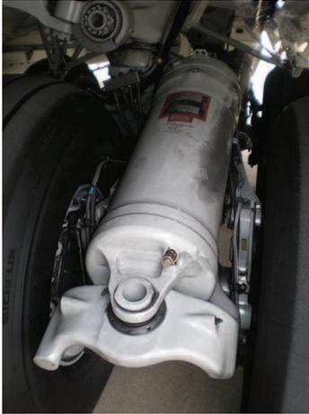
(a) Rear landing gear hydraulics.
