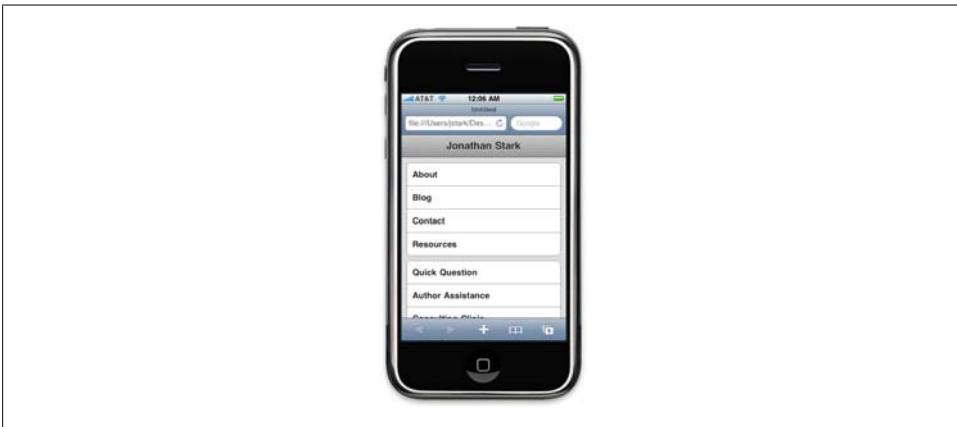
Figure 2-7. Gradients, text shadows, and rounded corners start to transform your web page into a native-looking iPhone app
