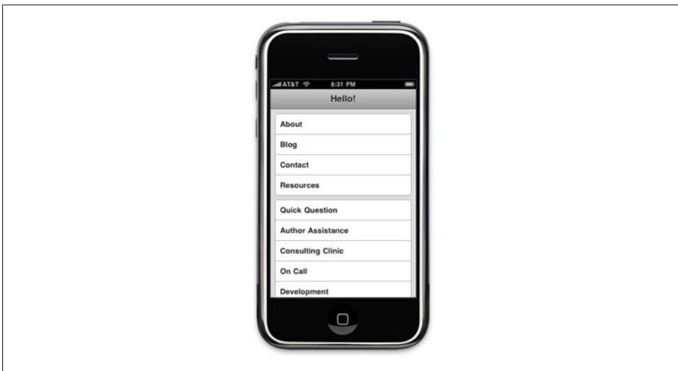
Figure 3-13. Full screen mode gives you about 25% more screen real estate and allows you to customize the appearance of the status bar
