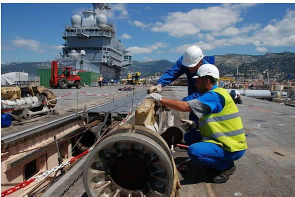
Figure 5.33: Piston of a steam catapult from the aircraft carrier Charles de Gaulle.
