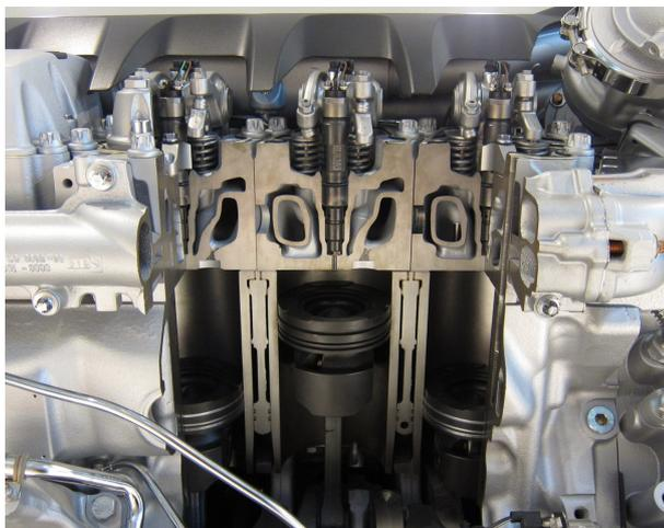
Figure 2.1: A cutaway in a truck engine reveals three pistons in their cylinders. A closed system is a useful tool for studying the air trapped in a cylinder. The photographed engine is a diesel V8 from MAN.
