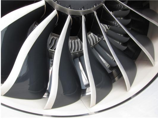
Figure 4.17: Air intake of one of the four General Electric GENX-2B turbofans equipping a Boeing 747-8. The two-color fan blades are visible in the foreground; behind, the air flow is divided between the compressor inlet (internal) and the cold flow rectifier stators (external).
