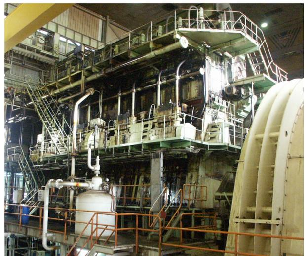
Figure 7.16: A nine-cylinder *Sulzer RTA76* Diesel engine producing 25 MW of power at 95 rpm. This unit is installed here in a factory but the model is commonly used to propel merchant ships.
