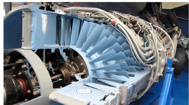
Figure 4.20: Compressor of a disassembled SNECMA Atar turbojet engine (1948). Air flows from the left to the center of the image.
