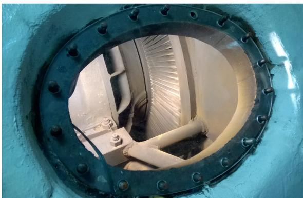
Figure 8.14: Inspection window of one of the low-pressure turbines (power approximately  $25 \text{ MW}$ ) of the aircraft carrier *USS Hornet* launched in 1943.
