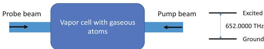
**Fig. 5.2** Saturated absorption spectroscopy needs two laser beams: a probe beam and a pump beam. Not pictured is the photodiode with which we monitor the transmission of the probe beam
