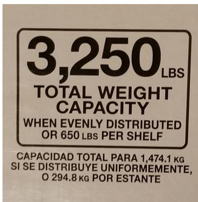
As shown in the picture, a shelving system is rated to hold a total weight of 3,250 pounds, or 650 pounds on each of its five shelves. The metric equivalents printed on the box are 1,474.1 kilograms and 294.8 kilograms.
