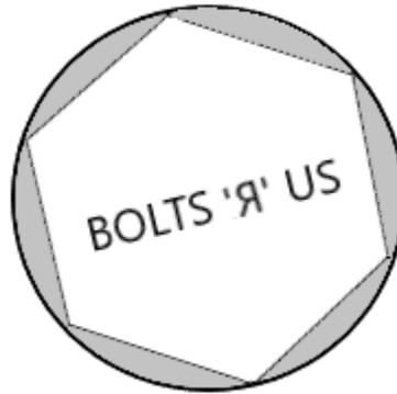
7. The hexagonal head of a bolt fits snugly into a circular cap with a circular hole with inside diameter 46 mm as shown in this diagram. Opposite sides of the bolt head are 40 mm apart. Find the total empty area in the hole around the edges of the bolt head.
