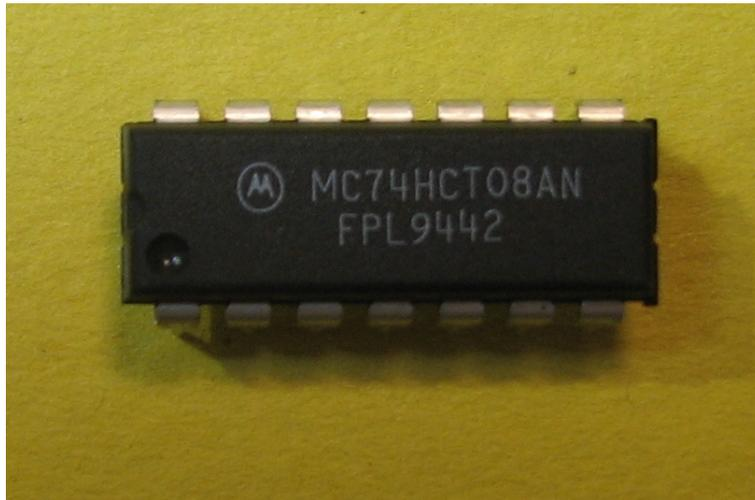
Figure 4-6: 7408 chip, circle indicates top of chip.
