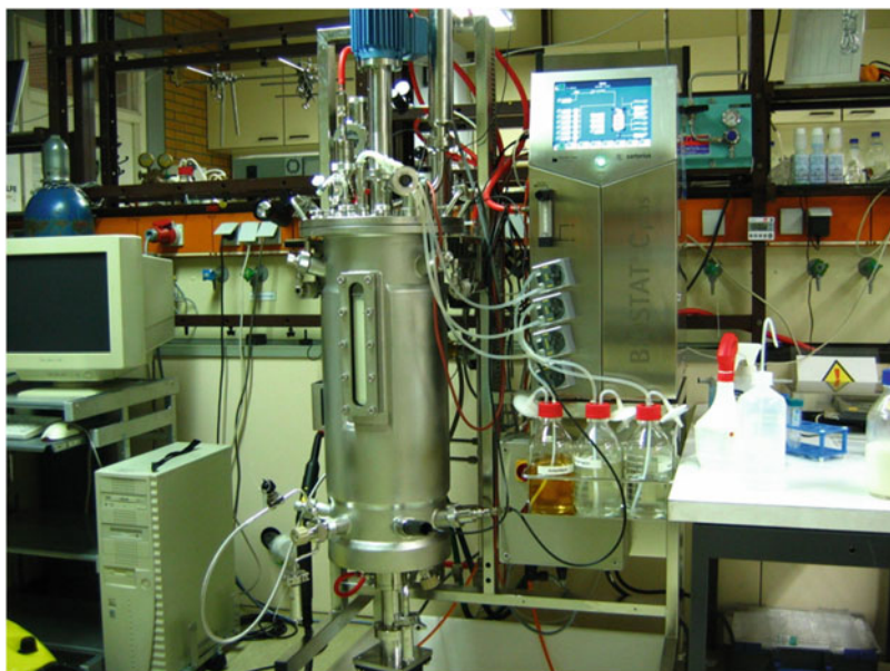
Fig. 7.12 A stirred-tank bioreactor for the controlled growth of microorganisms, with devices for stirring, O 2 and pH control, feeding-in of substrate, base, and antifoam
