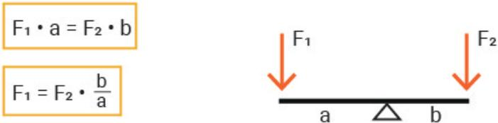
*Figure 3-5: Archimedes' principle of the level*
