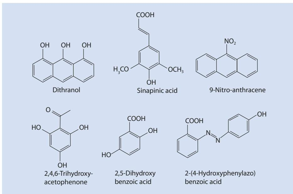
■ Fig. 3.14 Typical matrix molecules. Dithranol (also known as anthralin and Cignolin) is shown in its enol-form which is in tautomeric equilibrium with the keto-form
