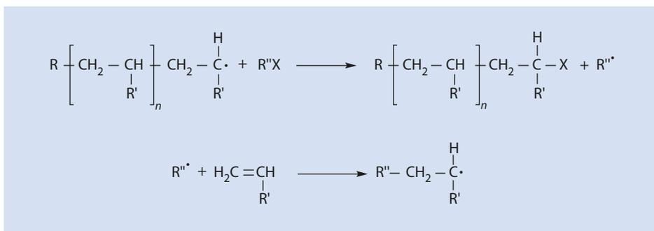
Fig. 9.4 Example of chain transfer
