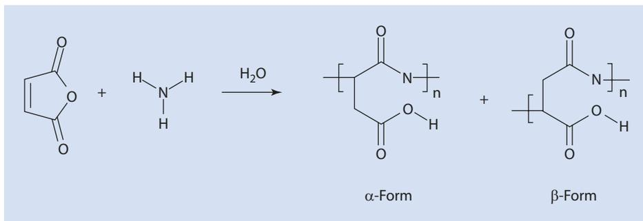
■ Fig. 21.7 Synthesis of polyaspartic acid from maleic acid anhydride, ammonia, and water
