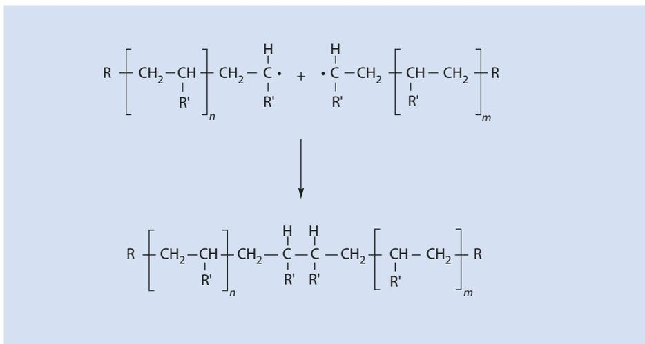
Fig. 9.3 Termination of chain growth by radical combination
