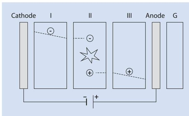
■ **Fig. 22.10** Schematic representation of the electron and hole conduction through the organic layers of an OLED
