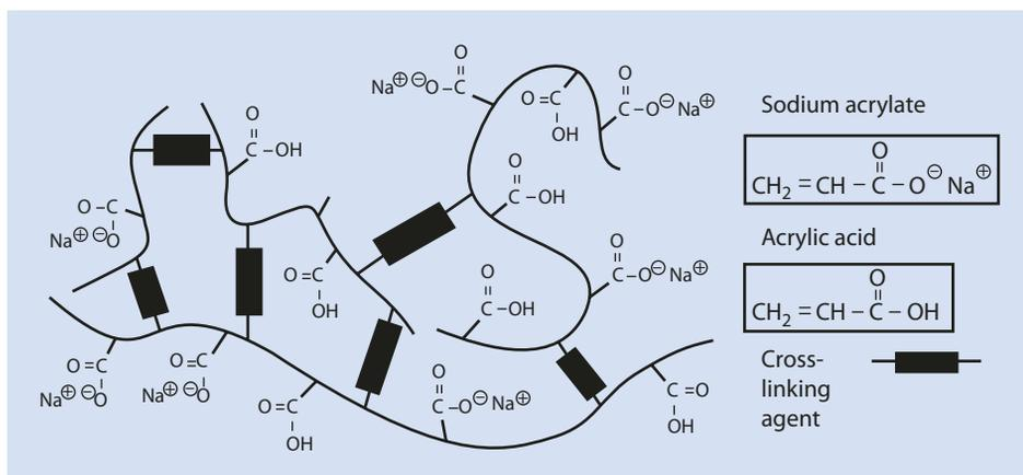
Fig. 19.19 Structure of cross-linked sodium polyacrylate (super-absorber)
