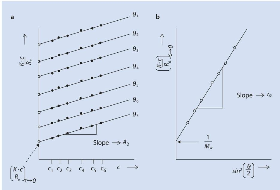
■ Fig. 3.12 Twofold extrapolation for a set of light scattering data. (a) Extrapolation to a zero concentration  $c_2 = 0$ . (b) Then to a scattering angle  $\theta = 0$ .  $c$  Polymer concentration  $c_i$ , indices indicate different polymer concentrations
