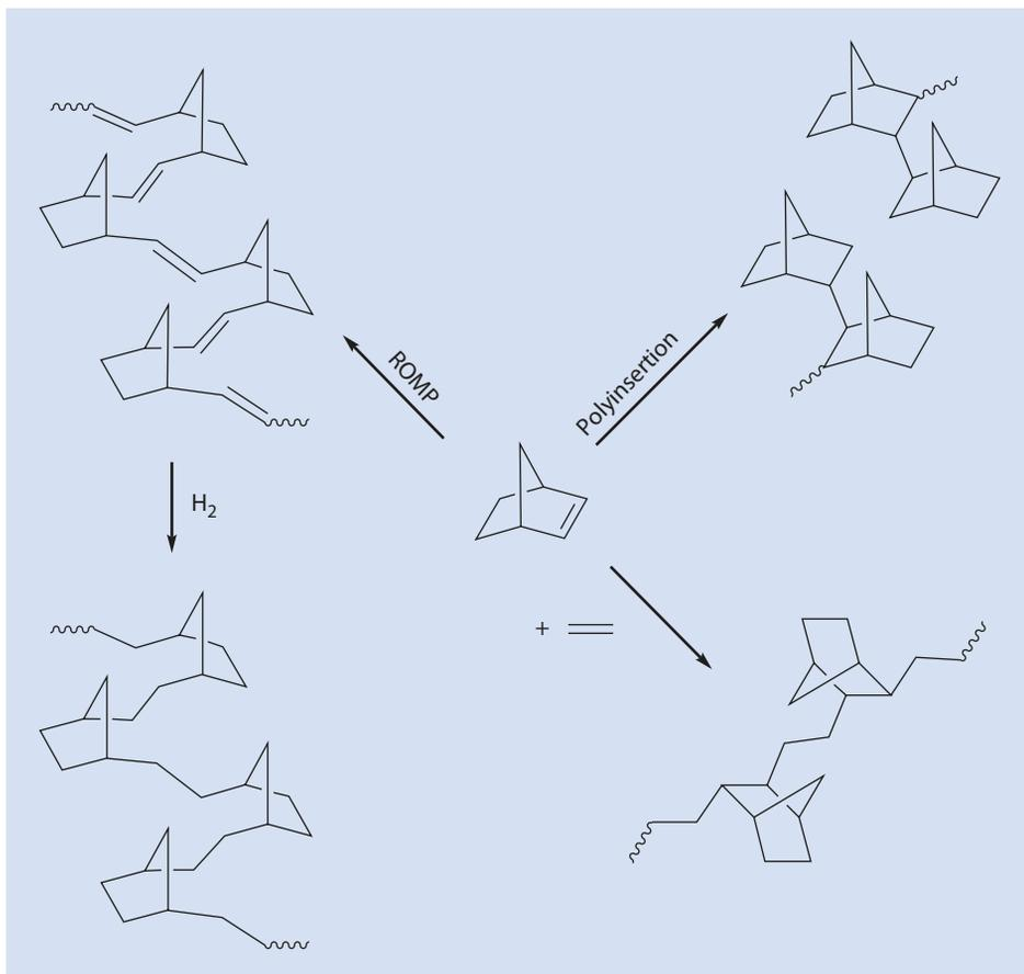
Fig. 11.33 Polymers based on norbornene
