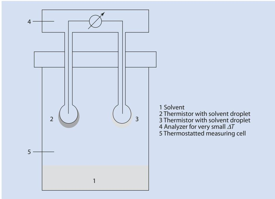
Fig. 3.5 Simplified sketch of a vapor pressure osmometer
