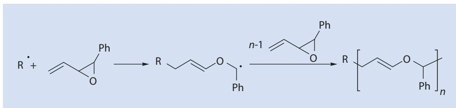
Fig. 12.3 RROP of vinyl oxiranes. Ph: phenyl
