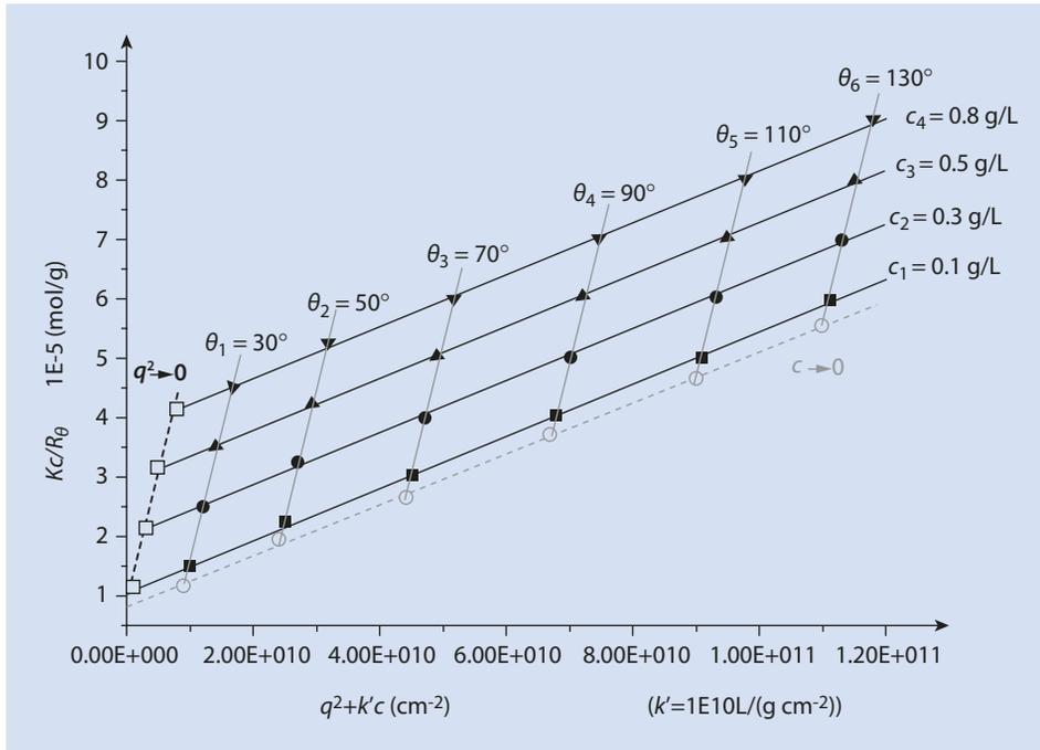
Fig. 3.13 Zimm-diagram from light scattering measurements on a polymer in toluene. The extrapolations yield the molar mass  $M_w = 121$  kg/mol, the radius of gyration  $r_G = 124$  nm, and the second virial coefficient  $A_2 = 2.2 \cdot 10^{-4}$  mol cm<sup>3</sup> g<sup>-2</sup>.  $c$  polymer concentration  $c_i$  indices refer to the different polymer concentrations
