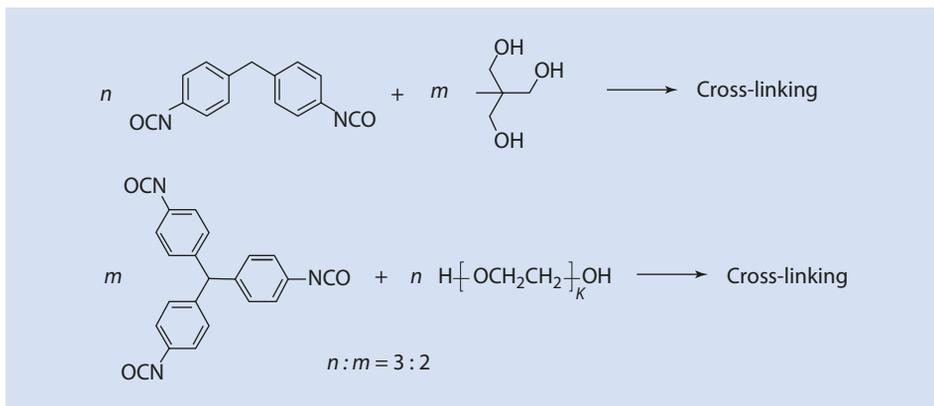
Fig. 8.20 Formation of polyurethane networks
