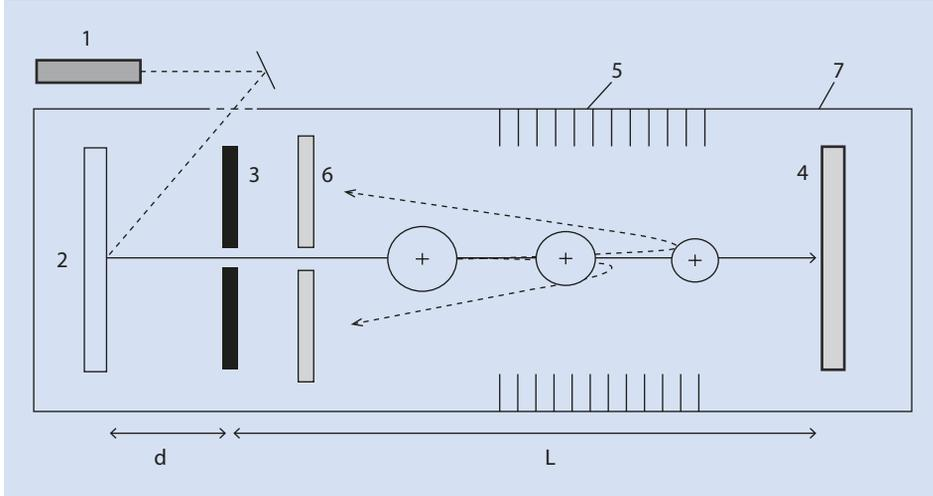
■ **Fig. 3.15** Setup of a time-of-flight analyzer. (1) Laser, (2) sample holder, (3) accelerating electrode, (4) linear-detector, (5) reflectron, (6) reflectron-detector, (7) vacuum chamber,  $d$  acceleration section,  $L$  field-free flight distance (linear), (*dashed line*) flight routes (for the function of the optional reflectron, ion mirrors – see text)
