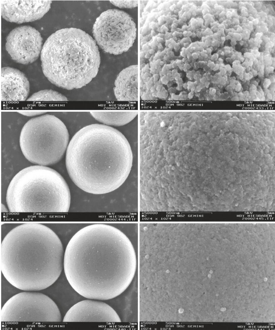
■ Fig. 3.18 Electron micrographs at various magnifications of SEC-gels with various pore sizes. (By kind permission of Polymer Standards Services GmbH, Mainz)
