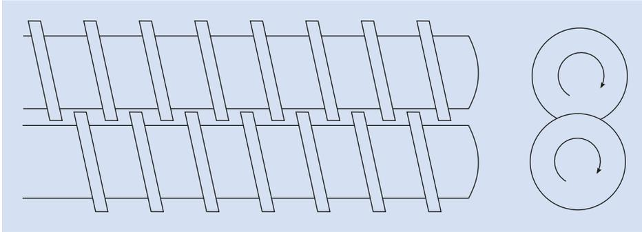
■ Fig. 17.2 Principle of a twin-screw extruder
