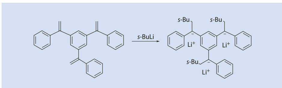
Fig. 10.66 An example of a trifunctional initiator
