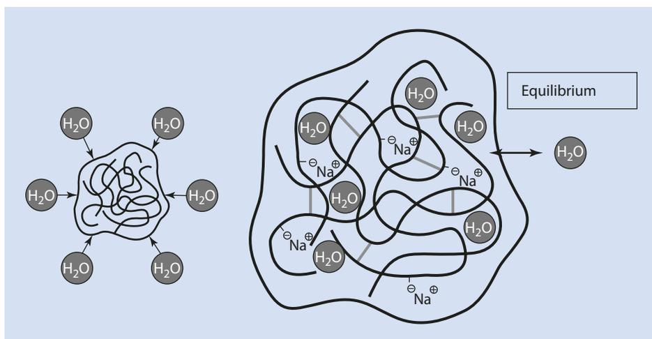
Fig. 19.20 Swelling of a super-absorber produced by osmosis
