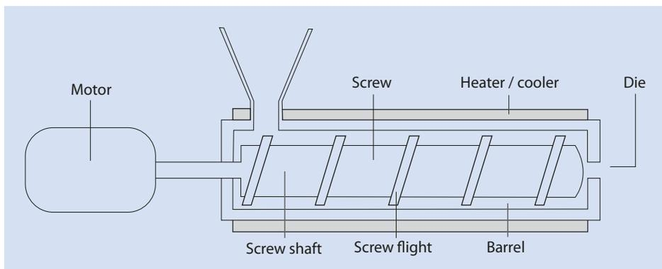
■ Fig. 17.1 Simplified diagram of an extruder
