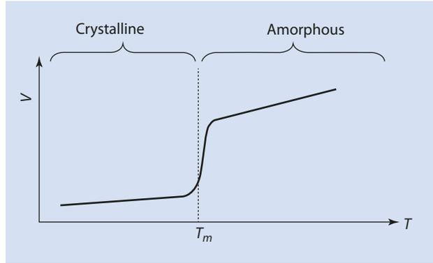
Fig. 4.4 Sketch showing the volume change at a glass transition.  $T_G$  glass transition temperature
