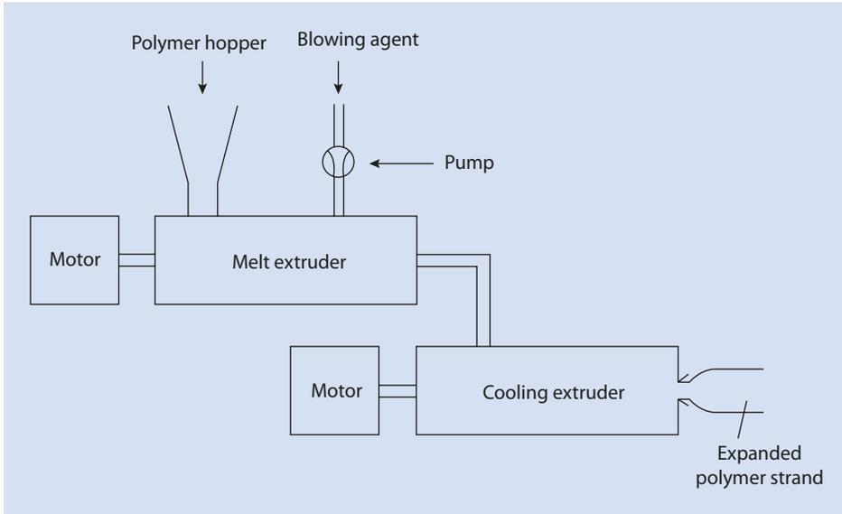
■ Fig. 17.12 Tandem extruder arrangement for foam extrusion
