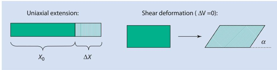
■ Fig. 4.2 Schematic representation of the shape change under uniaxial stress by  $\Delta x$  or shear stress by a shear angle  $\alpha$
