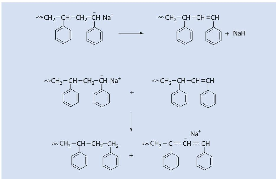
Fig. 10.71 Formation of an unreactive 1,3-diphenyl allyl anion
