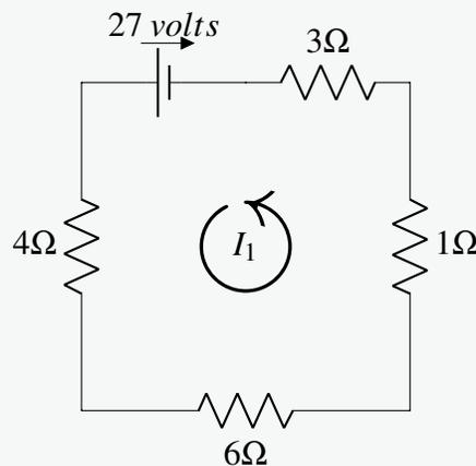
**Solution.** Begin in the top left corner this time, and trace the circuit in the counter clockwise direction. At the first resistor, multiplying resistance and current gives  $4I_1$ . Continuing in this way through the four
