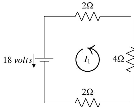
The jagged lines ( $\text{---}\text{---}\text{---}$ ) denote resistors and the numbers next to them give their resistance in ohms, written as  $\Omega$ . The voltage source ( $\text{---}|$ ) causes the current to flow in the direction from the shorter of the two lines toward the longer (as indicated by the arrow). The current for a circuit is labelled  $I_k$ .
