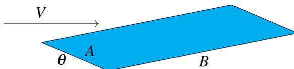
The angle  $\theta$  is called the angle of incidence,  $B$  is the span of the wing and  $A$  is called the chord. Denote by  $l$  the lift. Then this should depend on various quantities like  $\theta, V, B, A$  and so forth. Here is a table which indicates various quantities on which it is reasonable to expect  $l$  to depend.
