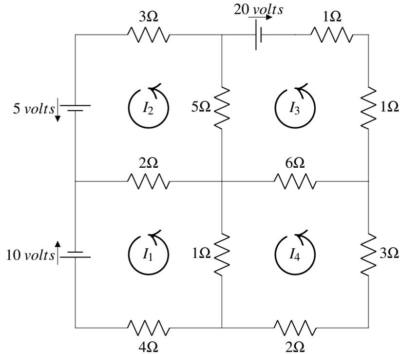
The current in amps in the four circuits is denoted by  $I_1, I_2, I_3, I_4$  and it is understood that the motion is in the counter clockwise direction. If  $I_k$  ends up being negative, then it just means the current flows in the clockwise direction.
