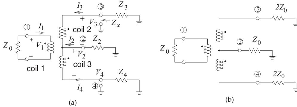
**Figure 5-22:** Magnetic transformer hybrid with each coil having the same number of windings: (a) showing general loading impedance; and (b) optimum loading to function as a  $180^\circ$  hybrid with Port 2 (terminal 2 to ground) isolated and the balanced input at Port 1. For example, an antenna could be attached to Port 1. A common flux passes through the three coils.
