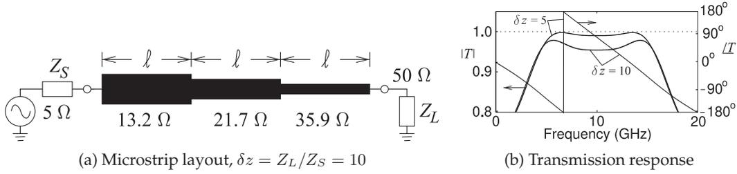
**Figure 7-11:** Maximally flat transmission line transformer designed in Example 7.3. At 10 GHz each section is of length  $\ell = \lambda_g/4 = 2.83$  mm where  $\lambda_g$  is the midband wavelength.
