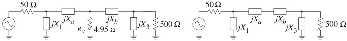
**Figure 6-22:** Matching network problem of Example 6.7. **Figure 6-23:** Final matching network in Example 6.7.
