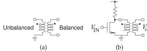
**Figure 5-26:** Marchand balun: (a) coaxial form of the Marchand balun; and (b) its equivalent circuit.
