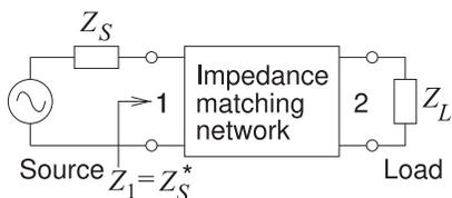
**Figure 6-42:** Matching problem with the matching network between the source and load designed for maximum power transfer.  $Z_S = R_S + jX_S = 29.36 - j12.05$ ,  $Z_1 = R_1 + jX_1 = Z_S^* = R_S - jX_S = 29.36 + j12.05$ , and  $Z_L = R_L + jX_L = 132.7 - j148.8$ .
