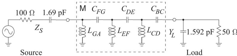
**Figure 7-7:** Matching network  $M$  in Example 7.1.
