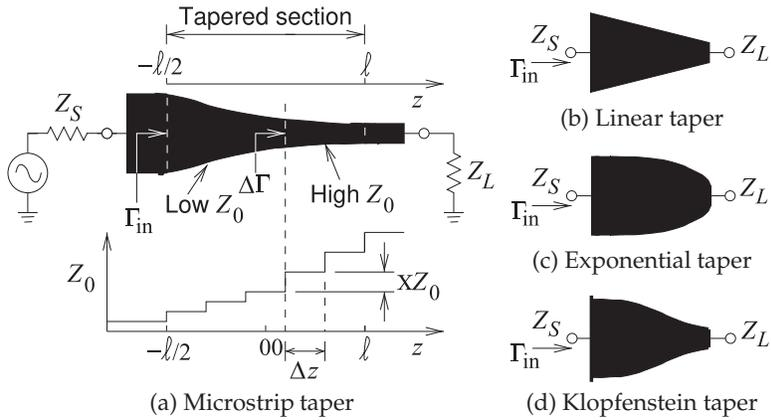
**Figure 7-14:** Tapered impedance transformers with length  $\ell$ . The width of the microstrip line is approximately inversely proportional to the characteristic impedance of the line. (Here  $Z_L > Z_S$  and both  $Z_L$  and  $Z_S$  are resistive.)
