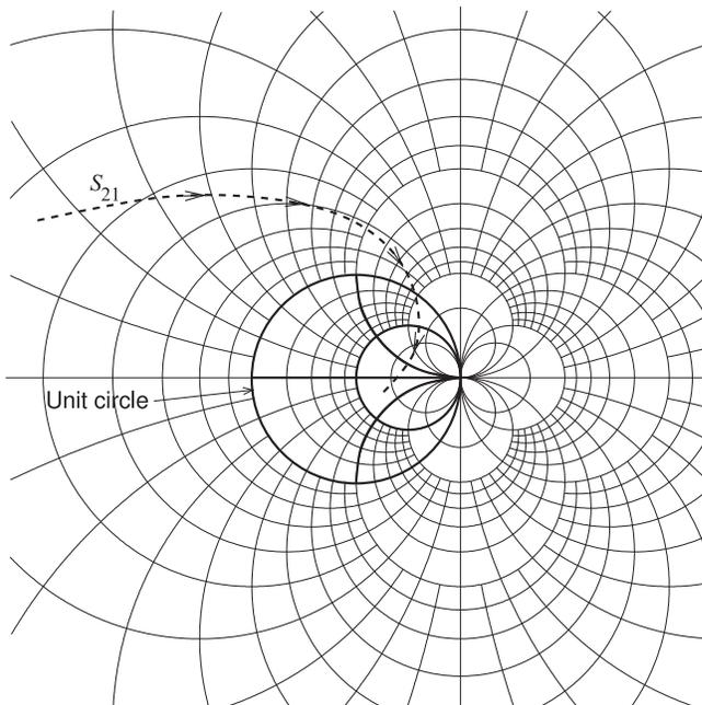
**Figure 3-32:** Expanded Smith chart used to plot scattering parameters with a magnitude greater than 1. The forward transmission parameter,  $S_{21}$ , of a transistor is shown with the arrows in the direction of increasing frequency. The unit circle of a conventional Smith chart is shown
