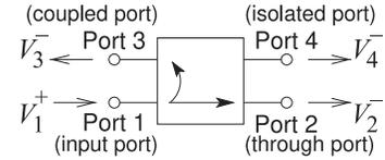
Figure 2-28: Schematic of a directional coupler.
