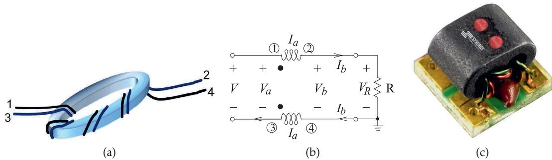
**Figure 5-30:** A broadband RF balun as coupled lines wound around a ferrite core: (a) physical realization (the wires 1–2 and 3–4 form a single transmission line); (b) equivalent circuit using a wire-wound transformer (the number of primary and secondary windings are equal); and (c) packaged as a module (Model TM1-9 with a frequency range of 100–5000 MHz. Copyright Synergy Microwave Corporation, used with permission [34]).
