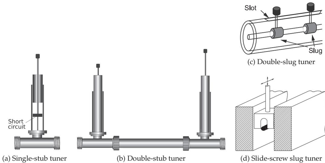
Figure 6-38: Laboratory tuners.
