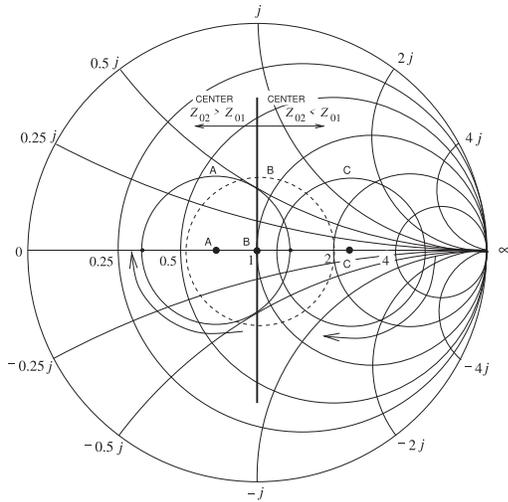
**Figure 3-36:** The locus of the input reflection coefficient normalized to  $Z_{02}$  of a terminated line of characteristic impedance  $Z_{01}$ . The locus is with respect to the electrical length of the line and the arrows show the direction of rotation of the reflection coefficient. (Note that for the same terminating impedance the radii will also change, but this is not shown here.)
