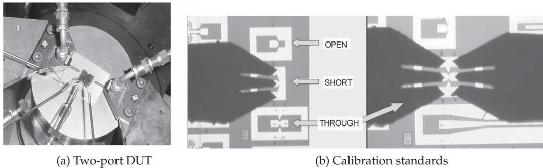
**Figure 4-14:** Two-port measurements: (a) two-port device under test with DC needle probes at the bottom and GSG probes on the left and right; and (b) open, short, and through calibration standards with GSG probes.
