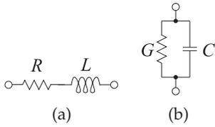
**Figure 5-3:** Loss elements of practical inductors and capacitors: (a) an inductor has a series resistance  $R$ ; and (b) for a capacitor, the dominant loss mechanism is a shunt conductance  $G = 1/R$ .
