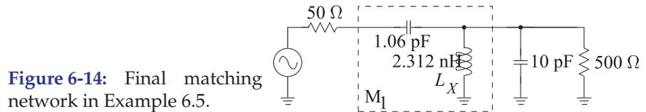
**Figure 6-14:** Final matching network in Example 6.5.
