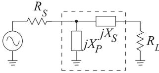
**Figure 6-10:** Two-element matching network topology for  $R_S > R_L$ .
