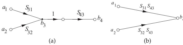
**Figure 3-5:** Signal flow graph simplification eliminating a variable.
