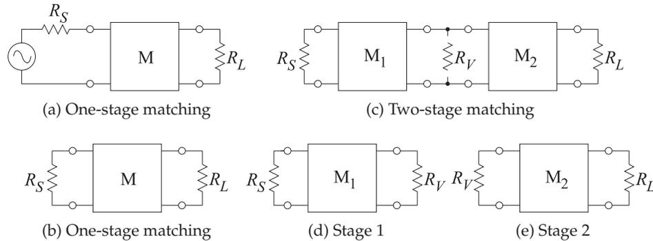
**Figure 6-18:** Matching in stages: (a) matching network  $M$  matching  $R_S$  to  $R_L$ ; (b) without an explicit source; (c) two-stage matching with a virtual resistor  $R_V$ ; (d) matching  $R_S$  to  $R_V$ ; and (e) matching  $R_V$  to  $R_L$ .
