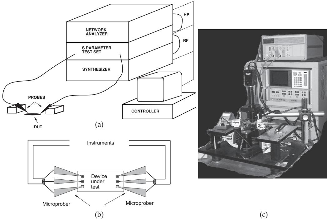
**Figure 4-3:** *S* parameter measurement system: (a) shown in a configuration to do on-chip testing; (b) details of coplanar probes with a GSG configuration and contacting pads; and (c) a vector network analyzer in the background with probe station including camera.
