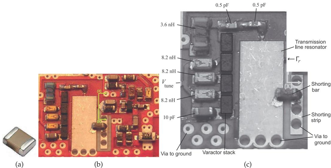
**Figure 5-6:** Circuit board showing the use of surface-mount components: (a) chip resistor or capacitor with metal terminals at the two ends; (b) populated RF microstrip circuit board of a 5 GHz voltage-controlled oscillator [7] (the larger components have dimensions  $1.6 \text{ mm} \times 0.8 \text{ mm}$ ); and (c) identification of several components including a varactor stack with four varactor diodes and a shorting bar that is a  $0 \Omega$  resistor.
