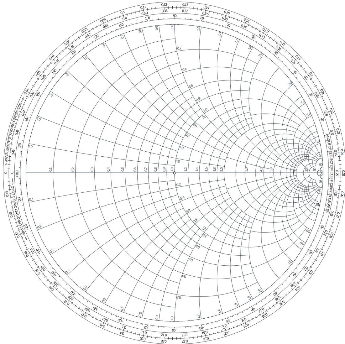
**Figure 3-18:** Impedance Smith chart. Also called a normalized Smith chart since resistances and reactances have been normalized to the system reference impedance  $Z_{REF}$ :  $z = Z/Z_{REF}$ .
