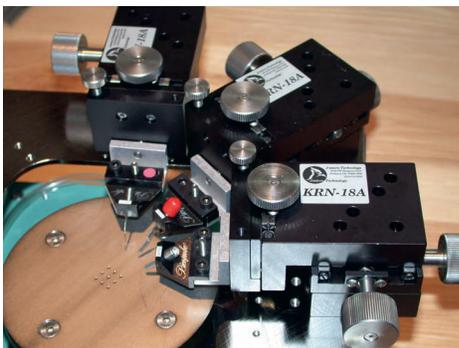
**Figure 4-4:** Micropositioners used with coplanar probes. Used with permission of J MicroTechnology, Inc.
