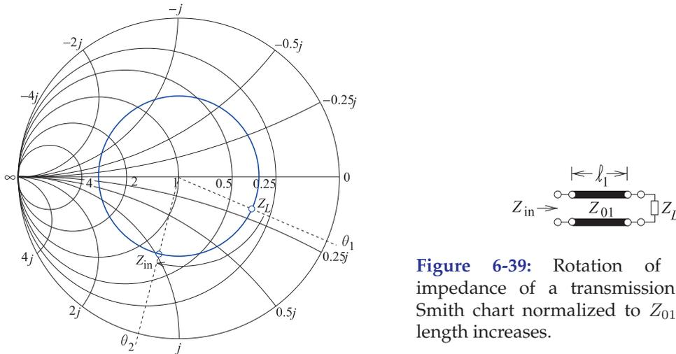
Figure 6-39: Rotation of the input impedance of a transmission line on a Smith chart normalized to  $Z_{01}$  as the line length increases.
