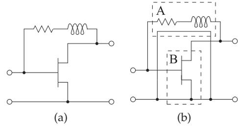
**Figure 2-9:** Series-parallel connection of two-ports.
