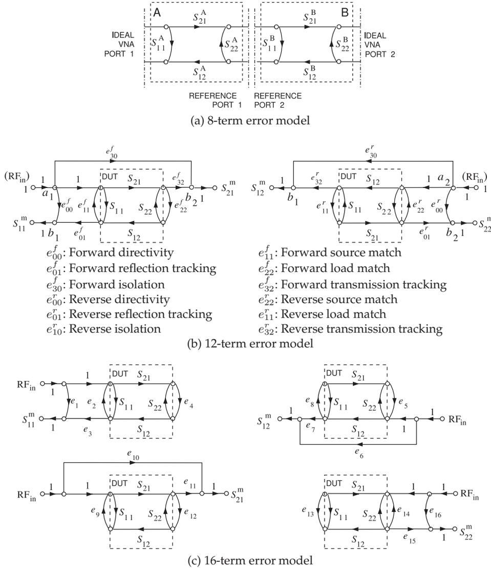
**Figure 4-10:** Two-port error models: (a) SFG representation of the 8-term two-port error model (1968) [1]); (b) SFG of the 12-term two-port error model (1978) [7]; and (c) SFG of the 16-term two-port error model (circa 1979) [8].  $S_{ij}^m$  are the raw  $S$  parameter measurements,  $S_{ij}$  are the  $S$  parameters of the DUT, and  $e_{ij}$ ,  $e_{ij}^r$ , and  $e_{ij}^f$  are error  $S$  parameters determined during calibration.
