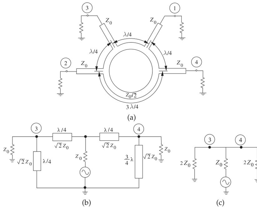
**Figure 5-40:** Rat-race hybrid with input at Port 1, outputs at Ports 3 and 4, and virtual ground at Port 2: (a) implementation as a planar circuit; (b) transmission line model; and (c) equivalent circuit model.
