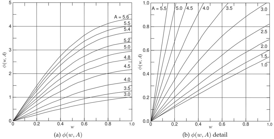
**Figure 7-15:** Klopfenstein taper function  $\phi(w, A)$  used in designing a taper segment. The taper has length  $\ell$ ,  $z$  is the coordinate at the center of a taper segment, the center of the taper is at  $z = 0$ , and  $\phi(-w, A) = -\phi(w, A)$ ,  $w = 2z/\ell$ .
