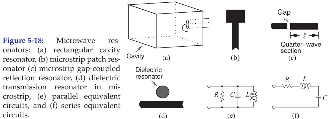
**Figure 5-18:** Microwave resonators: (a) rectangular cavity resonator, (b) microstrip patch resonator (c) microstrip gap-coupled reflection resonator, (d) dielectric transmission resonator in microstrip, (e) parallel equivalent circuits, and (f) series equivalent circuits.
