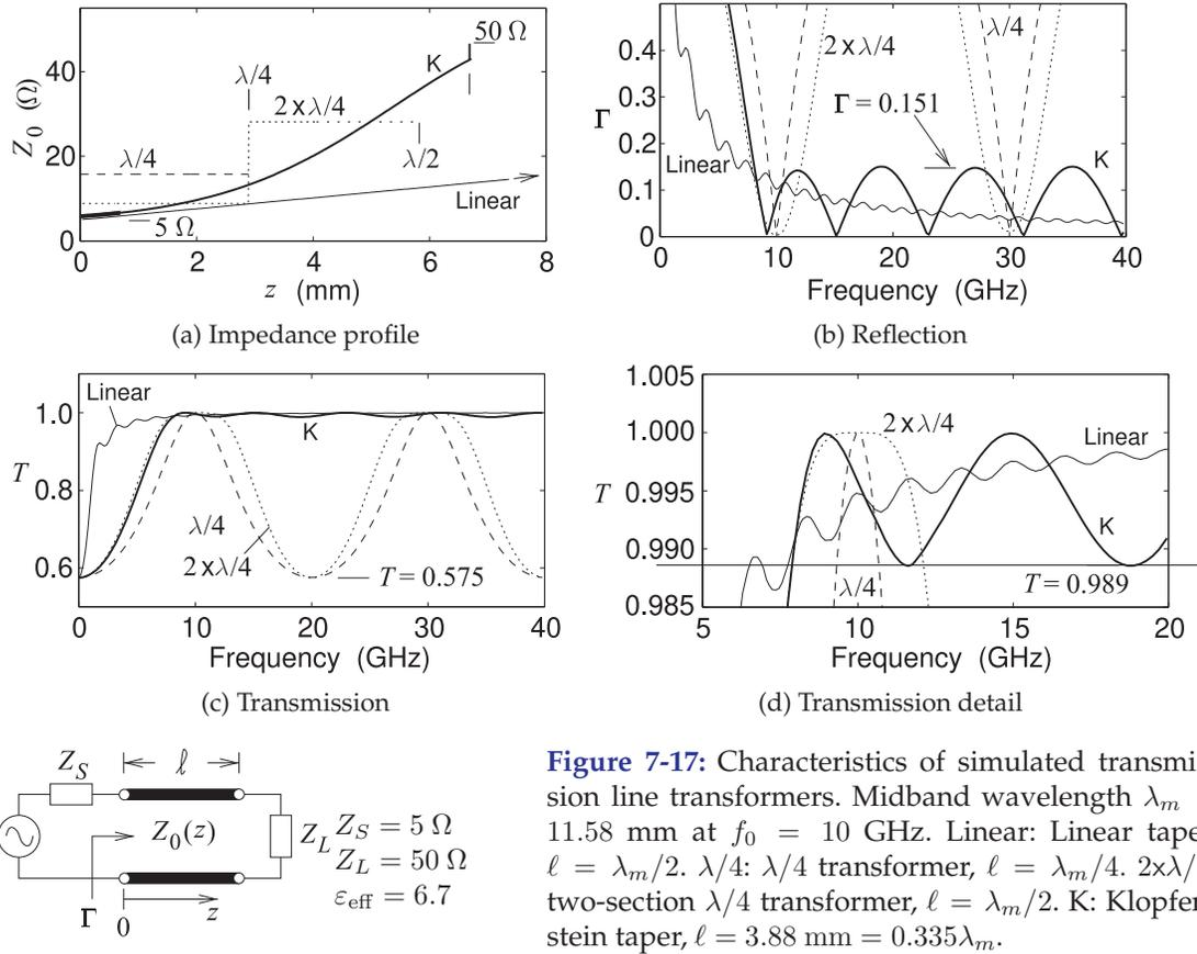
**Figure 7-17:** Characteristics of simulated transmission line transformers. Midband wavelength  $\lambda_m = 11.58$  mm at  $f_0 = 10$  GHz. Linear: Linear taper,  $\ell = \lambda_m/2$ .  $\lambda/4$ :  $\lambda/4$  transformer,  $\ell = \lambda_m/4$ .  $2 \times \lambda/4$ : two-section  $\lambda/4$  transformer,  $\ell = \lambda_m/2$ . K: Klopfenstein taper,  $\ell = 3.88$  mm =  $0.335\lambda_m$ .
