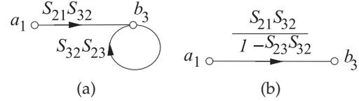
**Figure 3-8:** Signal flow graph with loop.
