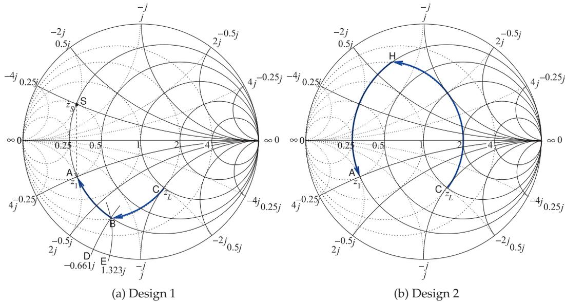
**Figure 6-35:** Smith chart-based designs used in Example 6.11. (50 Ω normalization used.)
