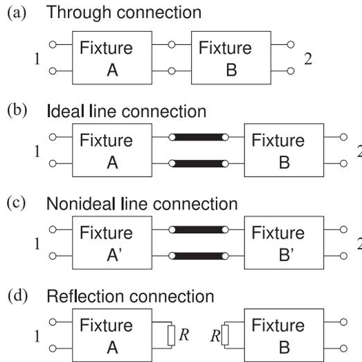
**Figure 4-11:** Measurement connections in two-port calibration using the TRL procedure: (a) through connection; (b) ideal line connection; (c) realistic configuration with nonidentical fixtures; and (d) with arbitrary reflection.
