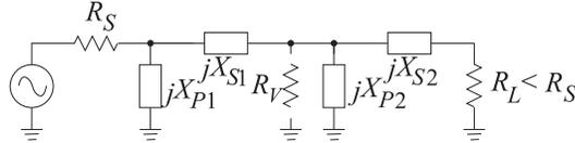
Figure 6-29: Cascaded L networks for broadband matching.
