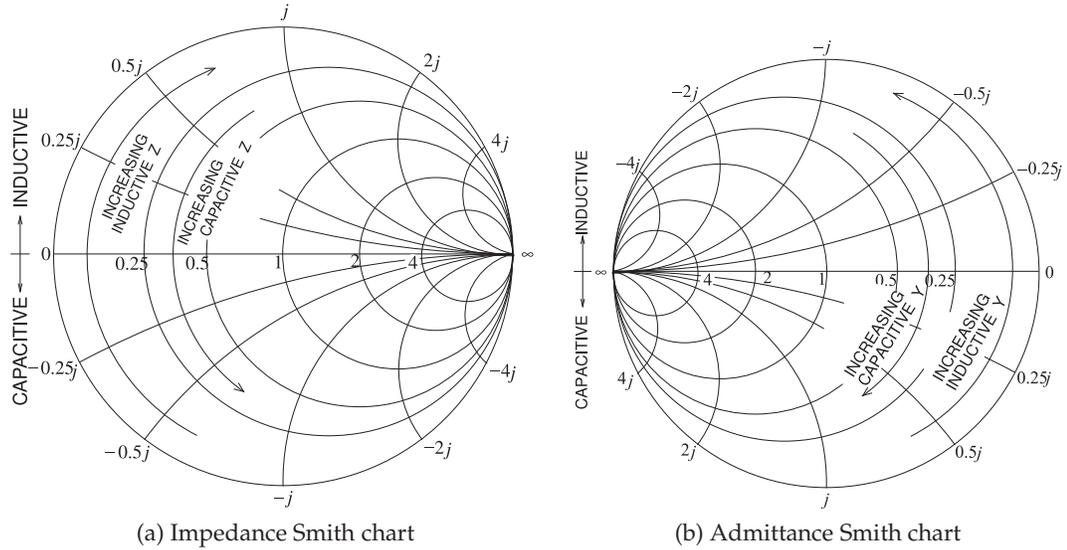
**Figure 6-30:** Inductive and capacitive regions on Smith charts. Increasing capacitive impedance ( $Z$ ) indicates smaller capacitance; increasing inductive admittance ( $Y$ ) indicates smaller inductance.
