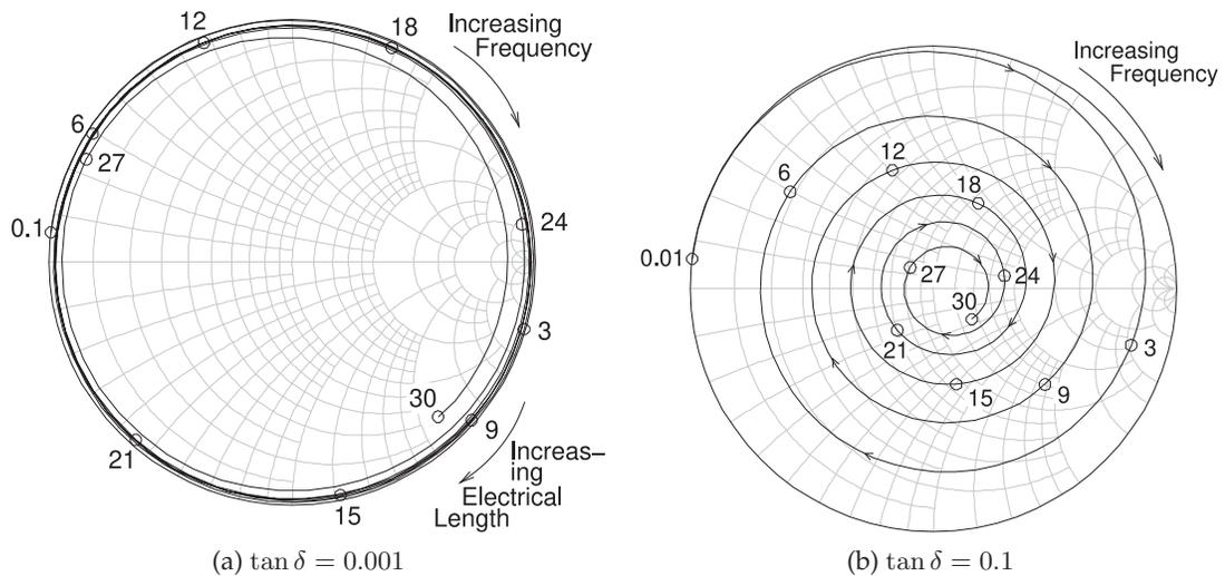
**Figure 3-31:** Smith chart plot of the reflection coefficient of the shorted 1 cm-long microstrip line in Figure 3-30: (a) a low-loss substrate with  $\tan \delta = 0.001$ ; and (b) a high-loss substrate with  $\tan \delta = 0.1$ . Frequencies are marked in gigahertz.
