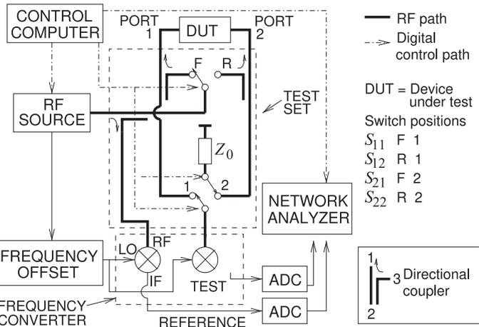
**Figure 4-2:** Vector network analyzer system with four receivers.
