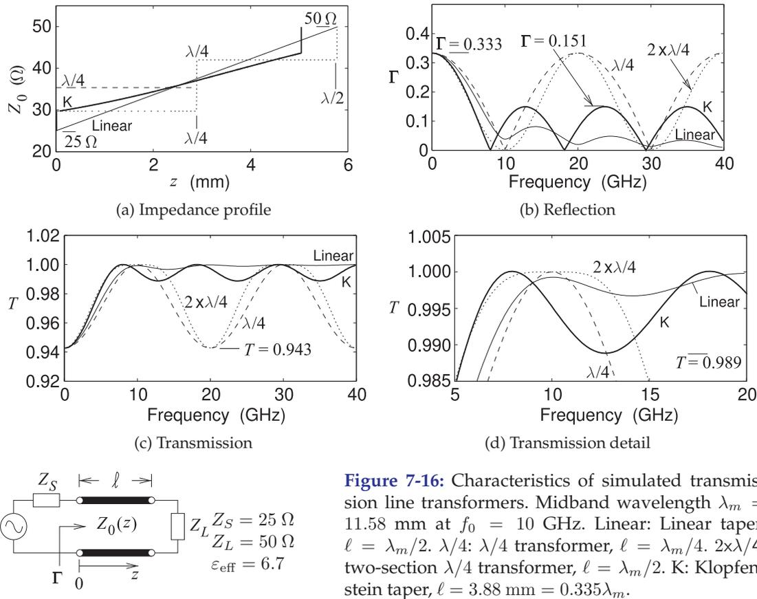
**Figure 7-16:** Characteristics of simulated transmission line transformers. Midband wavelength  $\lambda_m = 11.58$  mm at  $f_0 = 10$  GHz. Linear: Linear taper,  $\ell = \lambda_m/2$ .  $\lambda/4$ :  $\lambda/4$  transformer,  $\ell = \lambda_m/4$ .  $2 \times \lambda/4$ : two-section  $\lambda/4$  transformer,  $\ell = \lambda_m/2$ . K: Klopfenstein taper,  $\ell = 3.88$  mm =  $0.335\lambda_m$ .
