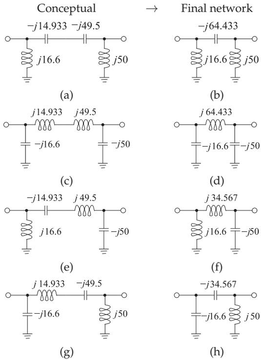
**Figure 6-24:** Four possible Pi matching networks: (a), (c), (e), and (g) conceptual circuits; and (b), (d), (f), and (h), respectively, their final reduced Pi networks.
