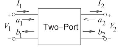
**Figure 2-25:** Two-port with parameters suitable for defining  $S$  and  $ABCD$  parameters.
