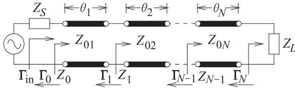
**Figure 7-9:** Stepped-impedance transmission line transformer with the  $n$ th section having characteristic impedance  $Z_{0n}$  and electrical length  $\theta_n$ .  $\Gamma_n$  is the reflection coefficient, and  $Z_n$  the impedance, considering only the  $(n + 1)$ th line.
