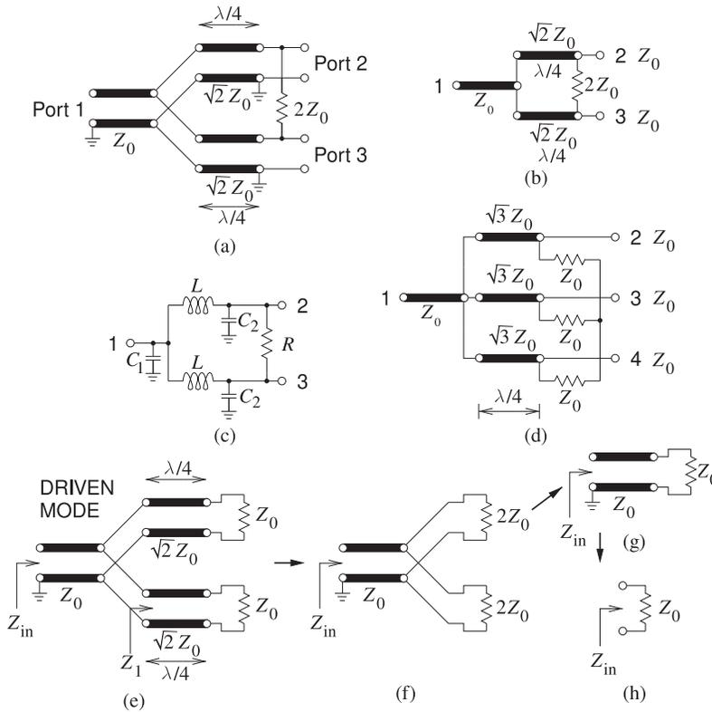
**Figure 5-27:** Wilkinson divider: (a) two-way divider with Port 1 being the combined signal and Ports 2 and 3 being the divided signals; (b) less cluttered representation; (c) lumped-element implementation; (d) three-way divider with Port 1 being the combined signal and Ports 2, 3, and 4 being the divided signals; and (e)–(h) steps in the derivation of the input impedance.
