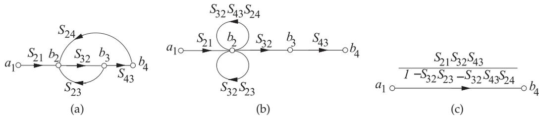
Figure 3-9: Signal flow graph with multiple loops.
