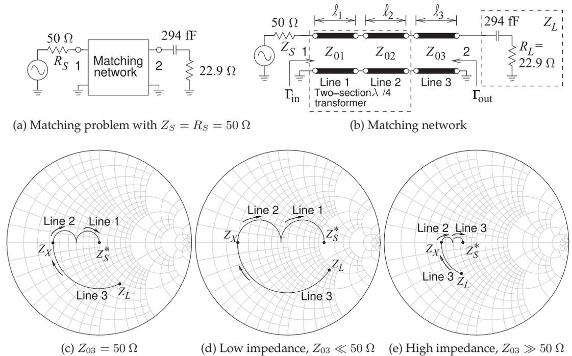
**Figure 7-18:** Matching problem of the case study of Section 7.6 using a two-section cascaded quarter-wave impedance transformer. The arrows in (c), (d), and (e) indicate increasing line length at 10 GHz. The Smith charts are normalized to  $Z_{03}$  and present three design concepts. (The choice of high  $Z_{03}$  is appropriate for  $R_L < Z_S$  and a capacitor in the load.)
