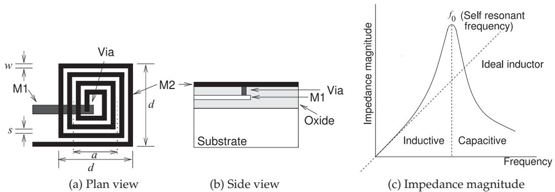
Figure 5-5: An on-chip spiral inductor.
