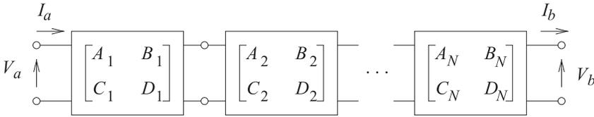
**Figure 2-10:** Cascade of two-port networks.
