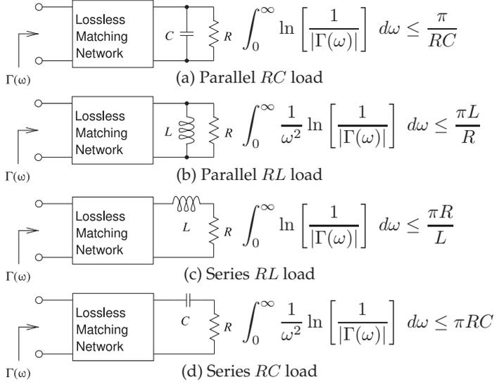
**Figure 7-1:** Fano-Bode limits for circuits with reactive loads.
