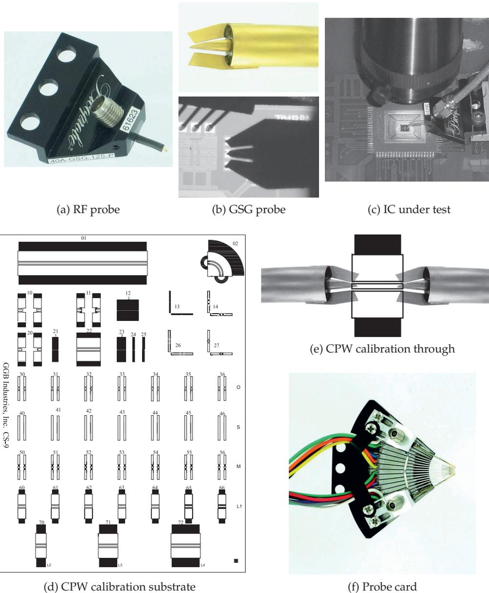
**Figure 4-5:** RF probes: (a) single RF probe probe; (b) detail of a GSG probe and contacting an IC; (c) an IC under test; (d) layout of a calibration substrate used with GSG probes; (e) probes contacting a through CPW structure on the calibration substrate; and (f) a probe card with 2 RF probes (top and bottom) and 13 needle probes for DC and low-frequency connections. ((a), (b) top, (d), (e), (f) Copyright GGB Industries Inc., used with permission [2].)
