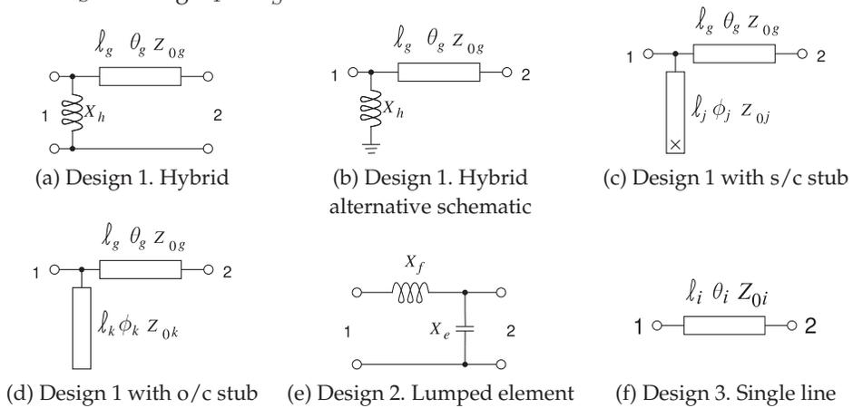
**Figure 6-45:** Matching network topologies using lumped elements and microstrip lines. In the stub layouts x is a via to the ground plane implementing a short circuit (s/c) and an open circuit o/c simply does not show a connection to the microstrip ground plane.
