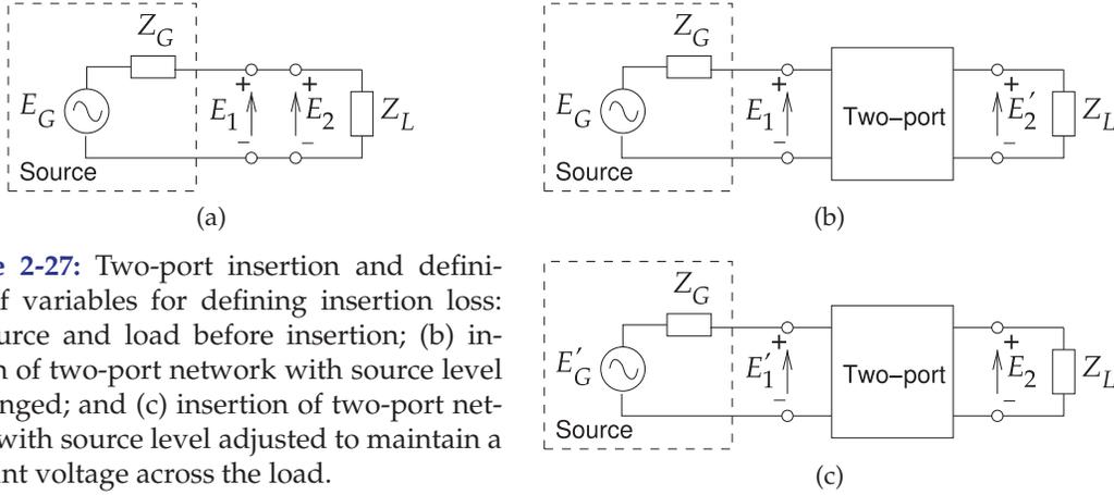
**Figure 2-27:** Two-port insertion and definition of variables for defining insertion loss: (a) source and load before insertion; (b) insertion of two-port network with source level unchanged; and (c) insertion of two-port network with source level adjusted to maintain a constant voltage across the load.
