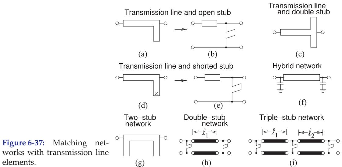
**Figure 6-37:** Matching networks with transmission line elements.
