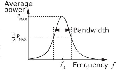
**Figure 5-2:** Second-order resonant circuits.
