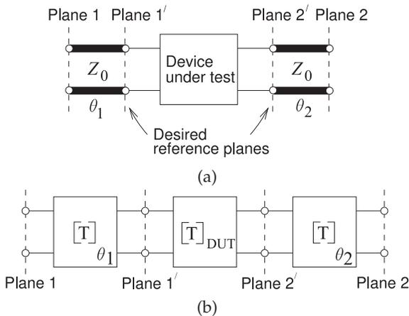
**Figure 2-24:** Two-port measurement setup: (a) a two-port comprising a device under test (DUT) and transmission line sections that create a reference plane at Planes 1 and 2; and (b) representation as cascaded two-port networks.
