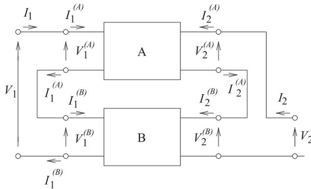
Figure 2-5: Series connection of two two-port networks.
