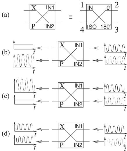
**Figure 5-21:** A 180° hybrid as a combiner (with output at the sum port,  $\Sigma$ ) and as a comparator (with output at the difference port,  $\Delta$ ): (a) equivalence between a 180° hybrid and a sum-and-difference hybrid; (b) the two inputs are in phase; (c) the two inputs are 180° out of phase; and (d) the two inputs are 90° out of phase.
