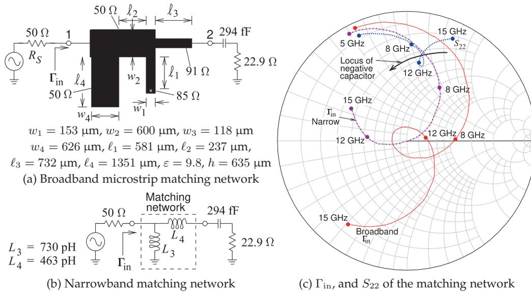
**Figure 7-23:** Broadband and narrowband matching networks with  $\Gamma_{in}$  of both networks and  $S_{22}$  of the broadband network shown with the the locus of the ideal conjugate match (identified as the locus of negative capacitor). In (a)  $\ell_1 = 0.048 \lambda, \ell_2 = 0.020 \lambda, \ell_3 = 0.060 \lambda,$  and  $\ell_4 = 0.117 \lambda$  at 10 GHz. In (b) a 50  $\Omega$  Smith chart is used.
