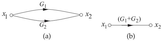
**Figure 3-3:** Signal flow graph representation of addition.
