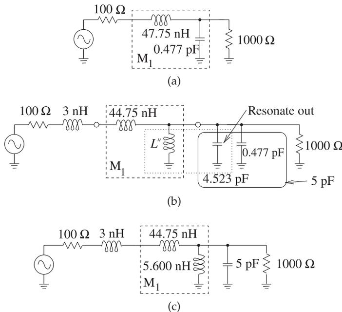
**Figure 6-17:** Evolution of the matching network in Example 6.6: (a) matching network design considering only the source and load resistors; (b) matching network with the reactive parts of the source and load impedances included; and (c) final design.
