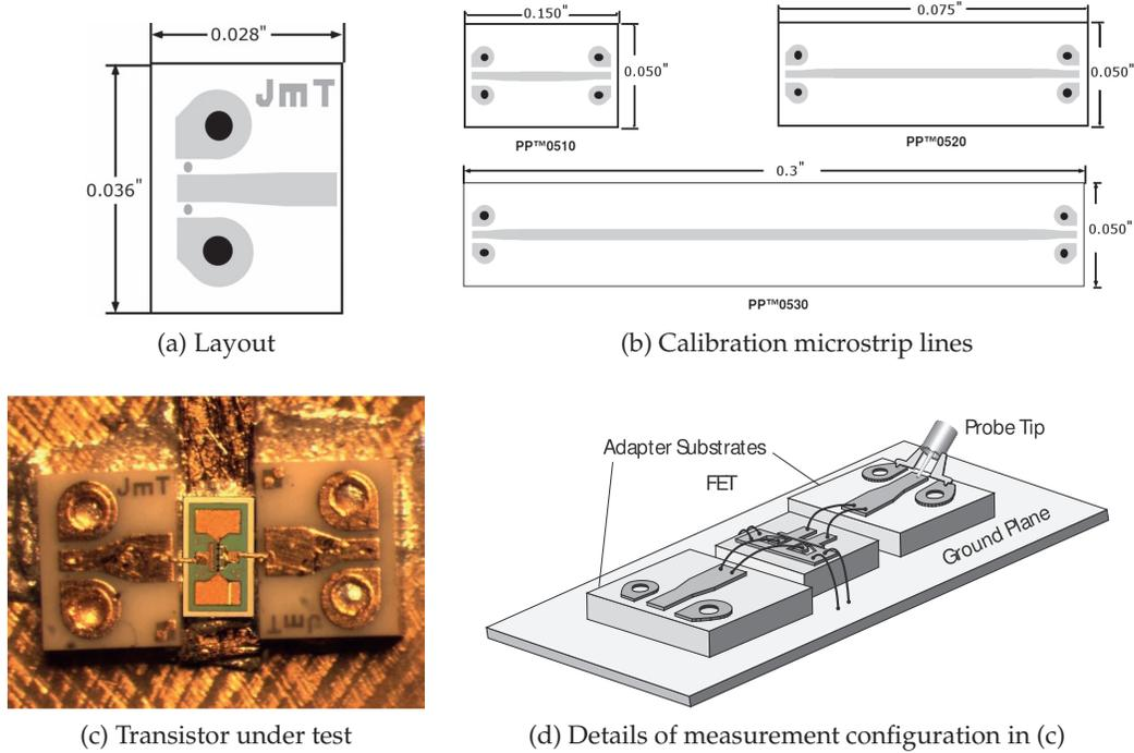
**Figure 4-6:** Use of a CPW-to-microstrip adaptor enabling coplanar probes to be used in characterizing a non-CPW device. The adaptors provide a low insertion loss CPW-to-microstrip transition. Used with permission of J microTechnology, Inc.
