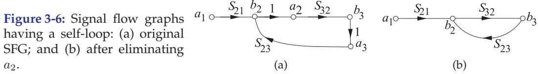
**Figure 3-7:** Signal flow graph of (a) a self-loop; and (b) with the loop eliminated.
