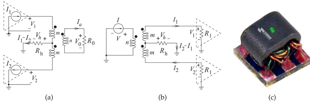
**Figure 5-36:** A  $180^\circ$  hybrid transformer: (a) used as a combiner; (b) used as a splitter; and (c) center-tapped transformer as a surface-mount component (Model TM1-2 with a frequency range of 20–1200 MHz. Copyright Synergy Microwave Corporation, used with permission [34]).
