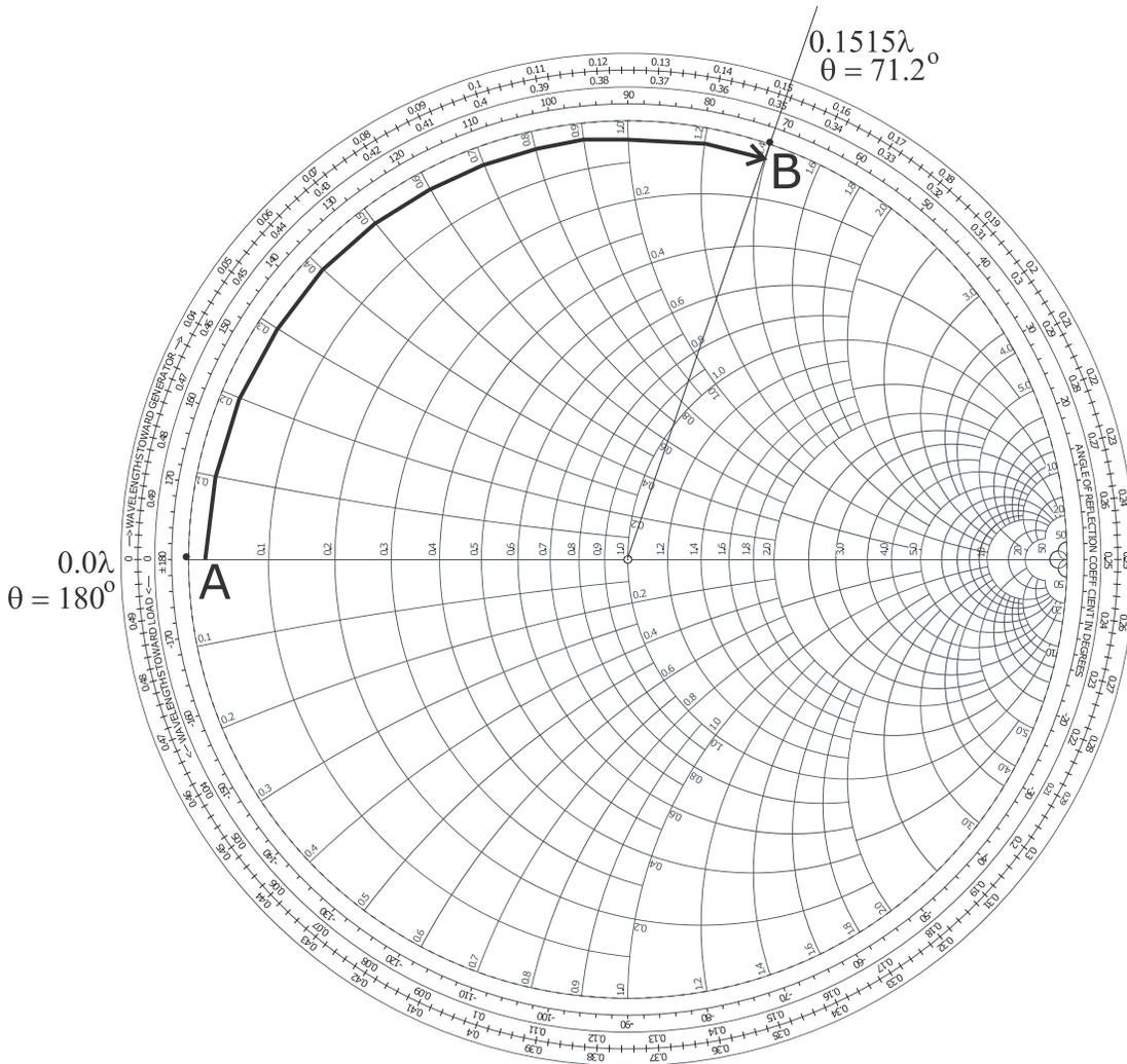
**Figure 3-20:** Design of a short-circuit stub with a normalized input impedance of  $j1.4$ . The path AB is actually on the unit circle but has been displaced here to avoid covering numbers. The electrical length in wavelengths has been read from the outermost circular scale, and the angle,  $\theta$ , in degrees refers to the angle of the polar plot (and is twice the electrical length).
