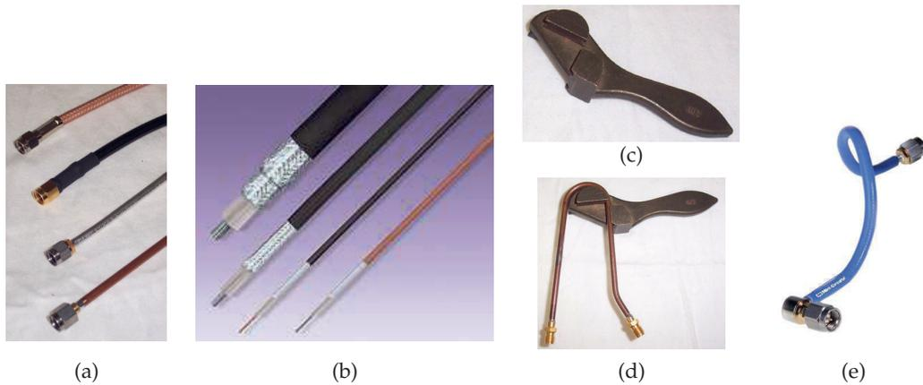
**Figure 2-8:** Coaxial lines: (a) SMA cables (from the top): flexible cable type I, type II, type III, and semirigid cable; (b) coaxial cables showing layers; (c) semirigid coaxial cable bender; (d) bender with line; and (e) hand-formable cable supporting tight radius with low return and insertion loss. ((b) Copyright Megaphase LLC, used with permission [5].) ((e) Copyright 2012 Scientific Components Corporation d/b/a Mini-Circuits, used with permission [4].)
