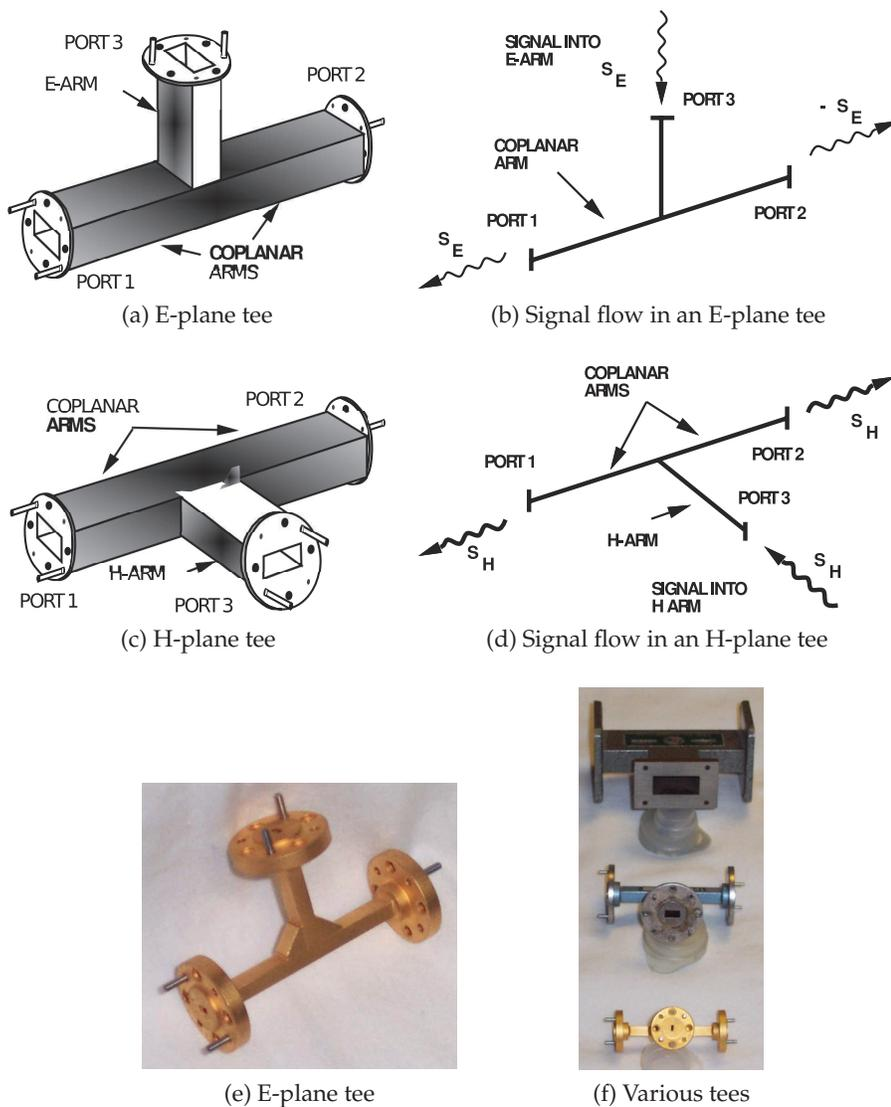
**Figure 6-12:** Rectangular waveguide tees: (a) three-dimensional representation of an E-plane tee; (b) description of the signal flow in an E-plane tee; (c) three-dimensional representation of an H-plane tee; (d) description of the signal flow in an H-plane tee; (e) photograph of an E-plane tee; and (f) photograph of waveguide tees for different waveguide bands (top, X-band H-plane tee; middle, Ku-band H-plane tee; bottom, Ka-band E-plane tee).
