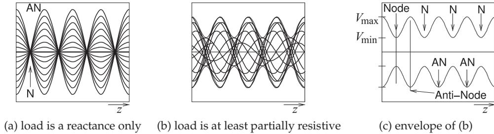
**Figure 2-19:** Standing waves as an overlay of waveforms at many times: (a) when the forward- and backward-traveling waves have the same amplitude; (b) when the waves have different amplitudes; and (c) the envelope of the standing wave. N is a node (a minimum) and AN is an antinode (a maximum). Nodes, N, are separated by  $\lambda/2$ . Antinodes, AN, are separated by  $\lambda/2$ .
