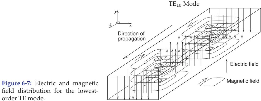
**Figure 6-7:** Electric and magnetic field distribution for the lowest-order TE mode.
