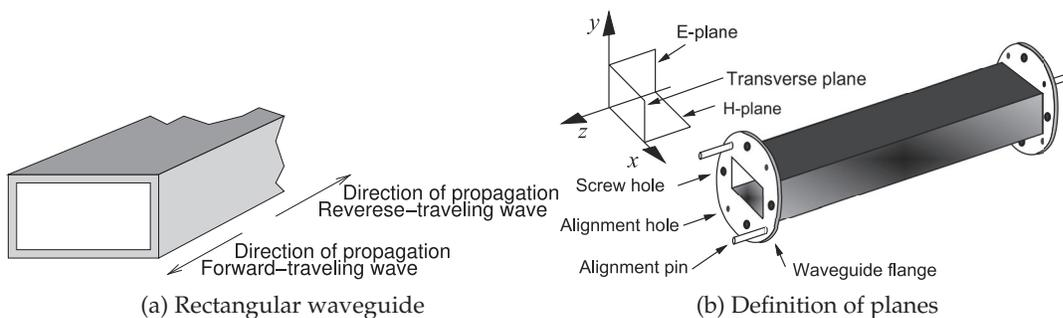
Figure 6-1: Rectangular waveguide.
