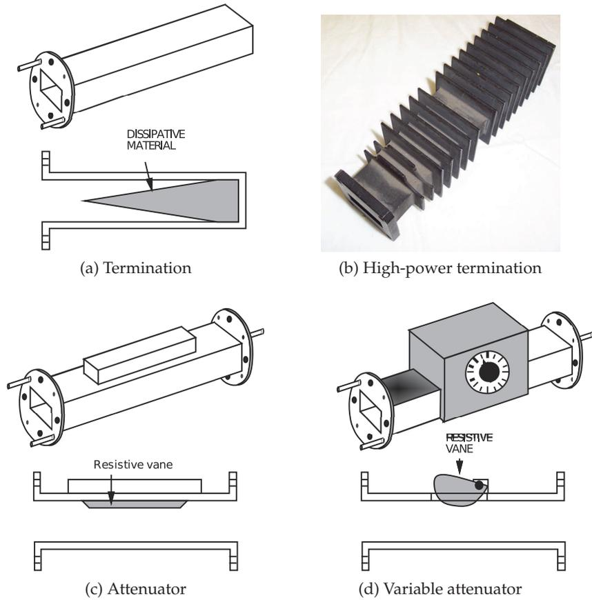
**Figure 6-13:** Terminations and attenuators in a rectangular waveguide.
