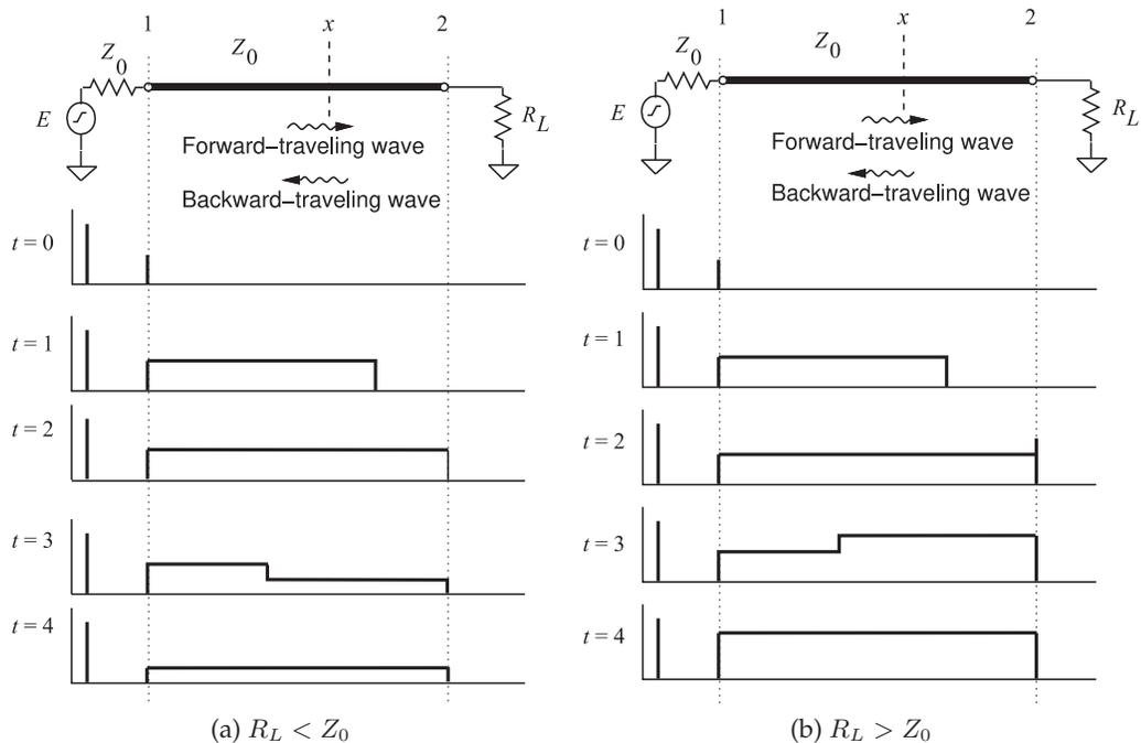
**Figure 2-14:** Reflection of a voltage pulse from a load: (a) when the resistance of the load,  $R_L$  is lower than the characteristic impedance of the line,  $Z_0$ ; and (b) when  $R_L$  is greater than  $Z_0$ .
