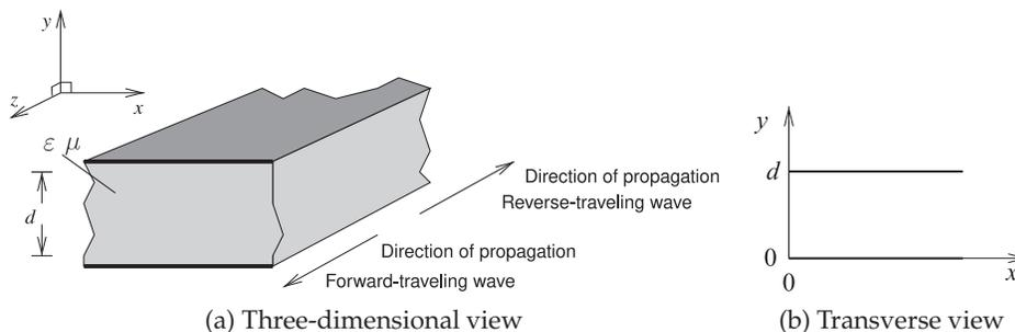
Figure 6-3: Parallel-plate waveguide.
