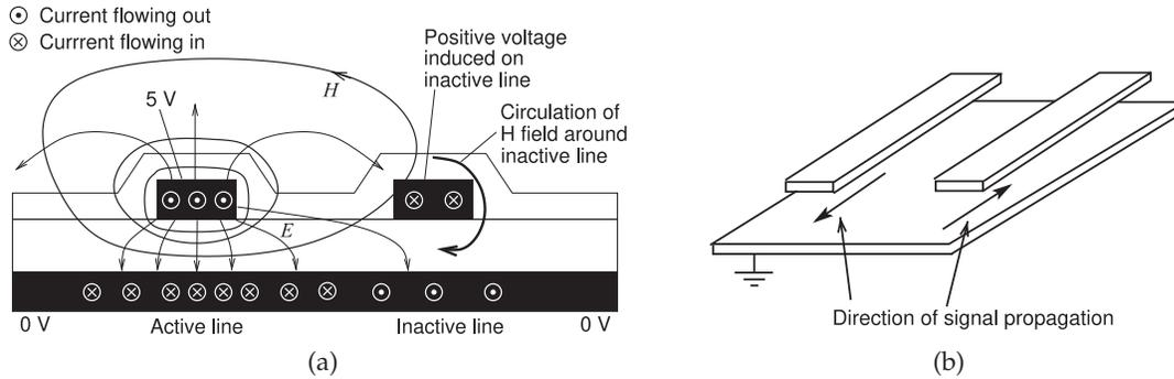
**Figure 5-1:** Edge-coupled microstrip lines with the left line driven with the forward-traveling field coming out of the page: (a) cross section of microstrip lines as found on a printed circuit board showing a conformal top passivation or solder resist layer; and (b) in perspective showing the direction of propagation of the driven line (left) and the direction of propagation of the main coupled signal on the victim line (right).
