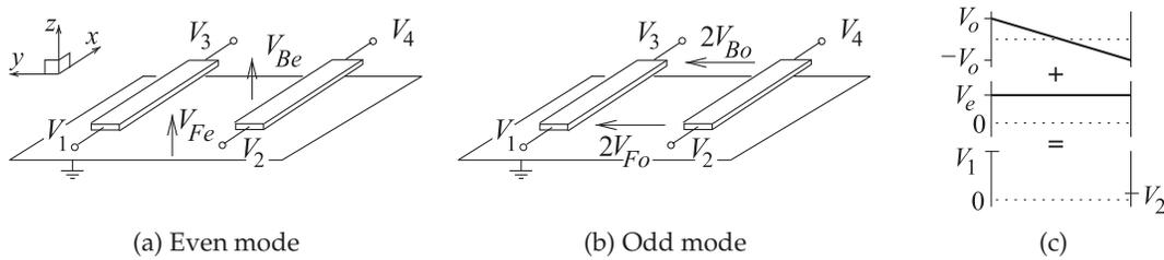
**Figure 5-3:** Definitions of total voltages and even- and odd-mode voltage phasors on a pair of coupled microstrip lines: (a) even-mode voltage definition; (b) odd-mode voltage definition; (c) depiction of how even- and odd-mode voltages combine to yield the total voltages on individual lines. *F* indicates front and *B* indicates back.
