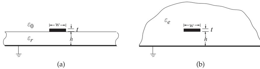
**Figure 3-7:** Microstrip /ink.sh micr (a) cross section; and (b) approximate equivalent structure where the strip is embedded in a dielectric of semi-infinite extent with effective relative permittivity  $\epsilon_e$ .
