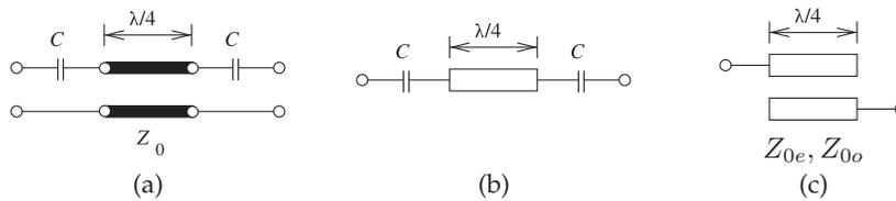
**Figure 5-23:** Coupled line equivalence: (a) a one-quarter wavelength long line with input and output series capacitance; (b) microstrip layout; and (c) equivalent coupled lines laid out in microstrip. The network in (a) is equivalent to the network in (c) if  $Z_{0e} = (1/C + 2Z_0)$  and  $Z_{0o} = Z_0$ .
