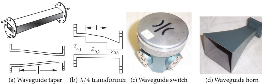
**Figure 6-16:** Waveguide components: (a) waveguide switch; (b) rectangular waveguide quarter-wavelength impedance transformer; (c) rectangular waveguide taper connecting one waveguide series to another; and (d) waveguide horn antenna.
