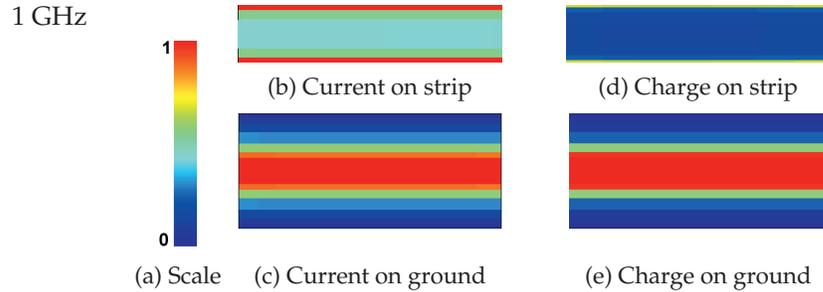
**Figure 4-5:** Normalized current and charge magnitudes on an alumina microstrip line at 1 GHz ( $\epsilon_r = 10.0$ ): (a) scale; (b) longitudinal current,  $i_z$ , on the strip (10–26 A/m); (c) on the ground plane (0–3.2 A/m); (d) charge on the strip (80–400 nC/m<sup>2</sup>); and (e) on the ground (0–33 nC/m<sup>2</sup>). See inside the back cover for a color image.
