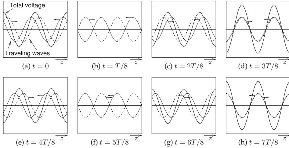
**Figure 2-18:** Evolution of a standing wave with a reactive load as the sum of forward- and backward-traveling waves (to the right and left, respectively) of equal amplitude evaluated at times  $t$  equal to eighths of the period  $T$ . At  $t = T/8$  and  $t = 5T/8$  the total voltage everywhere on the line is zero.
