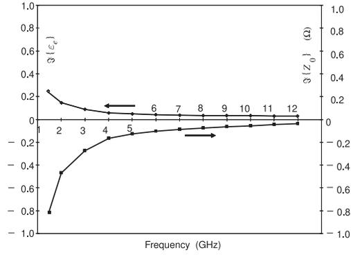
(a)  $w = 240 \mu\text{m}$ ,  $h = 500 \mu\text{m}$
