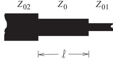
**Figure 2-26:** Layout of a microstrip quarter-wave transformer.
