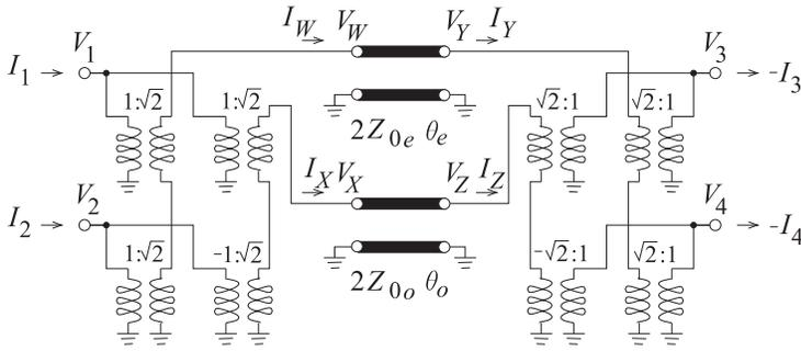
**Figure 5-26:** Annotated coupled-line model used in Example 5.4.
