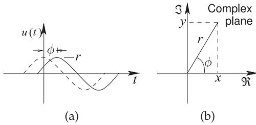
**Figure 1-11:** Sinusoidal signal representations: (a) waveform referenced to the zero-phase cosinusoid shown as the dashed waveform; and (b) representation as a phasor on the complex plane where  $Re$  is the real part and  $Im$  is the imaginary part.
