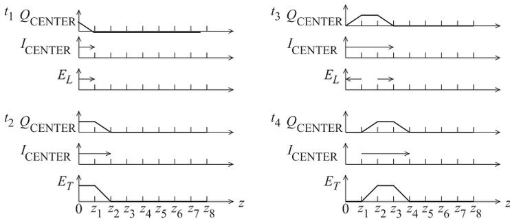
**Figure 2-3:** Fields, currents, and charges on the coaxial transmission line of Figure 2-2 at times  $t_4 > t_3 > t_2 > t_1$ .  $Q_{\text{CENTER}}$  is the net free charge on the center conductor.  $I_{\text{CENTER}}$  is the current on the center conductor.
