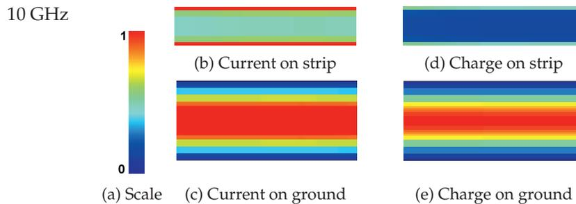
**Figure 4-6:** Normalized current and charge magnitudes on an alumina microstrip line at 10 GHz: (a) scale; (b) longitudinal current,  $i_z$ , on the strip (10–28 A/m); (c) on the ground plane (0–4.1 A/m); (d) charge on the strip (114–512 nC/m<sup>2</sup>); and (e) on the ground (0–39 nC/m<sup>2</sup>). See inside the back cover for a color image.
