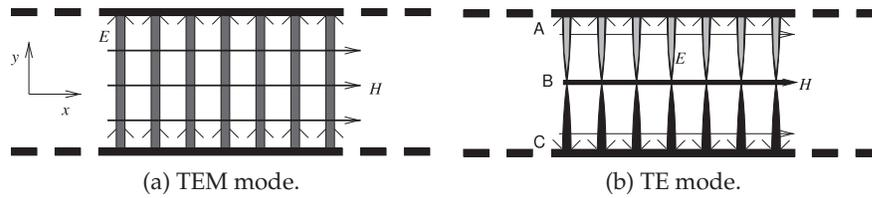
**Figure 4-14:** Parallel-plate waveguide showing electric,  $E$ , and magnetic,  $H$ , field lines. The electric ( $E$ ) and magnetic ( $H$ ) field lines are shown with the line thickness indicating field strength. The shading of the  $E$  field lines indicates polarity (+ or -) and the arrows indicate direction (and also polarity). The  $z$  direction is into the page.
