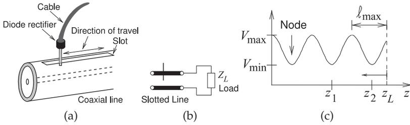
**Figure 2-20:** Measurement of standing waves: (a) coaxial slotted line; (b) schematic of slotted line; (c) measured standing wave.
