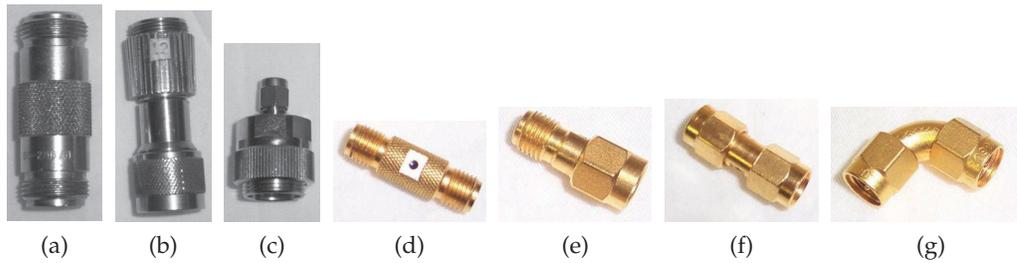
**Figure 2-6:** Coaxial line adaptors: (a) N-type female-to-female (N(f)-to-N(f)); (b) APC-7 to N-type male (APC-7-to-N(m)); (c) APC-7 to SMA-type male (APC-7-to-SMA(m)); SMA adaptors: (d) SMA-type female-to-female (SMA(f)-to-SMA(f)); (e) SMA-type male-to-female (SMA(m)-to-SMA(f)); (f) SMA-type male-to-male (SMA(m)-to-SMA(m)); and (g) SMA elbow. N, APC-7 and SMA are known as connector series.
