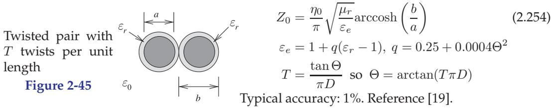
Characteristics of two-conductor transmission lines.
