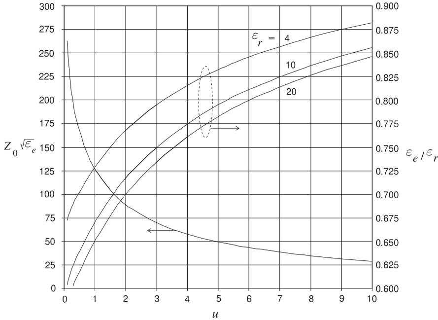
**Figure 5-11:** Normalized characteristic impedance and normalized effective permittivity of a microstrip line as a function of  $u = w/h$ . For example, if  $u = 1$  and  $\epsilon_r = 10$ , then from the figure,  $Z_0\sqrt{\epsilon_e} = 126 \Omega$  and  $\epsilon_e/\epsilon_r = 0.671$ ; thus  $Z_0 = 48.6 \Omega$  and  $\epsilon_e = 6.71$ .
