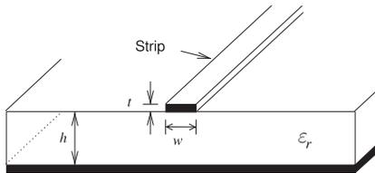
Figure 1-1: Microstrip transmission line.
