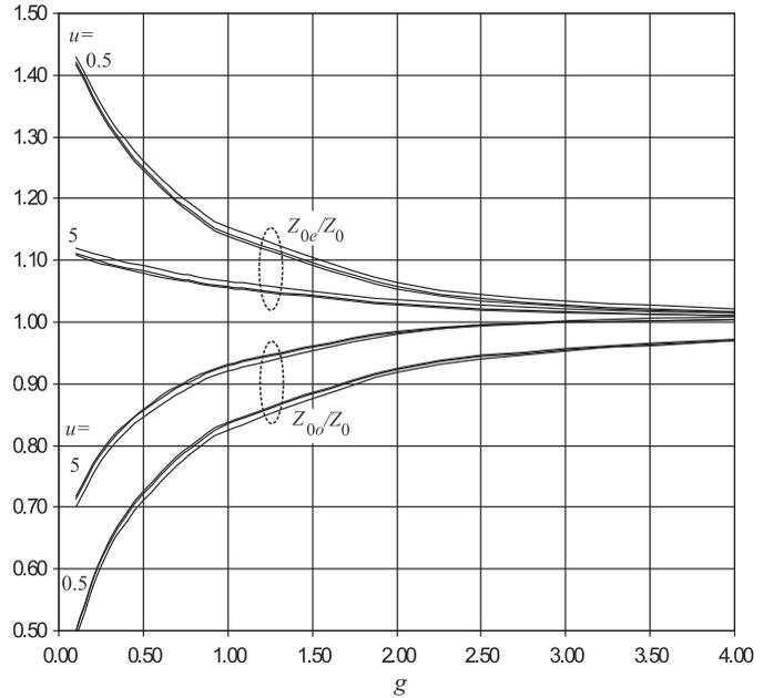
**Figure 5-13:** Normalized even-mode and odd-mode characteristic impedances of a pair of coupled microstrip lines for extremes of  $u$ . Each family of three curves is for  $\epsilon_r = 4, 10,$  and  $20$ .  $Z_0$  is the characteristic impedance of an individual microstrip line with the same normalized width,  $u = w/h$ . The strips have equal width.
