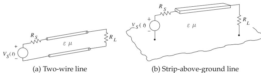
**Figure 2-1:** Two conductor transmission lines.
