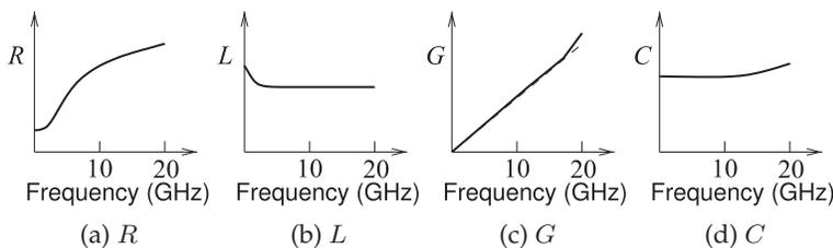
**Figure 4-1:** Frequency dependence of transmission line parameters.
