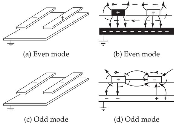
**Figure 5-2:** Modes on parallel-coupled microstrip lines. In (b) and (d) the electric fields are indicated as arrowed lines and the magnetic field lines are dashed.
