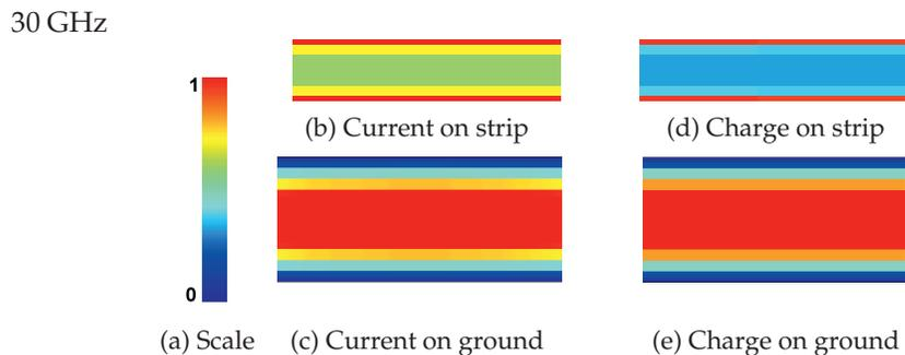
**Figure 4-7:** Normalized magnitudes of current and charge on an alumina microstrip line at 30 GHz: (a) scale; (b) longitudinal current,  $i_z$ , on the strip (10–31 A/m); (c) on the ground plane (0–6 A/m); (d) the charge on the strip (200–575 nC/m<sup>2</sup>); and (e) on the ground (0–68 nC/m<sup>2</sup>). See inside the back cover for a color image.
