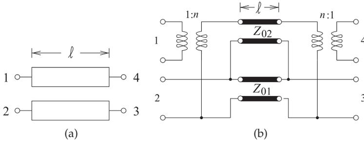
**Figure 5-27:** A pair of symmetrical coupled lines: (a) physical layout; and (b) its approximate equivalent circuit model in a form that appears in network synthesis.  $n = (Z_{0e} + Z_{0o}) / (Z_{0e} - Z_{0o})$ .
