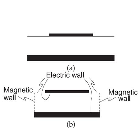
**Figure 4-16:** Approximation of a microstrip line as a waveguide: (a) cross section of microstrip; and (b) **microstrip waveguide model** having effective width  $w + 0.4h$  with magnetic and electric walls.
