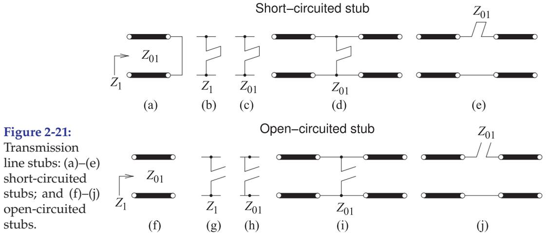
**Figure 2-21:** Transmission line stubs: (a)–(e) short-circuited stubs; and (f)–(j) open-circuited stubs.
