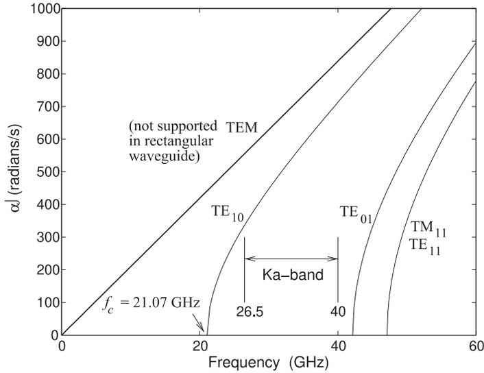
**Figure 6-8:** Dispersion diagram of waveguide modes in air-filled Ka-band rectangular waveguide with internal dimensions of 0.280 × 0.140 inches (7.112 mm × 3.556 mm). Ka-band waveguide is used between 26.5 GHz and 40 GHz. Over this frequency range only the TE<sub>10</sub> mode propagates.
