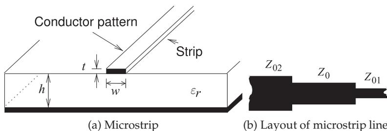
**Figure 2-10:** Microstrip transmission line. The layout (or top) view is commonly used with circuit designs using microstrip. This is the pattern of the strip where (b) shows three lines of different width.
