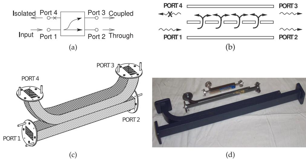
**Figure 6-18:** Rectangular waveguide directional couplers: (a) schematic; (b) and (c) waveguide directional coupler showing coupling slots; and (d) three directional couplers with the fourth port terminated in an integral matched load. In (d), from top to bottom: W-band, 10 cm long; Ka-band, 15 cm long, and X-band, 35 cm long.
