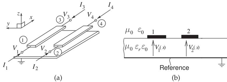
of the two modes will differ since the two modes have different amounts of energy in the air and in the dielectric, resulting in different effective permittivities of the two modes.
