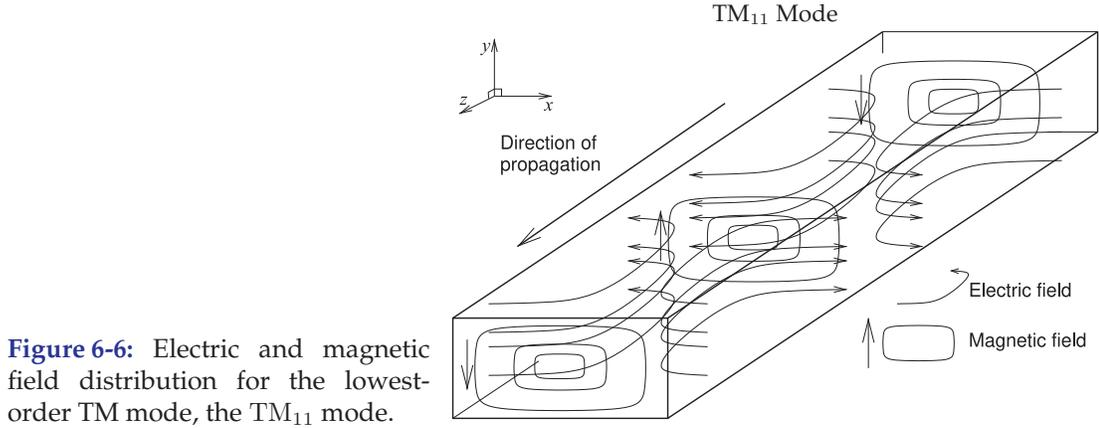
**Figure 6-6:** Electric and magnetic field distribution for the lowest-order TM mode, the  $TM_{11}$  mode.
