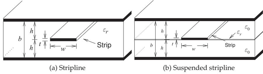
**Figure 3-13:** Fringe capacitance at the corners of the strip in a stripline transmission lines.
