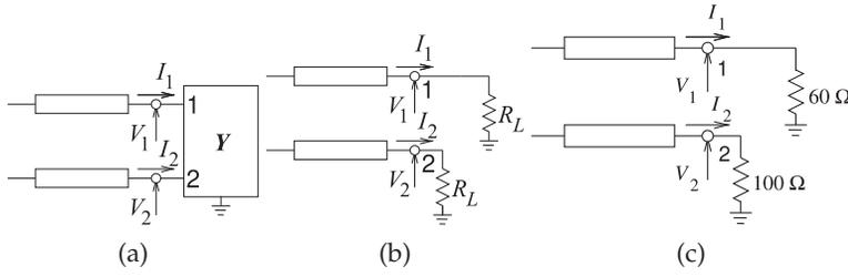
**Figure 5-14:** Terminated coupled lines: (a) with a load described by the y-parameter matrix  $\mathbf{Y}$ ; (b) symmetrical loads; (c) loads considered in example.
