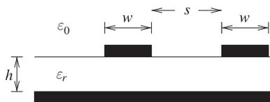
**Figure 5-9:** Cross section of symmetrically coupled microstrip lines.
