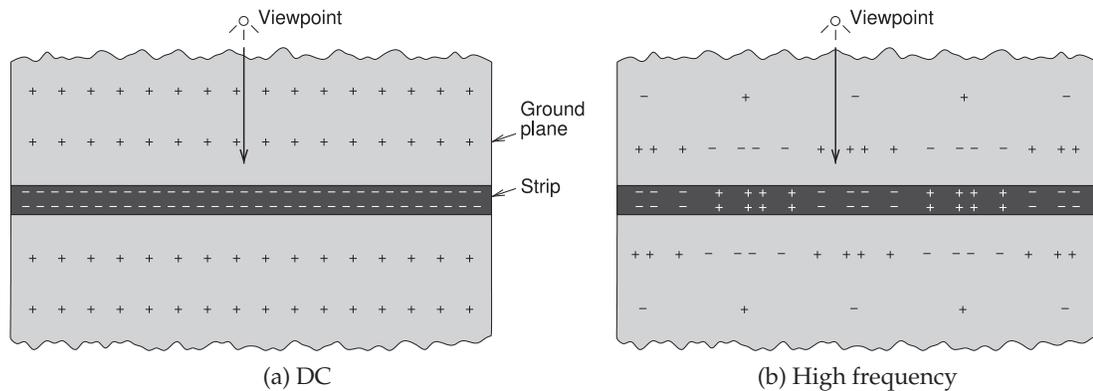
**Figure 4-4:** Current bunching effect in time. Positive and negative charges are shown on the strip and on the ground plane. The viewpoint is on the ground plane.
