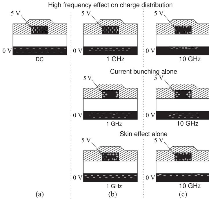
**Figure 4-3:** Cross-sectional view of the charge distribution on an interconnect at different frequencies. The + and - indicate charge concentrations of different polarity and corresponding current densities. There is no current bunching or skin effect at DC.
