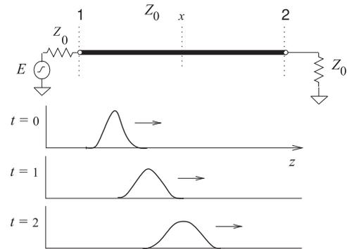
**Figure 4-2:** Dispersion of a pulse along a line.
