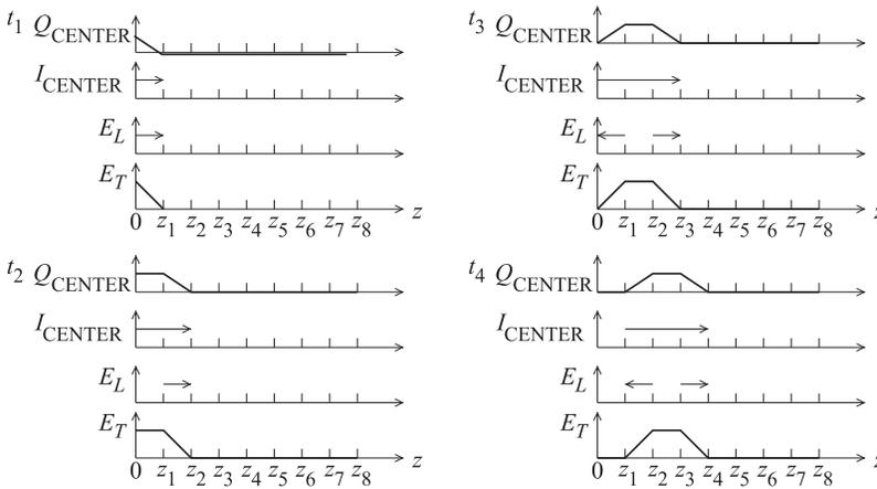
**Figure 2-48:** Fields, currents, and charges on the coaxial transmission line of Figure 2-2 at times  $t_4 > t_3 > t_2 > t_1$ .  $Q_{\text{CENTER}}$  is the net free charge on the center conductor.  $I_{\text{CENTER}}$  is the current on the center conductor.
