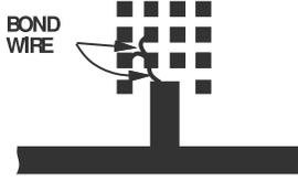
**Figure 2-22:** Open-circuited stub with variable length realized using wire bonding from the fixed stub to one of the bond pads. The bond pads are on the same layer as the strip metal layer and bonding to them extends the length of the open-circuited stub.
