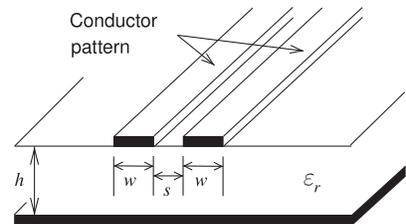
Figure 3-16: Differential line or coplanar strips (CPS).
