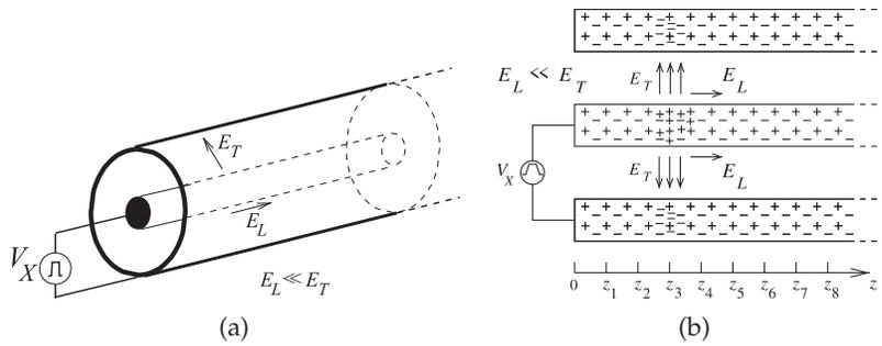
**Figure 2-2:** A coaxial transmission line: (a) three-dimensional view; (b) the line with pulsed voltage source showing the electric fields at an instant in time as a voltage pulse travels down the line.  $E_L \ll E_T$ .
