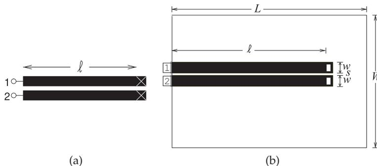
**Figure 5-30:** Coupled microstrip line layout: (a) schematic; and (b) layout in an EM field solver. Dimensions of the coupled lines are  $w = 500 \mu\text{m}$ ,  $s = 100 \mu\text{m}$ ,  $l = 1 \text{ cm}$ ,  $W = 6 \text{ mm}$ ,  $L = 12 \text{ mm}$ . The metal is  $6 \mu\text{m}$  thick gold (conductivity  $\sigma = 42.6 \times 10^6$ ) and the alumina substrate height is  $600 \mu\text{m}$  with relative permittivity  $\epsilon_r = 9.8$  and a loss tangent of 0.001.
