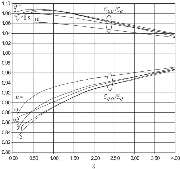
**Figure 5-12:** Normalized even-mode and odd-mode effective permittivity of a pair of coupled microstrip lines. The effective permittivity of an individual microstrip line with the same normalized width  $u$  is  $\epsilon_e$ .
