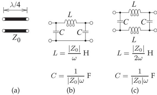
**Figure 2-37:** Lumped equivalent circuit of a one-quarter wavelength long line of characteristic impedance  $Z_0$  which is the same as that of an impedance inverter (of  $Z_0 \Omega$ ): (a) one-quarter wavelength long line segment; (b) lumped-element equivalent circuit; and (c) alternative lumped-element model.
