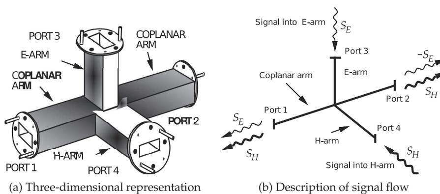
**Figure 6-20:** Rectangular waveguide hybrid.
