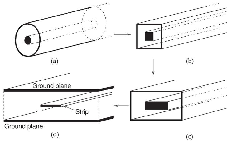
**Figure 1-2:** Evolution of the stripline transmission line: (a) coaxial line with a round center conductor; (b) square coaxial line with a square flat center conductor; (c) rectangular coaxial line with a flat center conductor; and (d) stripline.
