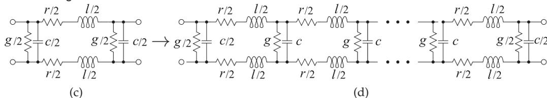
**Figure 2-35:** Lumped-element transmission line models: (a) model of a short segment (e.g.  $\lambda/20$  long); (b) complete model of a transmission line; (c) more accurate model of a segment ; and (d) complete accurate model of a transmission line.
