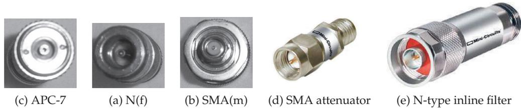
**Figure 2-7:** Various coaxial  $50\ \Omega$  transmission line connectors: (a) APC-7 coaxial connector (7 mm outer conductor diameter); (b) female N-type (N(f)) coaxial connector (7 mm); (c) male SMA-type (SMA(m)) coaxial connector (3.5 mm); (d) DC to 26 GHz, 2-W SMA precision fixed attenuator; and (e) N-type inline 500 MHz lowpass filter. ((d) and (e) copyright 2012 Scientific Components Corporation d/b/a Mini-Circuits, used with permission [4]).
