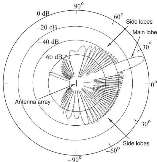
**Figure 2-20:** Electric field pattern from a 30 element array of antennas spaced  $0.65\lambda$  apart. The sidelobe levels are about 40 dB below the power level of the main lobe. The same signal is presented to the antenna elements except that phases of the signal at each antennas is adjusted to produce a main beam directed at 20 degrees. The signals to each antenna are thus correlated. After [13].
