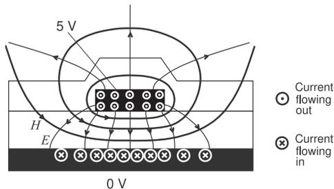
**Figure 4-2:** Cross-sectional view of a microstrip line showing electric and magnetic field lines and current flow. The electric and magnetic fields are in two mediums—the dielectric and air. If the line is homogeneous (the same dielectric everywhere) the electric and magnetic fields are only in the transverse plane, a field configuration known as the transverse electromagnetic mode (TEM).
