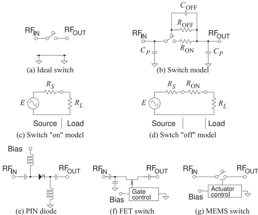
**Figure 11-12:** Microwave switches: (a) ideal switch connecting  $RF_{IN}$  and  $RF_{OUT}$  ports; (b) model of a microwave switch; (c) ideal circuit model with switch on and with source and load; (d) realistic low-frequency circuit model with switch on; (e) switch realized using a PIN diode; (f) switch realized using an FET; and (g) switch realized using a MEMS switch.
