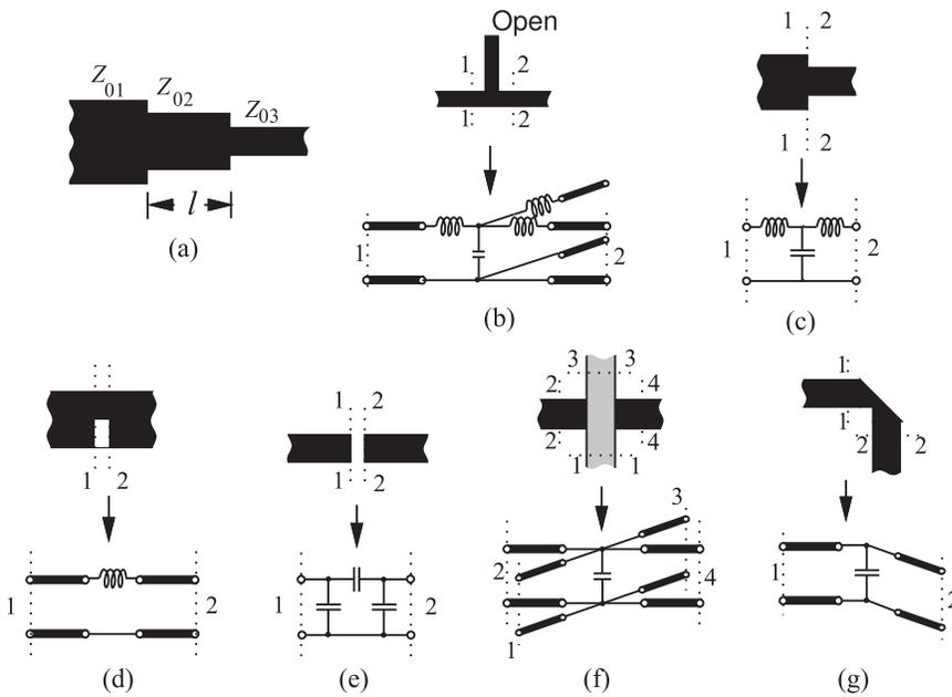
**Figure 9-12:** Microstrip discontinuities: (a) quarter-wave impedance transformer; (b) open microstrip stub; (c) step; (d) notch; (e) gap; (f) crossover; and (g) bend.
