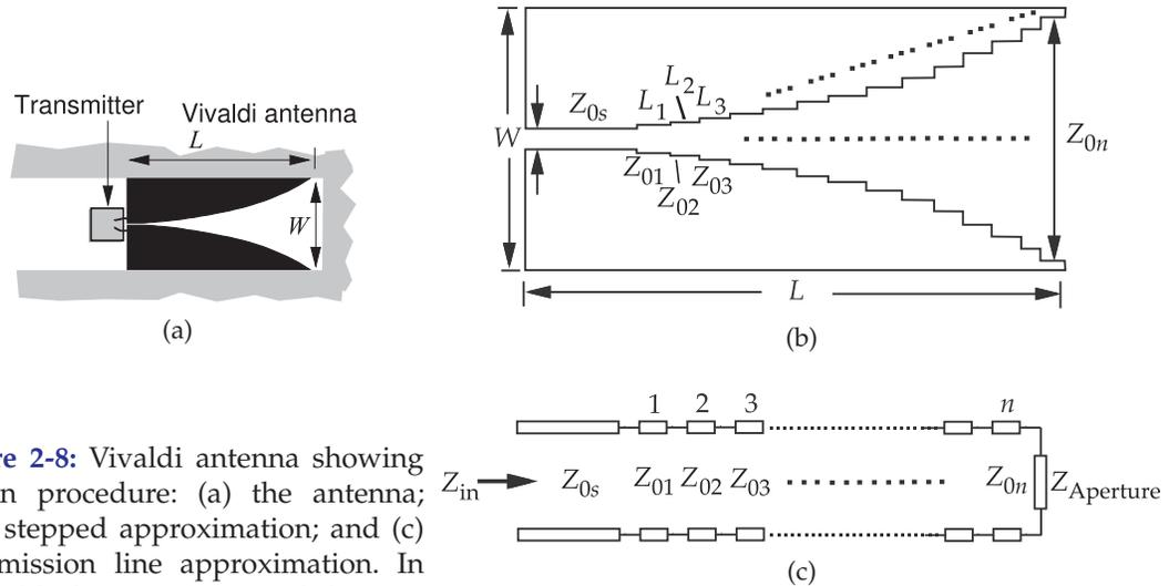
**Figure 2-8:** Vivaldi antenna showing design procedure: (a) the antenna; (b) a stepped approximation; and (c) transmission line approximation. In (a) the black region is a metal sheet.
