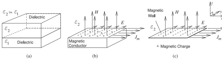
**Figure 5-7:** Properties of the EM field at a magnetic wall: (a) the interface of two dielectrics of contrasting permittivities approximates a magnetic wall; (b) the dielectric with lower permittivity can be approximated as a magnetic conductor; and (c) a magnetic wall.
