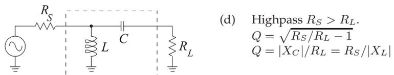
**Figure 10-7:**  $L$  matching networks consisting of one shunt reactive element and one series reactive element. ( $R_S$  is matched to  $R_L$ .)  $X_C$  is the reactance of the capacitor  $C$ , and  $X_L$  is the reactance of the inductor  $L$ . Note that with a two-element matching network the  $Q$  and thus bandwidth of the match is fixed.
