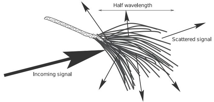
**Figure 2-14:** Pine needles scattering an incoming EM signal.
