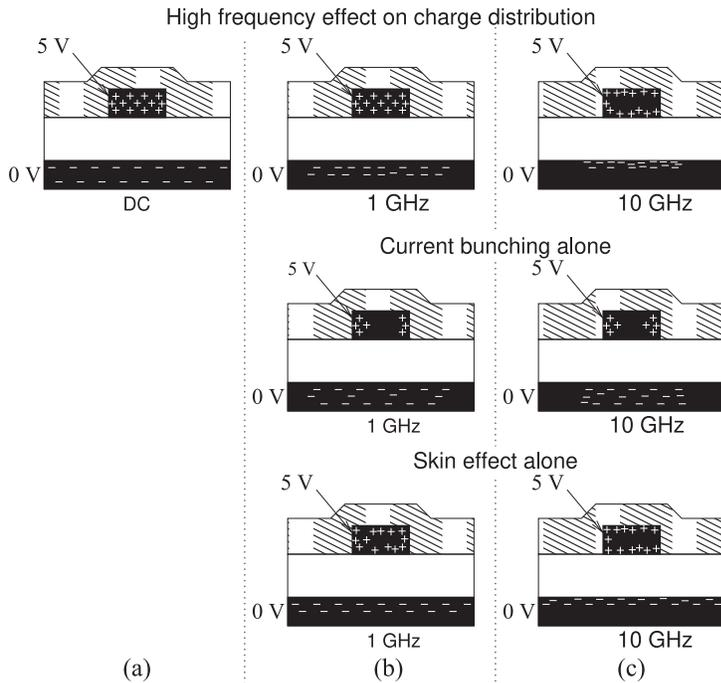
**Figure 5-3:** Cross-sectional view of the charge distribution on an interconnect at different frequencies. The + and - indicate charge concentrations of different polarity and corresponding current densities. There is no current bunching or skin effect at DC.
