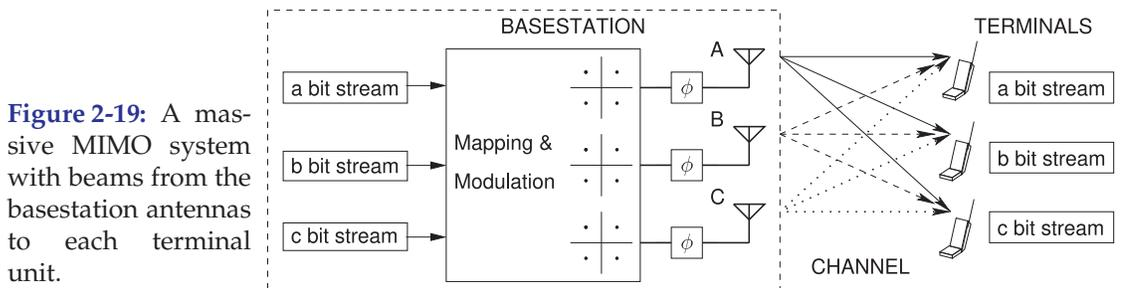
**Figure 2-19:** A massive MIMO system with beams from the basestation antennas to each terminal unit.
