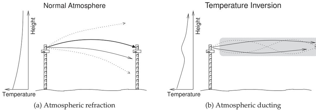
**Figure 2-15:** Fading resulting from ducting: (a) normal atmospheric refraction (normally the temperature of air drops with increasing height and the lower refractive index at high heights results in a concave refraction); and (b) atmospheric ducting (resulting from temperature inversion inducing an air layer with higher dielectric constant than the surrounding air).
