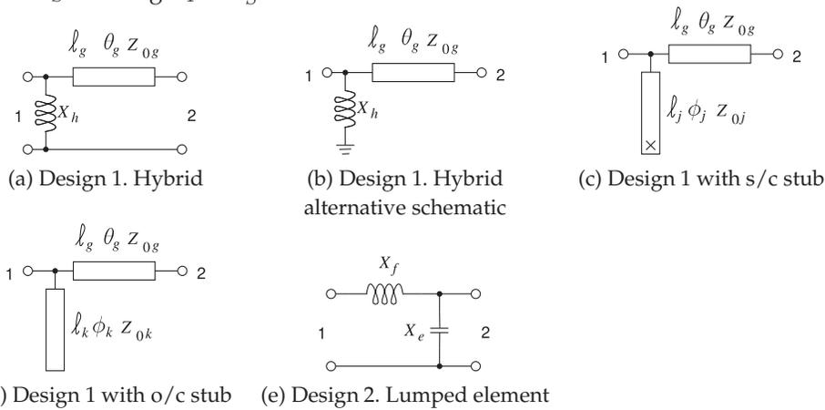
**Figure 10-45:** Matching network topologies using lumped elements and microstrip lines. In the stub layouts x is a via to the ground plane implementing a short circuit (s/c) and an open circuit (o/c) simply does not show a connection to the microstrip ground plane.
