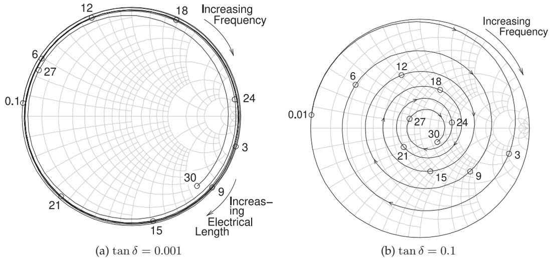
**Figure 8-18:** Smith chart plot of the reflection coefficient of the shorted 1 cm-long microstrip line in Figure 8-17: (a) a low-loss substrate with  $\tan \delta = 0.001$ ; and (b) a high-loss substrate with  $\tan \delta = 0.1$ . Frequencies are marked in gigahertz.
