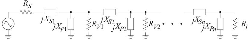
**Figure 10-29:** Cascaded L networks for broadband matching.
