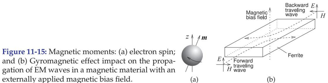
**Figure 11-15:** Magnetic moments: (a) electron spin; and (b) Gyromagnetic effect impact on the propagation of EM waves in a magnetic material with an externally applied magnetic bias field.
