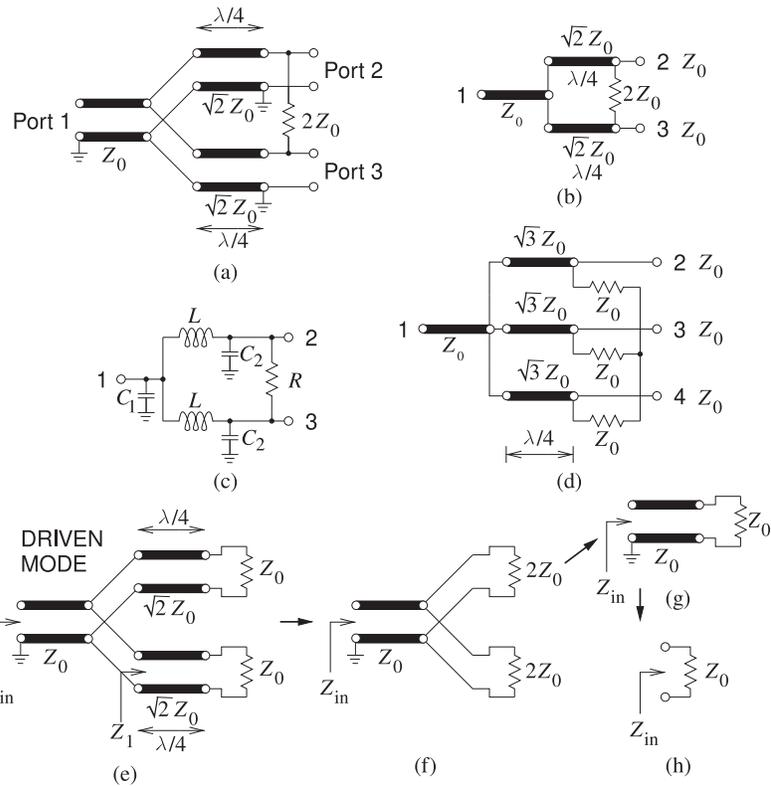
**Figure 9-18:** Wilkinson divider: (a) two-way divider with Port 1 being the combined signal and Ports 2 and 3 being the divided signals; (b) less cluttered representation; (c) lumped-element implementation; (d) three-way divider with Port 1 being the combined signal and Ports 2, 3, and 4 being the divided signals; and (e)–(h) steps in the derivation of the input impedance.
