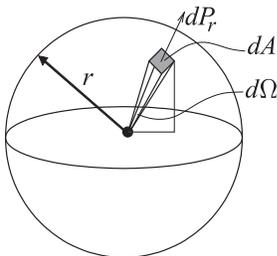
**Figure 2-9:** Free-space spreading loss. The incremental power,  $dP_r$ , intercepted by the shaded region of incremental area  $dA$  is proportional to  $1/r^2$ . The solid angle subtended by the shaded area is the incremental solid angle  $d\Omega$ . The integral of  $dA$  over the surface of the sphere, i.e. the area of the sphere is  $4\pi r^2$ . The total solid angle subtended by the sphere is the integral of  $d\Omega$  over the sphere and is  $4\pi$  steradians (or  $4\pi$  sr).
