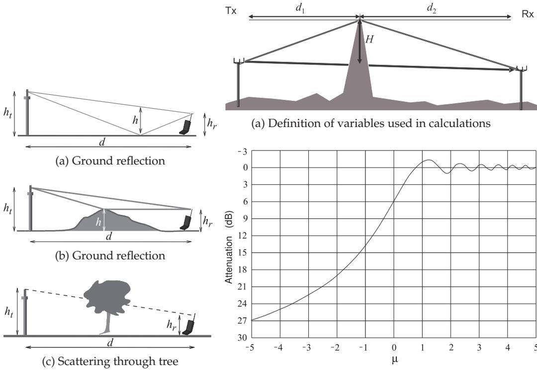
**Figure 2-12:** Common paths contributing to multipath propagation.
