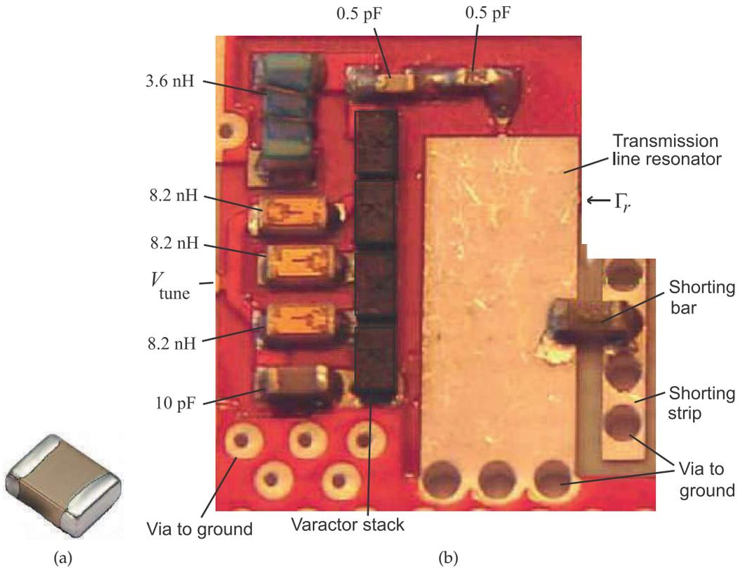
**Figure 9-4:** Circuit board showing the use of surface-mount components: (a) chip resistor or capacitor with metal terminals at the two ends; and (b) a populated RF microstrip circuit board of a 5 GHz tunable resonator [1]. The larger components have dimensions 1.6 mm × 0.8mm. The shorting bar is a 0 Ω chip resistor.
