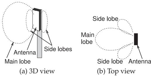
**Figure 2-10:** Field pattern produced by a microstrip antenna.
