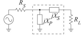
**Figure 10-10:** Two-element matching network topology for  $R_S > R_L$ .
