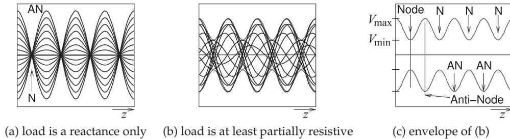
**Figure 3-14:** Standing waves as an overlay of waveforms at many times: (a) when the forward- and backward-traveling waves have the same amplitude; (b) when the waves have different amplitudes; and (c) the envelope of the standing wave. N is a node (a minimum) and AN is an antinode (a maximum). Nodes, N, are separated by  $\lambda/2$ . Antinodes, AN, are separated by  $\lambda/2$ .
