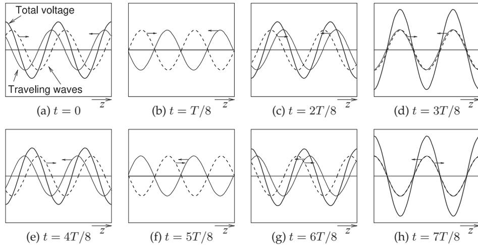
**Figure 3-13:** Evolution of a standing wave as the sum of forward- and backward-traveling waves (to the right and left, respectively) of equal amplitude evaluated at times  $t$  equal to eighths of the period  $T$ . At  $t = T/8$  and  $t = 5T/8$  the total voltage everywhere on the line is zero.
