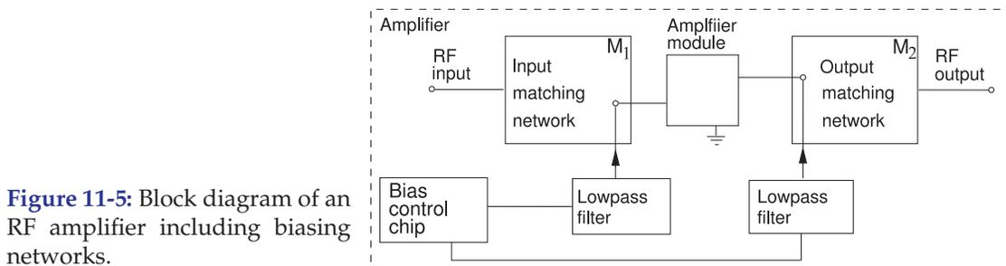
**Figure 11-5:** Block diagram of an RF amplifier including biasing networks.
