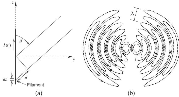
**Figure 2-5:** Monopole antenna showing total current and forward- and backward-traveling currents: (a) a  $\frac{1}{2}\lambda$ -long antenna; and (b) a relatively long antenna.
