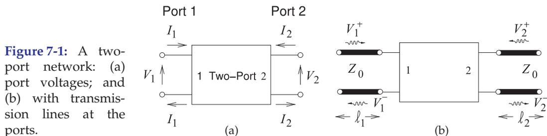
**Figure 7-1:** A two-port network: (a) port voltages; and (b) with transmission lines at the ports.
