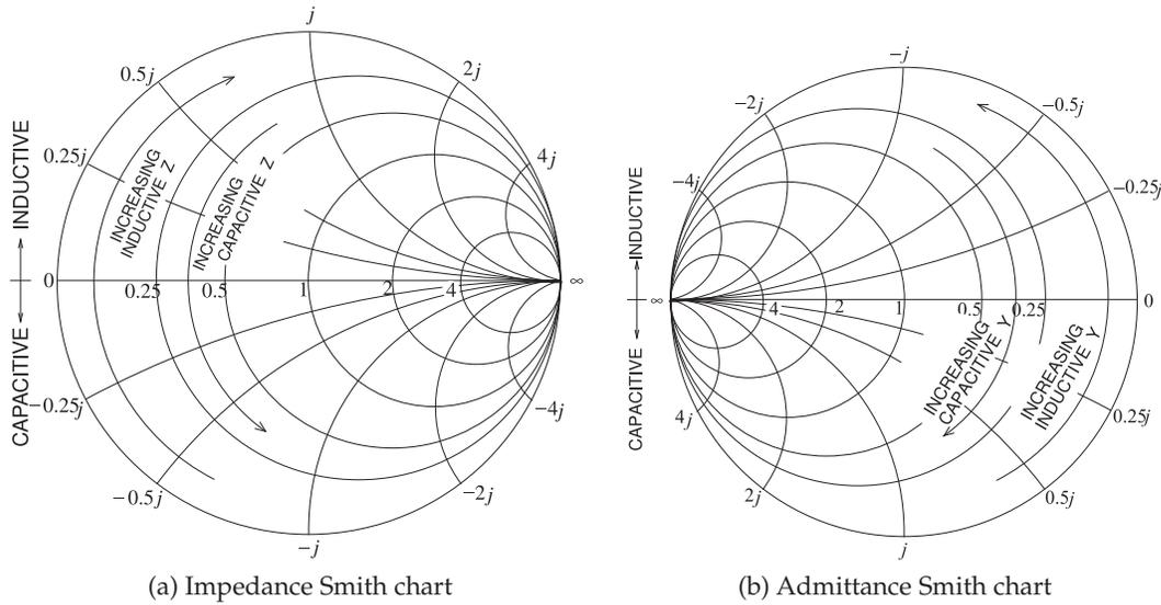
**Figure 10-30:** Inductive and capacitive regions on Smith charts. Increasing capacitive impedance ( $Z$ ) indicates smaller capacitance; increasing inductive admittance ( $Y$ ) indicates smaller inductance.
