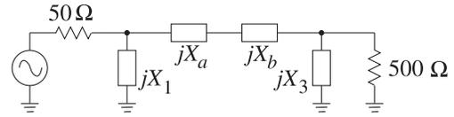
Figure 10-23: Final matching network in Example 10.7.
