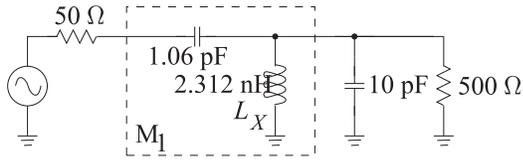
**Figure 10-14:** Final matching network in Example 10.5.
