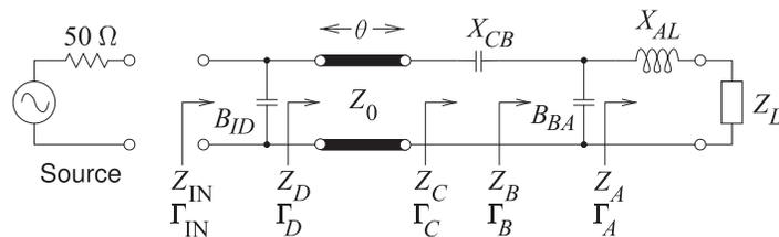
**Figure 8-13:** Circuit used in illustrating Smith chart manipulations.
