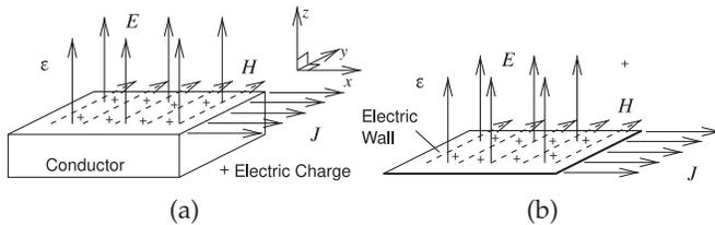
**Figure 5-6:** Properties of an electric wall: (a) the electrical field is perpendicular to a conductor and the magnetic field is parallel to it; and (b) a conductor can be approximated by an electric wall.
