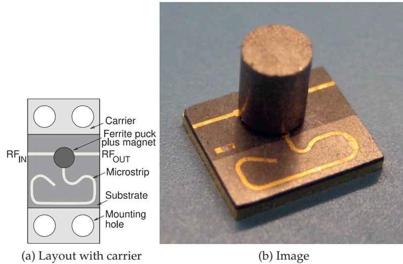
**Figure 11-17:** A microstrip isolator operating from 29 to 31.5 GHz. Isolator in (b) has the dimensions 5 mm × 6 mm and is 6 mm high. The isolator supports 2 W of forward and reverse power with an isolation of 18 dB and insertion loss of 1 dB. Renaissance 2W9 series, copyright Renaissance Electronics Corporation, used with permission.
