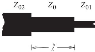
**Figure 3-20:** Layout of a microstrip quarter-wave transformer.
