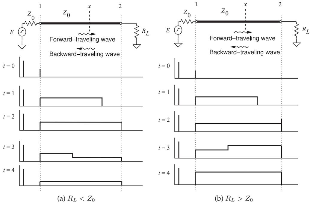
**Figure 3-9:** Reflection of a voltage pulse from a load: (a) when the resistance of the load,  $R_L$  is lower than the characteristic impedance of the line,  $Z_0$ ; and (b) when  $R_L$  is greater than  $Z_0$ .
