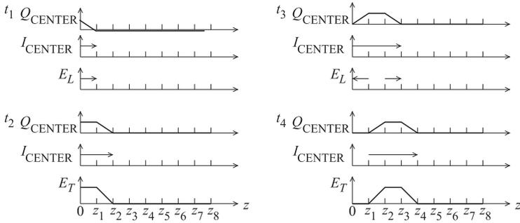
**Figure 3-3:** Fields, currents, and charges on the coaxial transmission line of Figure 3-2 at times  $t_4 > t_3 > t_2 > t_1$ .  $Q_{\text{CENTER}}$  is the net free charge on the center conductor.  $I_{\text{CENTER}}$  is the current on the center conductor.
