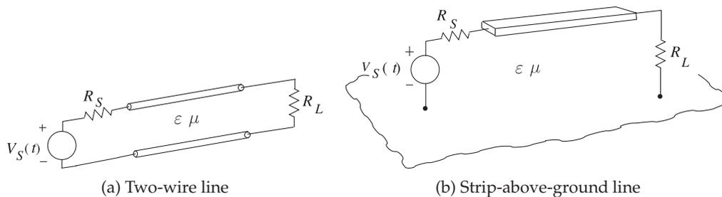
Figure 3-1: Two conductor transmission lines.
