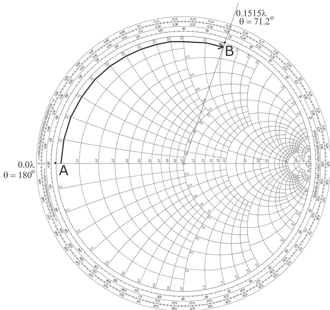
**Figure 8-7:** Design of a short-circuit stub with a normalized input impedance of  $j1.4$ . The path AB is actually on the unit circle but has been displaced here to avoid covering numbers. The electrical length in wavelengths has been read from the outermost circular scale, and the angle,  $\Theta$ , in degrees refers to the angle of the polar plot (and is twice the electrical length).
