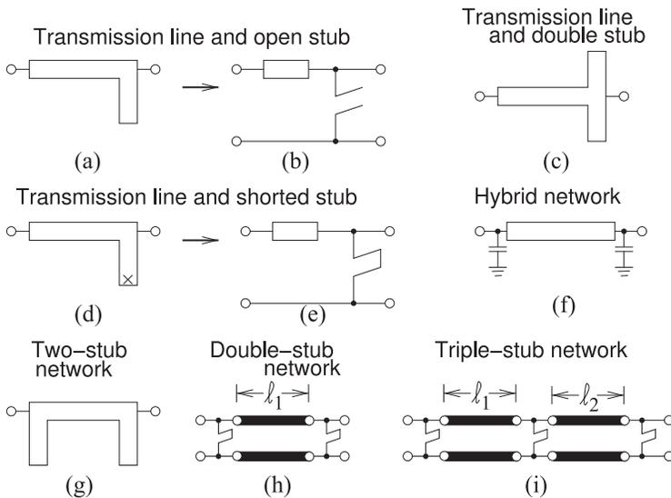
**Figure 10-37:** Matching networks with transmission line elements.
