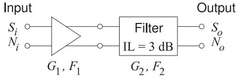
**Figure 11-10:** Differential amplifier followed by a differential filter.
