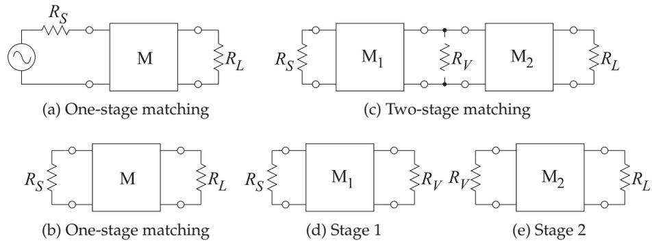
**Figure 10-18:** Matching in stages: (a) matching network  $M$  matching  $R_S$  to  $R_L$ ; (b) without an explicit source; (c) two-stage matching with a virtual resistor  $R_V$ ; (d) matching  $R_S$  to  $R_V$ ; and (e) matching  $R_V$  to  $R_L$ .
