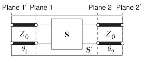
**Figure 8-1:** A two-port with scattering parameter matrix  $S$  augmented by lines at each port with the lines having the reference characteristic impedance  $Z_0$  and electrical length  $\theta_n$ . The scattering parameter matrix of the augmented two-port is  $S'$ .
