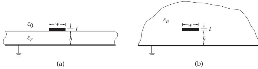
**Figure 4-6:** Microstrip line: (a) cross section; and (b) eps .. equivalent structure where the strip is embedded in a dielectric of semi-infinite extent with effective relative permittivity  $\epsilon_e$ .
