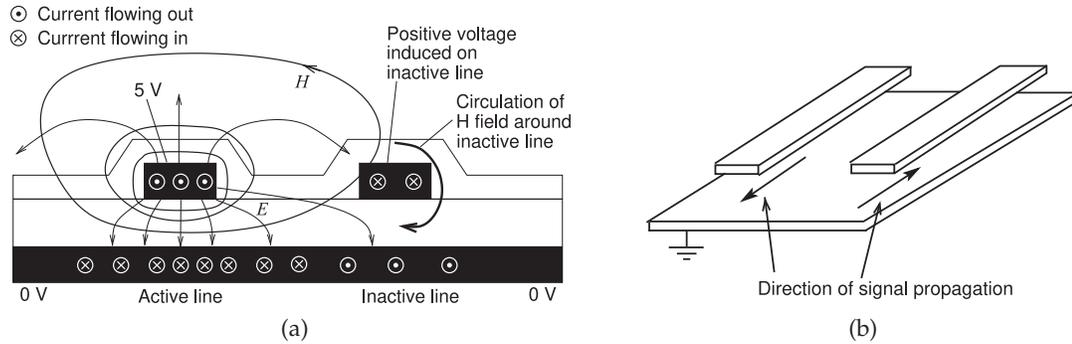
**Figure 6-1:** Edge-coupled microstrip lines with the left line driven with the forward-traveling field coming out of the page: (a) cross section of microstrip lines as found on a printed circuit board showing a conformal top passivation or solder resist layer; and (b) in perspective showing the direction of propagation of the driven line (left) and the direction of propagation of the main coupled signal on the victim line (right).
