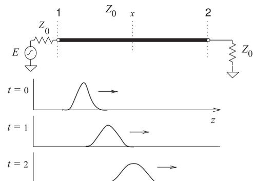
**Figure 5-2:** Dispersion of a pulse along a line.
