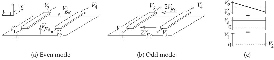
**Figure 6-3:** Definitions of total voltages and even- and odd-mode voltage phasors on a pair of coupled microstrip lines: (a) even-mode voltage definition; (b) odd-mode voltage definition; (c) depiction of how even- and odd-mode voltages combine to yield the total voltages on individual lines. *F* indicates front and *B* indicates back.
