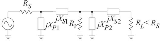
**Figure 10-28:** Matching network with two L networks.
