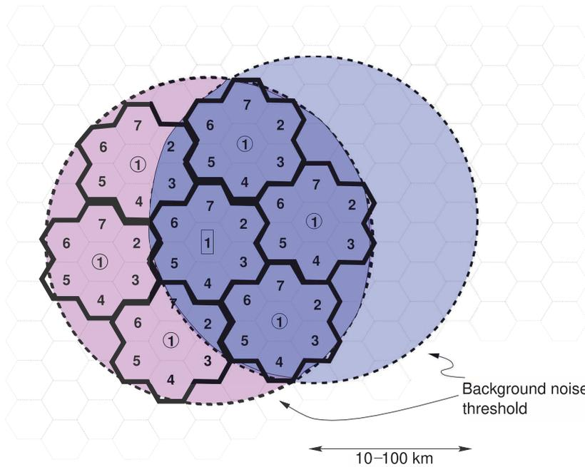
**Figure 1-9:** Interference in a cellular radio system.
