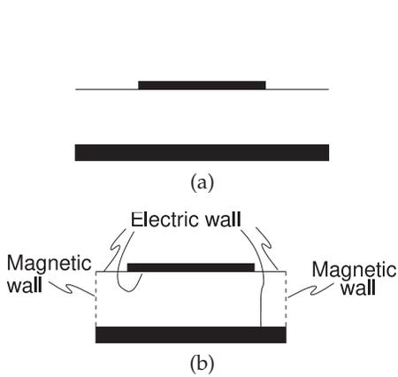
**Figure 5-10:** Approximation of a microstrip line as a waveguide: (a) cross section of microstrip; and (b) **microstrip waveguide model** having effective width  $w + 0.4h$  with magnetic and electric walls.
