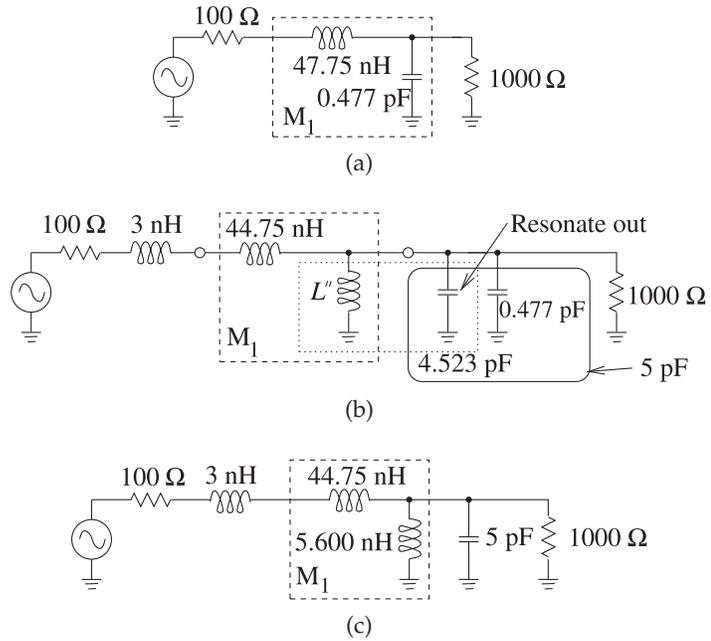
**Figure 10-17:** Evolution of the matching network in Example 10.6: (a) matching network design considering only the source and load resistors; (b) matching network with the reactive parts of the source and load impedances included; and (c) final design.
