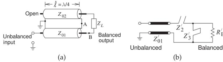
**Figure 9-17:** Marchand balun: (a) coaxial form of the Marchand balun; and (b) its equivalent circuit.
