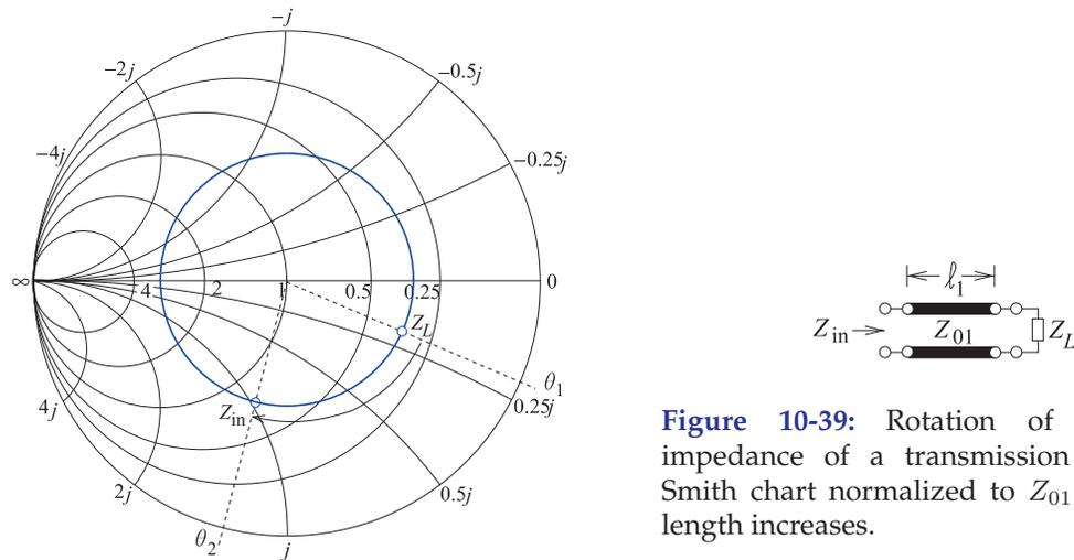
Figure 10-39: Rotation of the input impedance of a transmission line on a Smith chart normalized to  $Z_{01}$  as the line length increases.
