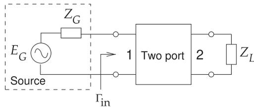
**Figure 7-5:** Terminated two-port used to define return loss.
