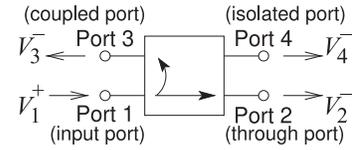
Figure 7-6: Schematic of a directional coupler.
