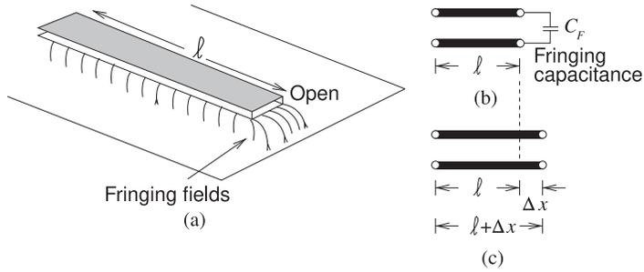
**Figure 9-11:** An open on a microstrip transmission line: (a) microstrip line showing fringing fields at the open; (b) fringing capacitance model of the open; and (c) an extended line model of the open with  $\Delta x$  being the extra transmission line length that captures the open.
