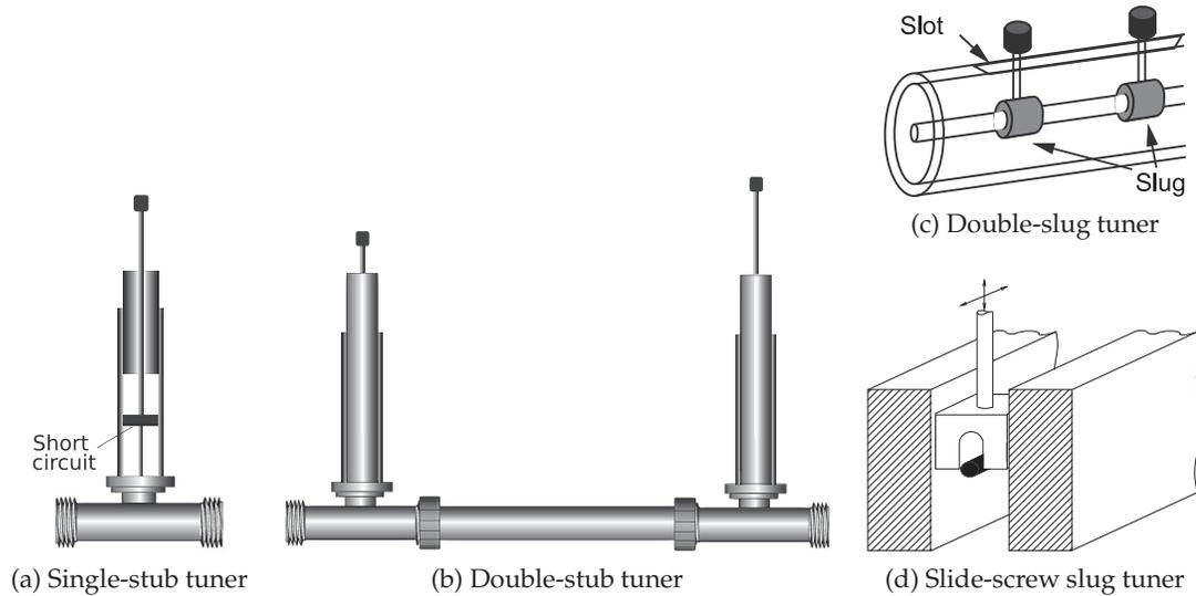
Figure 10-38: Laboratory tuners.
