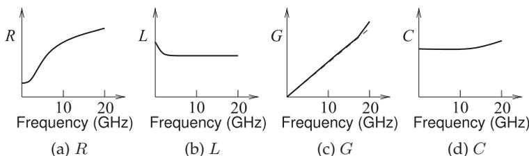
**Figure 5-1:** Frequency dependence of transmission line parameters.
