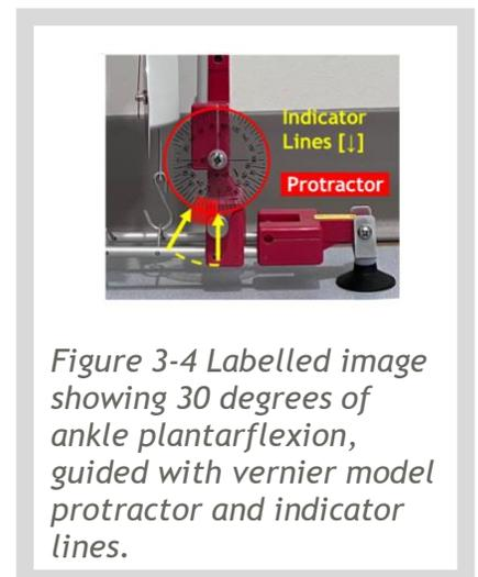
*Figure 3-4 Labelled image showing 30 degrees of ankle plantarflexion, guided with vernier model protractor and indicator lines.*
