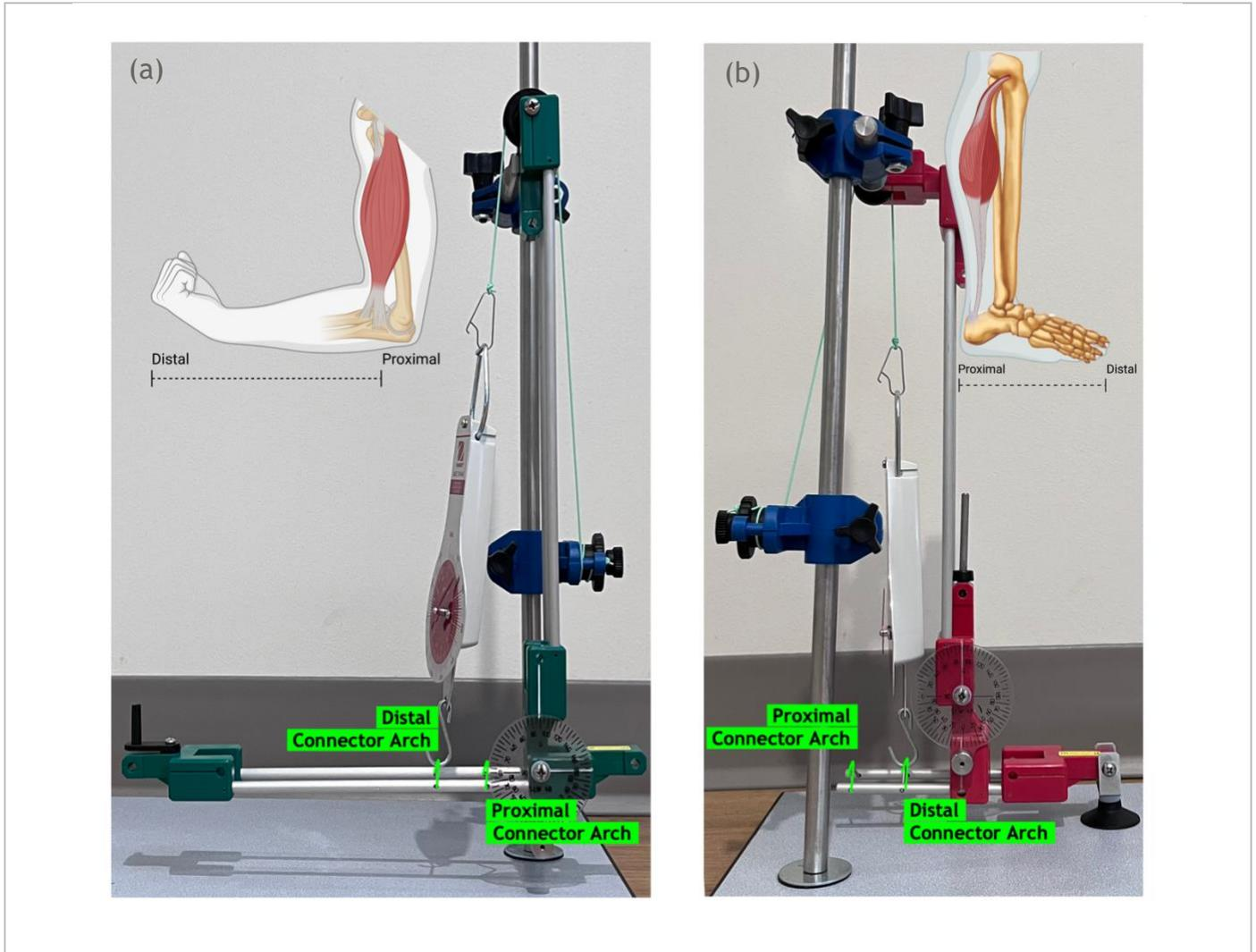
Figure 3-2 Labeled images illustrating the proximal and distal connector arches for the upper (a) and lower limb (b) Vernier musculoskeletal models. Some image components were created with BioRender.com
