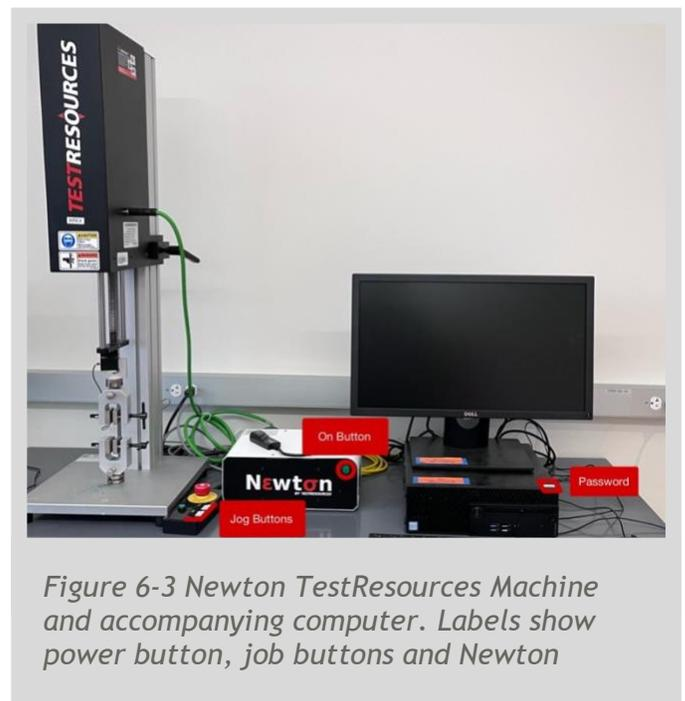
Figure 6-3 Newton TestResources Machine and accompanying computer. Labels show power button, job buttons and Newton
