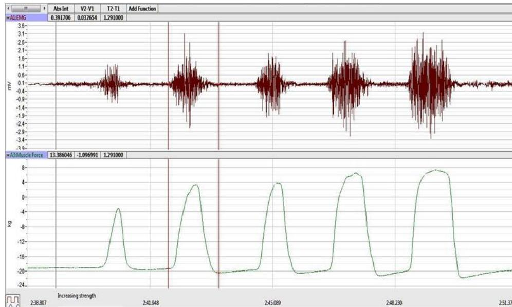
Figure 5-3 The EMG and muscle force recordings displayed in the Analysis window. The cursors are placed on the margins of the 2<sup>nd</sup> muscle contraction and the absolute integral function is used to measure the area under the EMG spikes and the area under the force recording.
