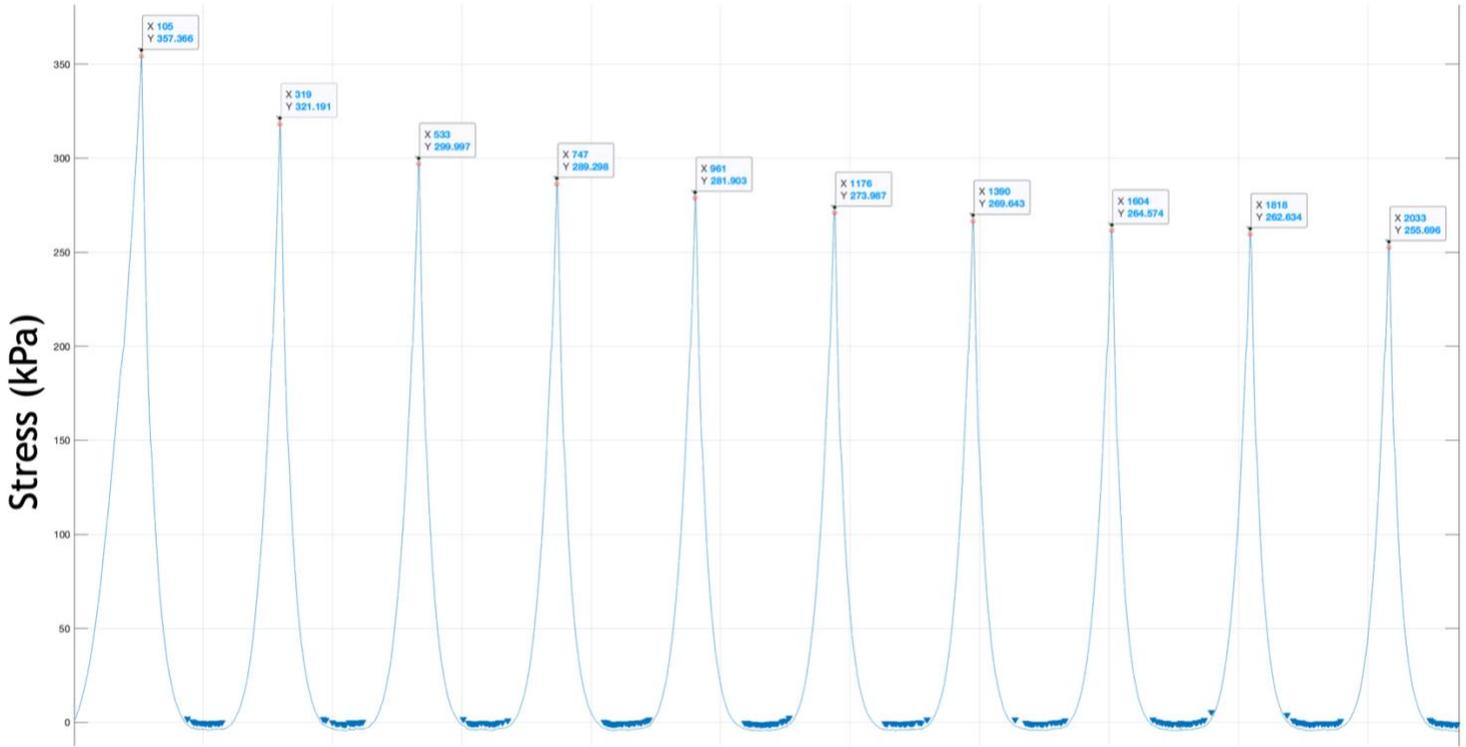
Figure 7-5 Stress (kPa) Vs Time (sec) plot with the peaks of each hysteresis cycle highlighted.
