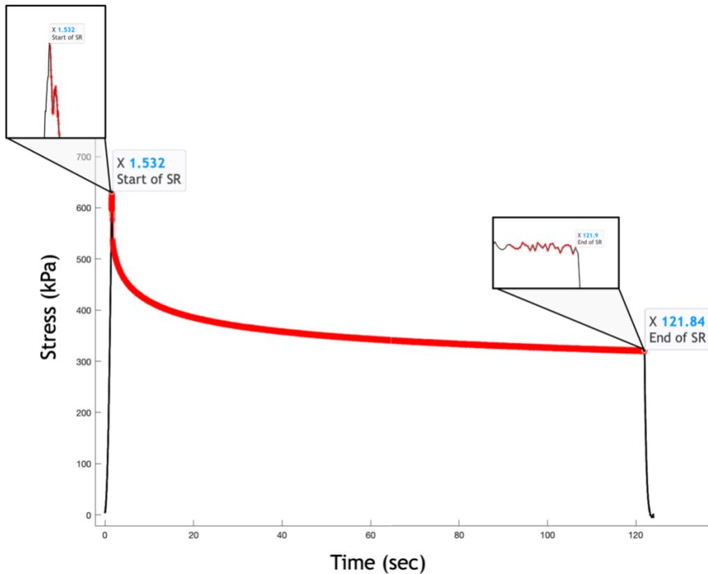
Figure 7-3 Stress (kPa) Vs Time (sec) plot with the Start and End of the Stress Relaxation (SR) period highlighted.
