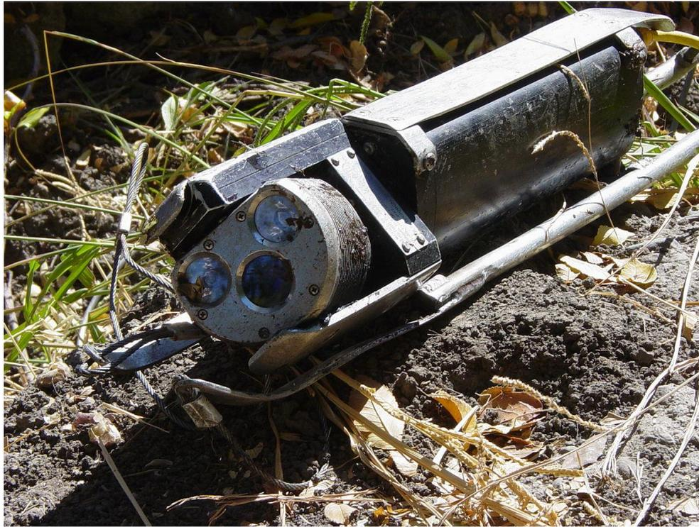
*Figure 3.6 - A Video 'Pig' for Pipe Inspection*
