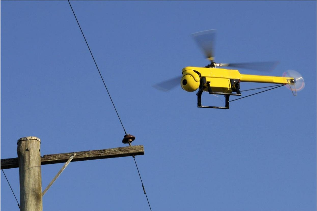
Figure 3.7 - An Unmanned Aerial Vehicle or 'Drone' used for Visual Inspection of Power Lines
