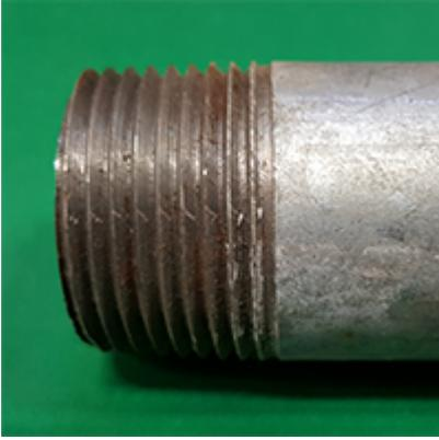
American standard thread used in plumbing and piping systems. It may also be referred to as MPT or MNPT for male external threads and FPT or FNPT for female internal threads. A thread sealant of some type should always be used to obtain a leak free seal (except for NPTF).
