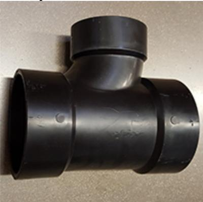
Sanitary Tees should be used when connecting a horizontal run, such as a waste arm to a vent stack or vertical riser. They are only used to go from the horizontal to vertical plane.
