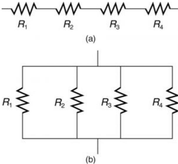
Image shows (a) A series connection of resistors. (b) A parallel connection of resistors.
