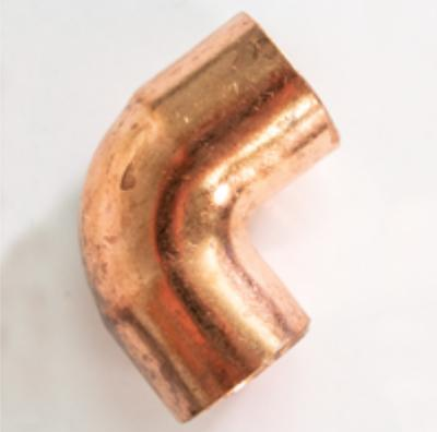
Elbows normally create a 90° or 45° change in direction of a piping system. 22-1/2° fittings are also available for some piping systems. Depending on the material, elbows come in female slip-to-female slip, female slip-to-female slip, slip-to-female thread, slip-to-male thread. PVC and Copper female slip-to-male slip elbows are referred to as street elbows and they are used for close turns and swivel to fit connections.
