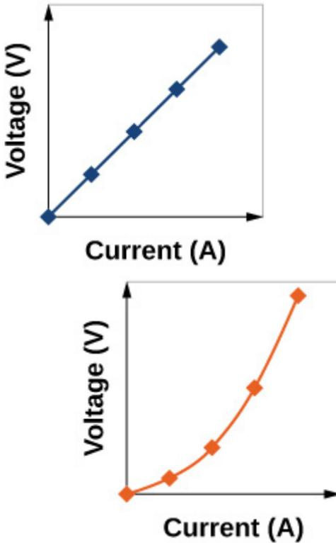
Figure #. The relationship between voltage and current for ohmic and non-ohmic materials are shown.
