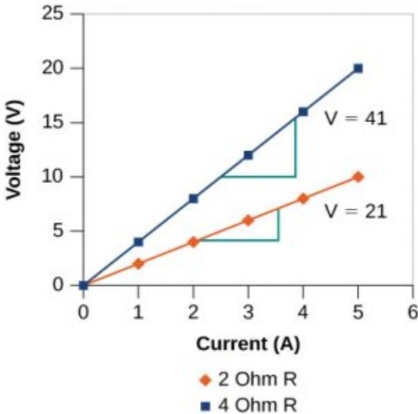
The figure illustrates the relationship between current and voltage for two different resistors. The slope of the graph represents the resistance value, which is  $2\Omega$  and  $4\Omega$  for the two lines shown.
