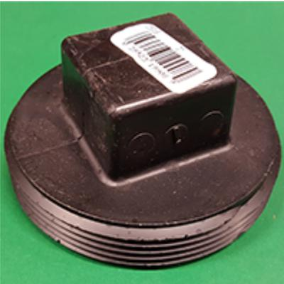
Clean-Outs are threaded plugged access points in a DWV system used for clearing clogged lines with augers and inspecting DWV systems with cameras. Plumbing system codes dictate how many clean-outs should be in a waste system by the length of run and the amount of turns in the system.
