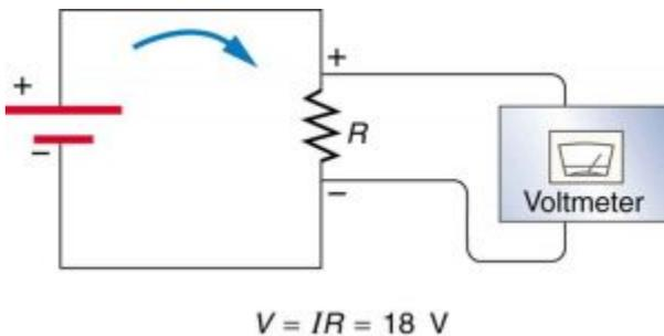
*The voltage drop across a resistor in a simple circuit equals the voltage output of the battery.*
