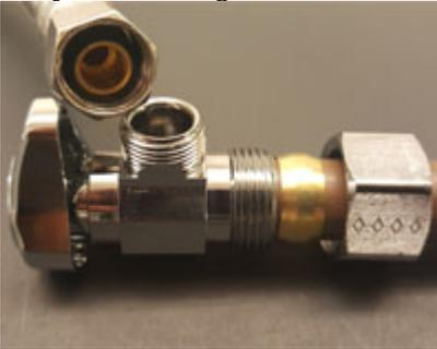
Compression fittings are sometimes used to install plumbing system components and make quick repairs on smooth outside diameter pipes like PVC and copper. Compression fittings require that a soft brass metal sleeve in copper applications, and Teflon or pliable washer in PVC applications, is compressed around the piping material by an adjustment nut to seal the fitting.
