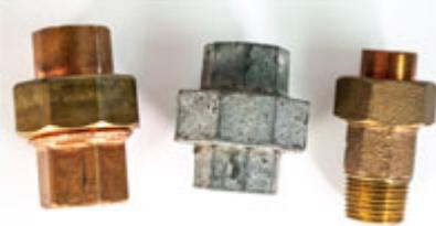
Unions facilitate the removal and repair of system components and consist of one fitting having a swivel nut which attaches to the other fitting which has a male threaded adapter with a flange or compression type seal.
